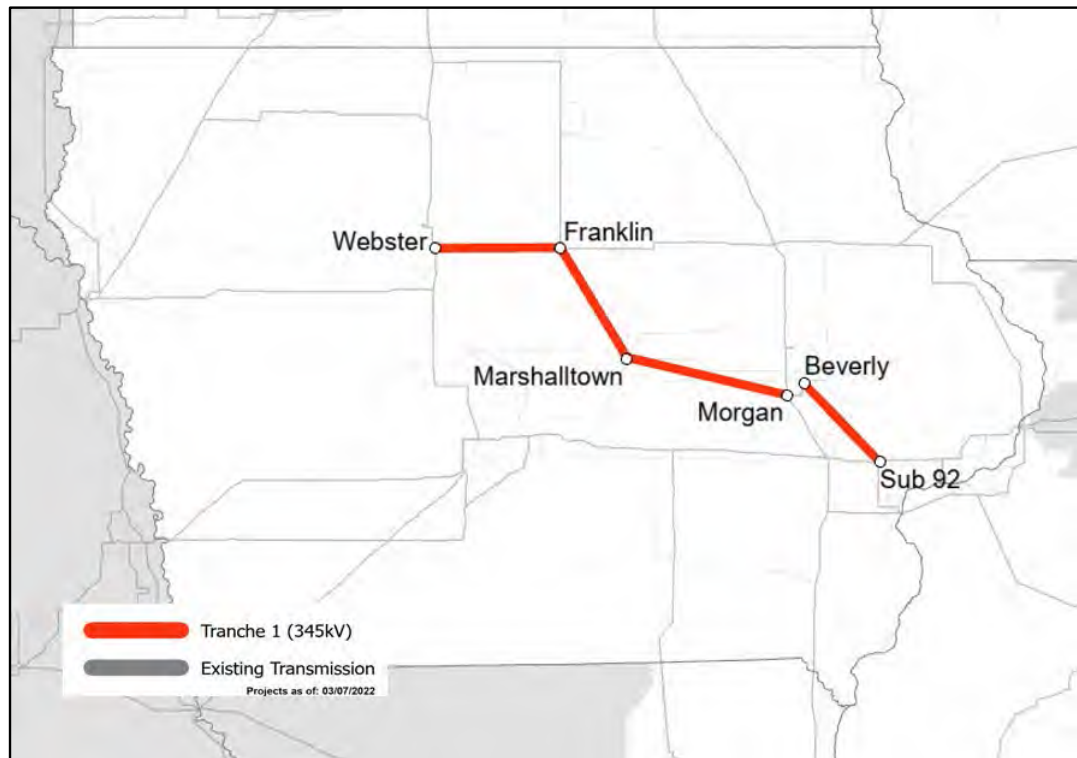
Figure 6-10: Central Iowa Final Solution
