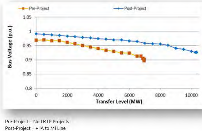
Figure 6-14: Improved voltage profiles in Indiana and Increased transfer levels with the Iowa to Michigan Projects
