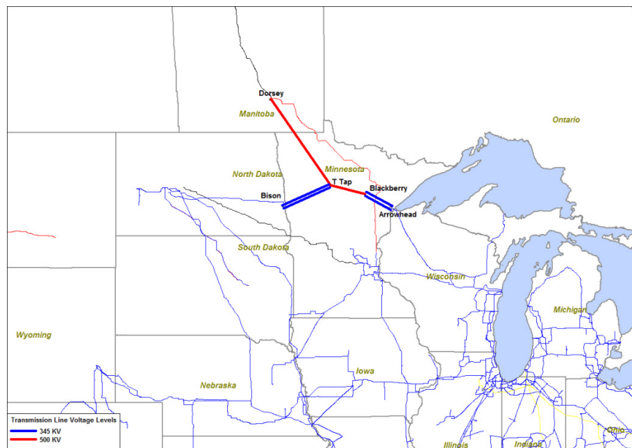
Figure 1-5: Manitoba – Fargo and Duluth “T” 500 kV Tie-Line
