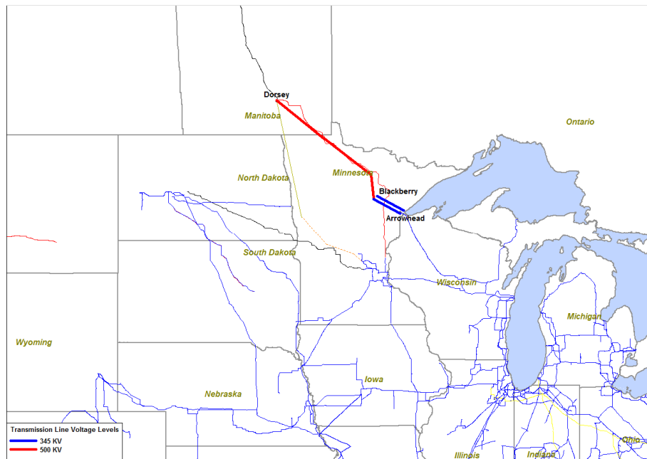
Figure 1-3: Manitoba - Duluth 500 kV Tie-Line
