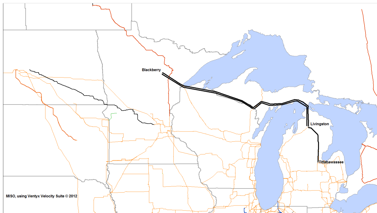
Figure 6-34: Blackberry – Livingston/Tittabawassee 500 kV HVDC
