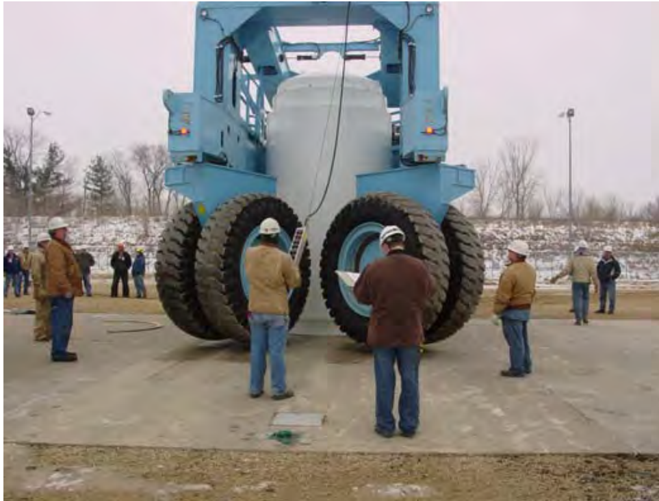
Figure 6. TN-40 Cask Placed on ISFSI Pad
