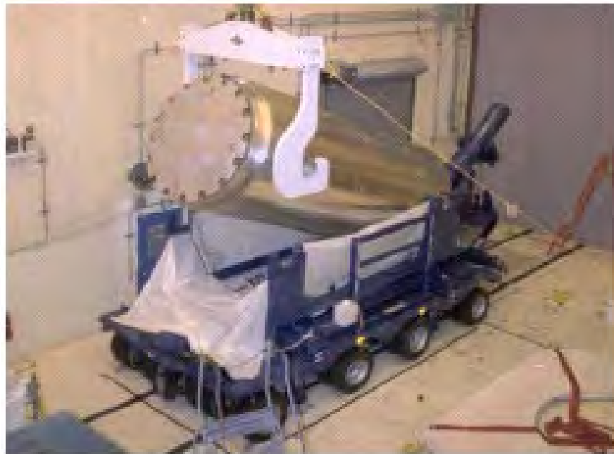
Figure C-8: Lowering Cask onto Trailer
