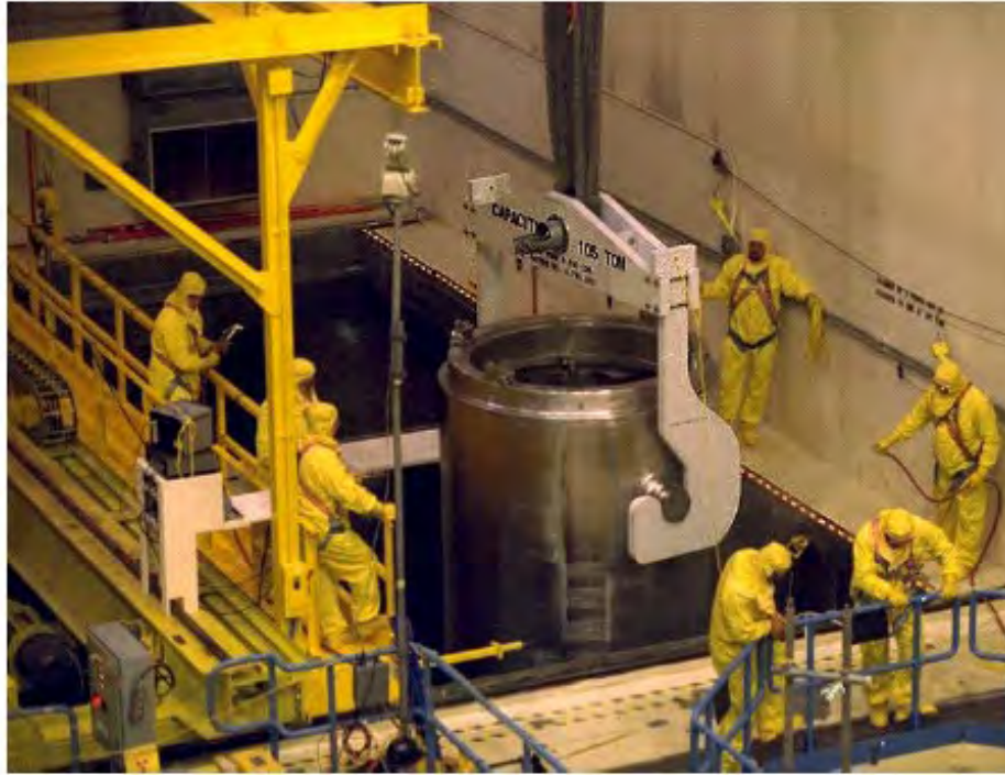
Figure C-7: Lowering Transfer Cask to Decontamination Area
