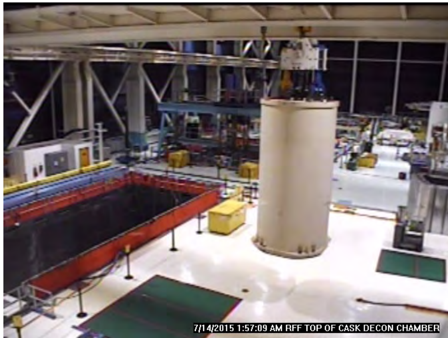
Figure C-10: Transfer Cask and Canister Movement to the Spent Fuel Pool
