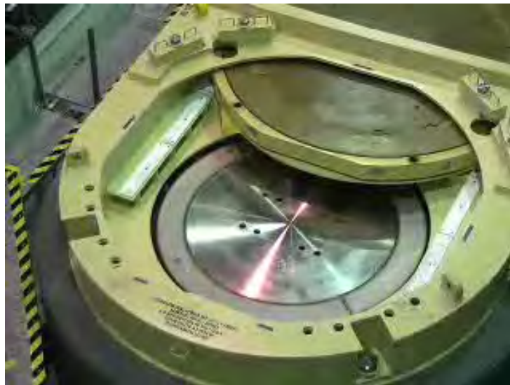
Figure C-18: Canister Lowered into Overpack; Lift Cleats and Downloader Slings Removed
