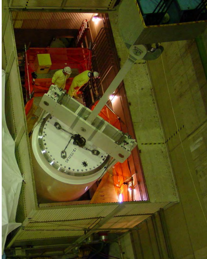
Figure C-3: Cask in Decontamination Area
