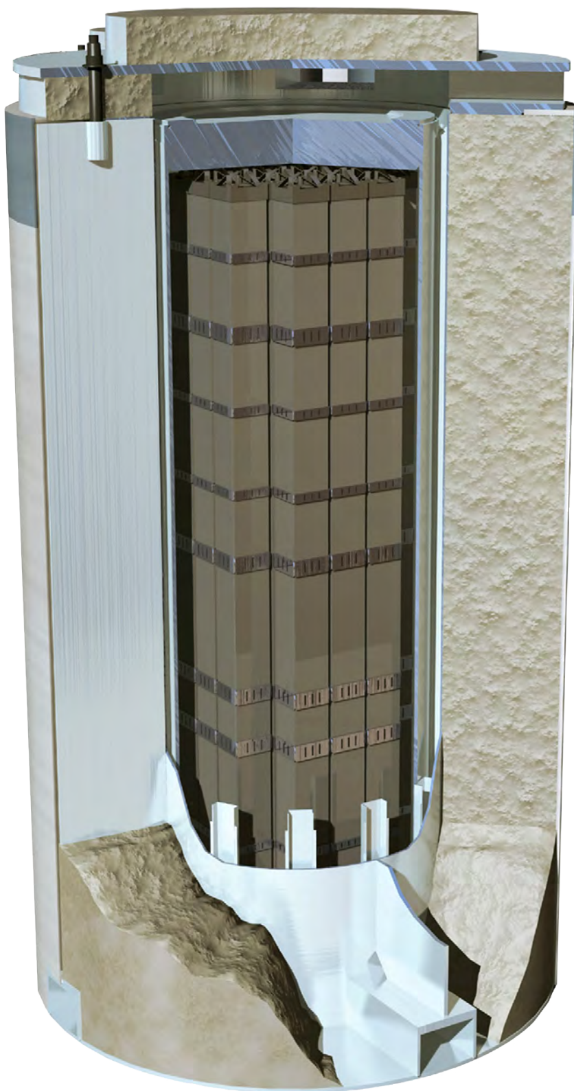
Cutaway of spent fuel storage cask shows spent fuel assemblies surrounded by steel and thick concrete shielding.
