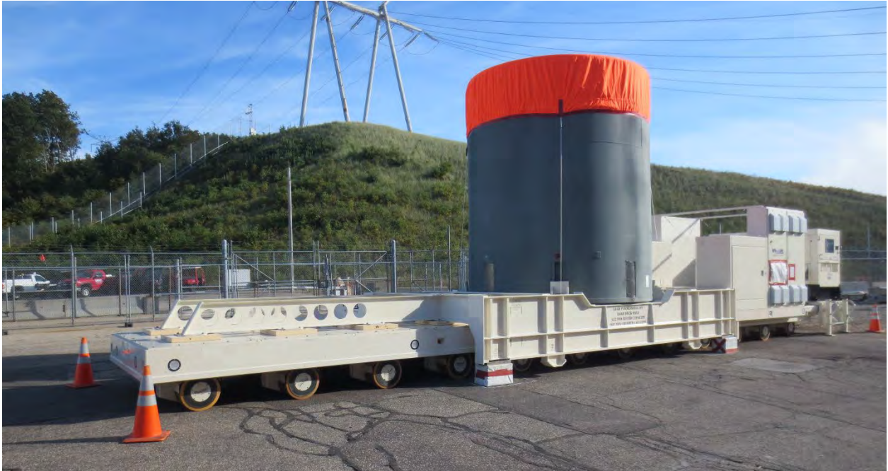
Figure C-14: Overpack on Crawler
