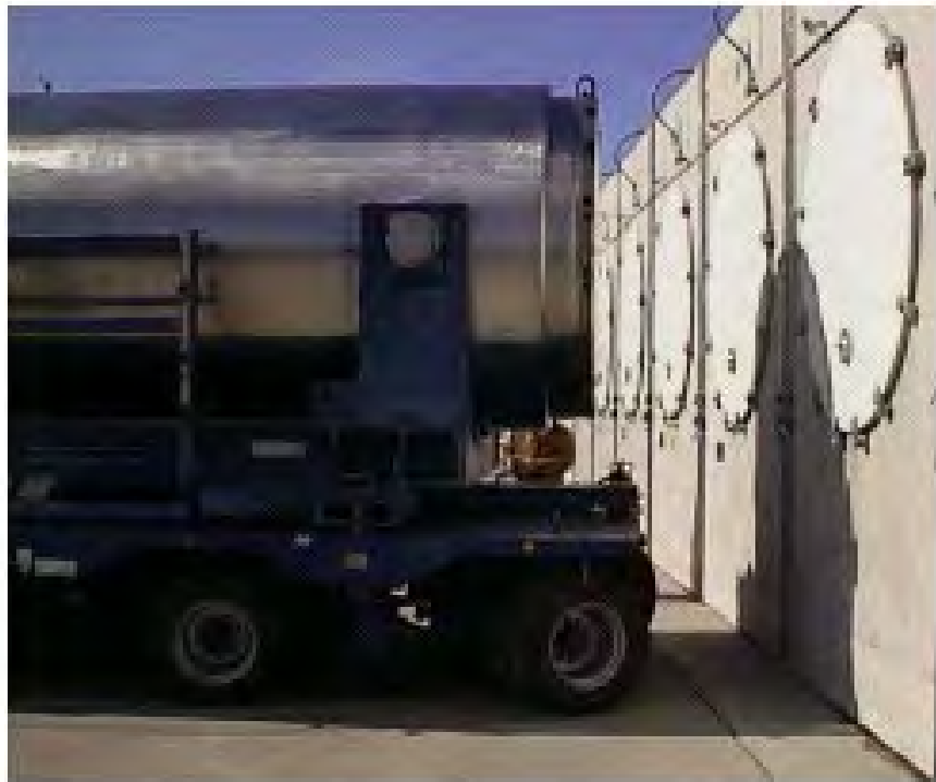
Figure C-9: Alignment of Transfer Cask with Storage Module
