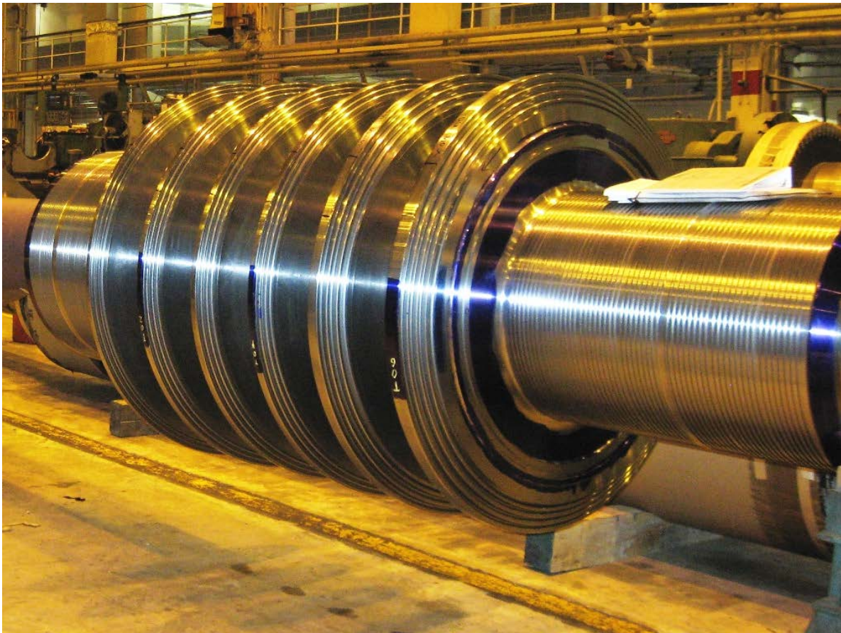
High-Pressure Turbine Rotor
