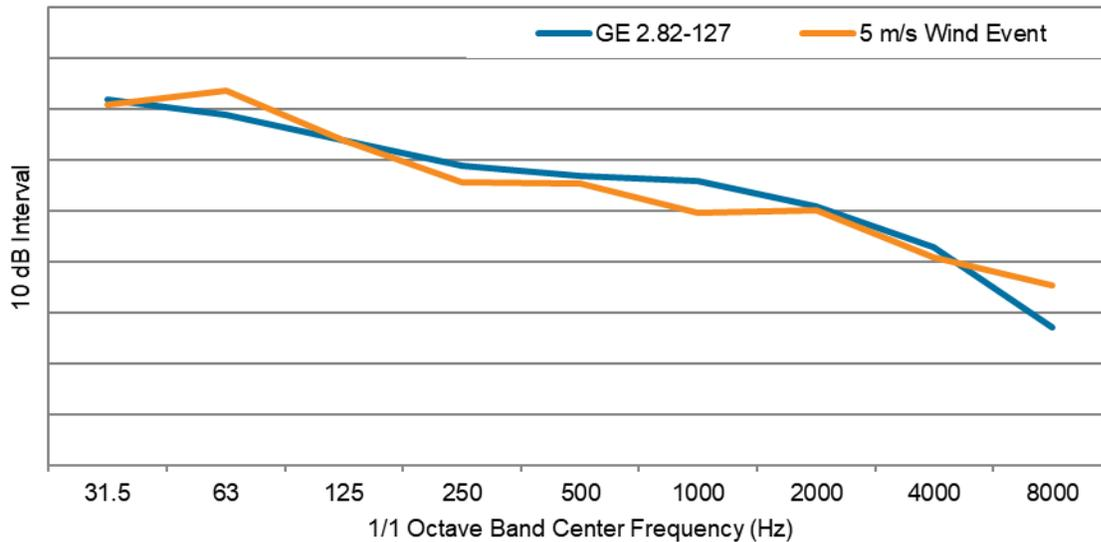
FIGURE 4: COMPARISON OF NORMALIZED FREQUENCY SPECTRA FROM THE WIND AND THE GE 2.82-127<sup>6</sup>
