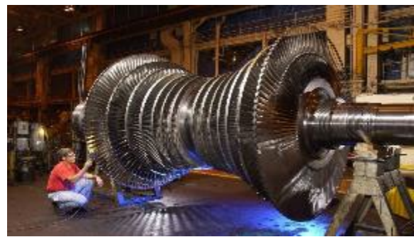
Figure 6 - LP Turbine Rotor
