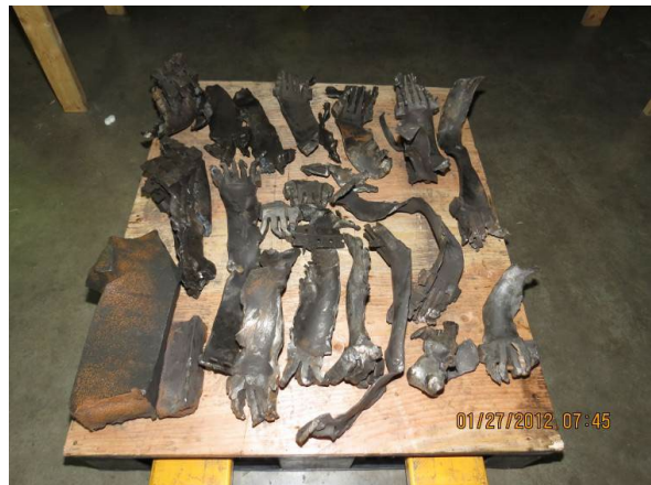
Figure 9 - Damaged LP Turbine Blades
