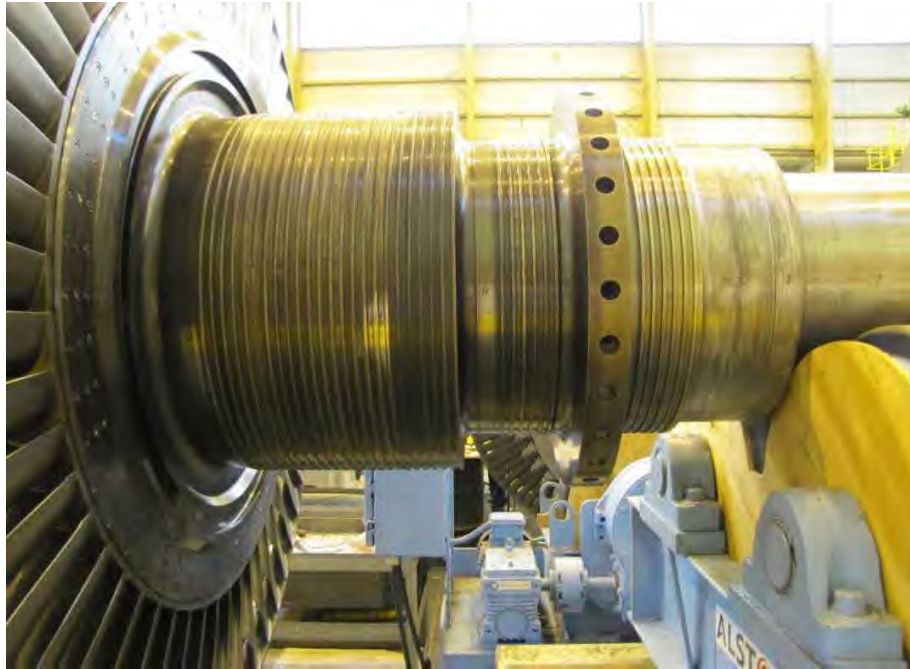
Fig. 34. Close-up photograph of intermediate pressure turbine rotor shown in Fig. 31 showing rub damage seal surfaces.
