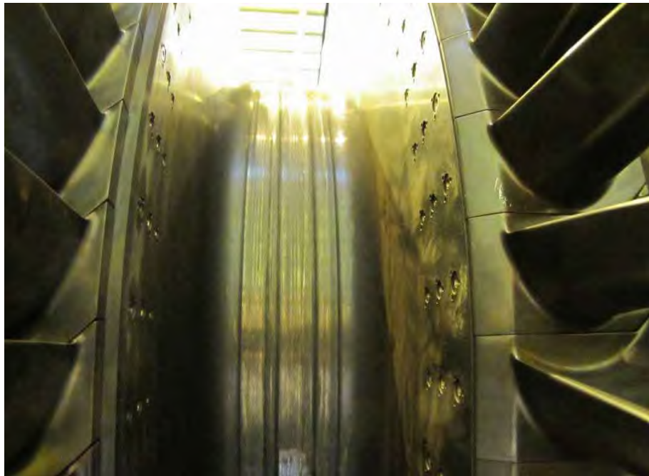
Fig. 37. Close-up photograph of intermediate pressure turbine rotor showing light rub damage on interstage seal surfaces.
