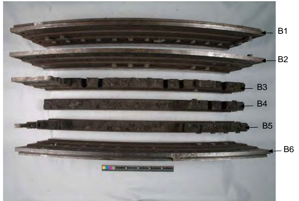
Fig 136. SID 14875 subsegment "B" after circumferential sectioning.
