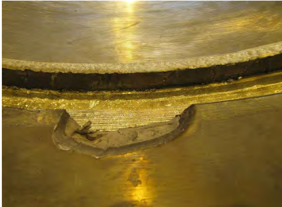
Fig. 22. Close-up of high pressure turbine inner casing shown in Fig. 20 showing fractured section of the inlet gland seal fit.
