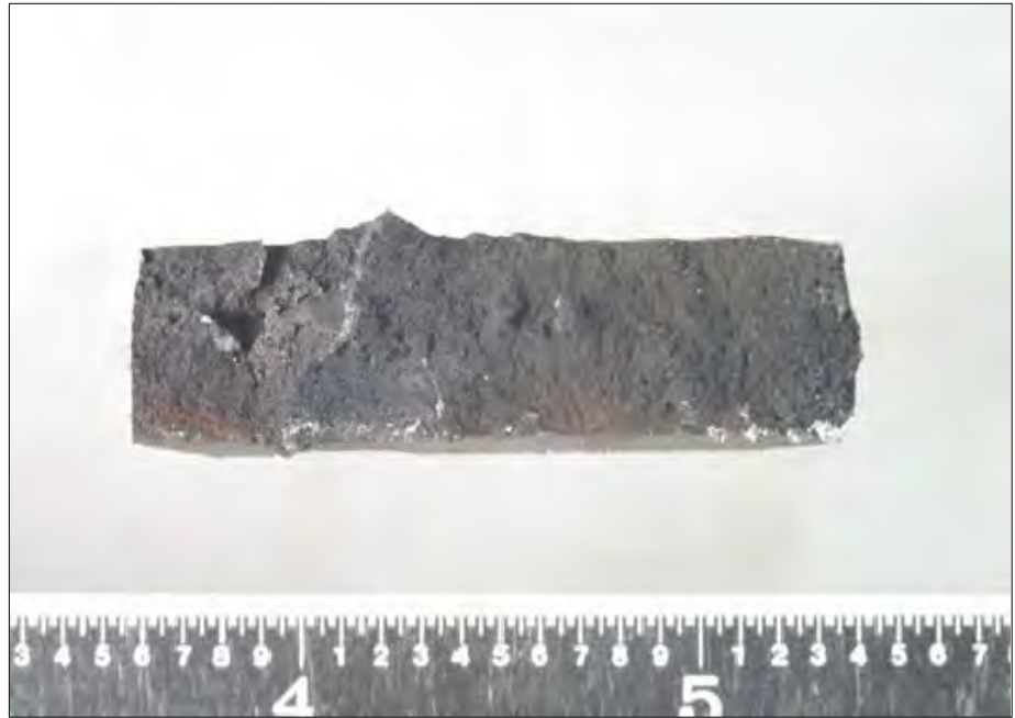
Fig 166. Close-up of surface of fracture through crack No. 1 from SID 14875 subsegment "C4".
