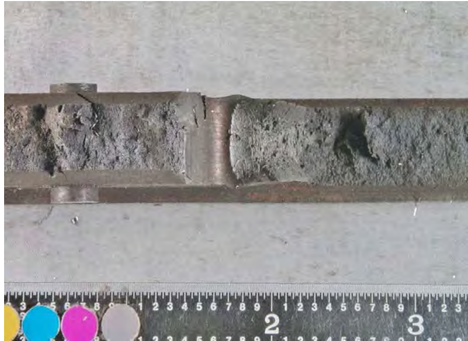
Fig. 134. Close-up photograph of SID 14874 subsegment "A4" fracture surface shown in Fig. 132.
