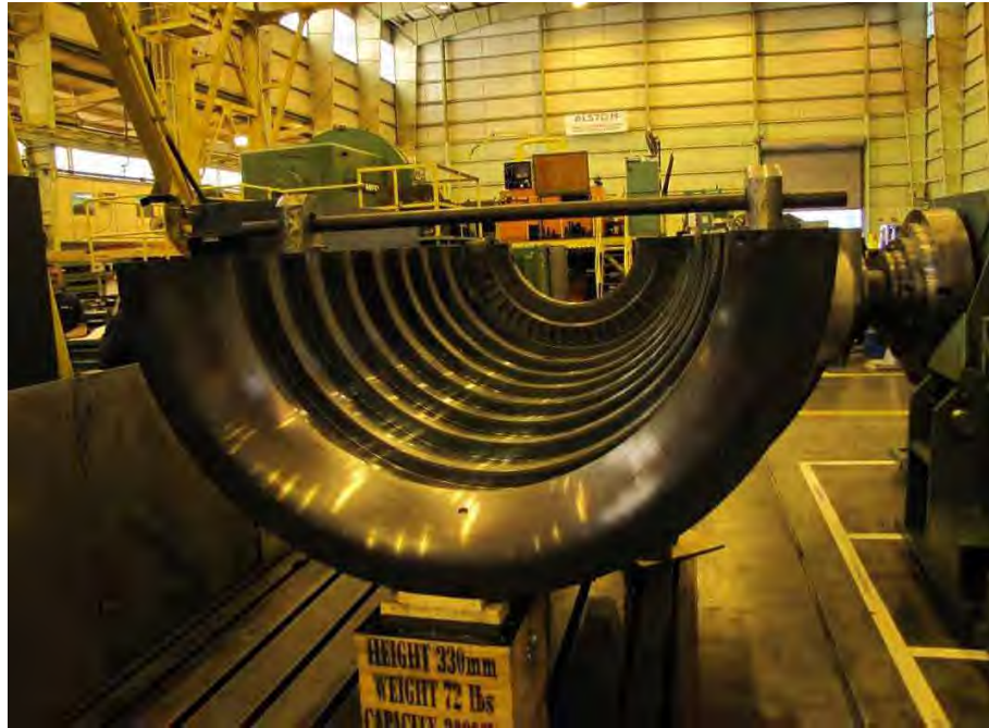
Fig. 20. Photograph of high pressure turbine inner casing at the Alstom Power, Inc. repair facility in Richmond, VA.
