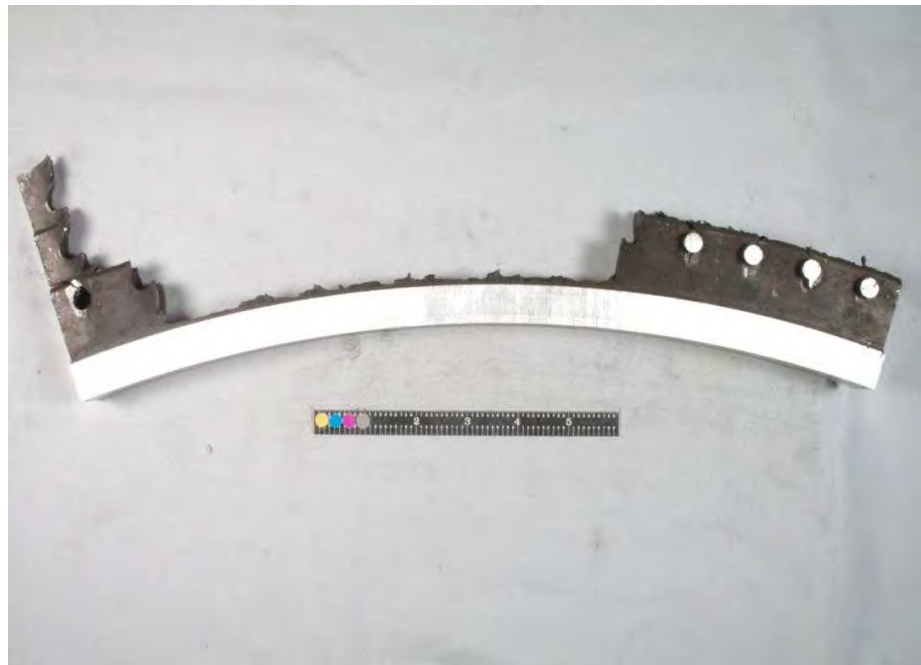
Fig. 139. SID 14875 subsegment "B5" finger pinned blade attachment, outlet side.
