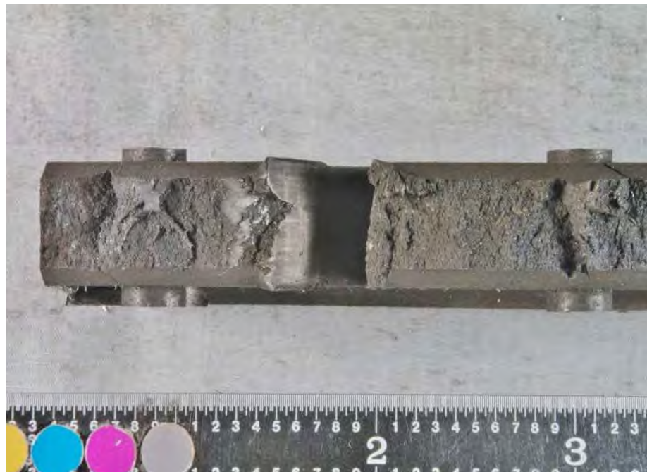
Fig 133. Close-up of SID 14874 subsegment "A4" fracture surface shown in Fig. 132.
