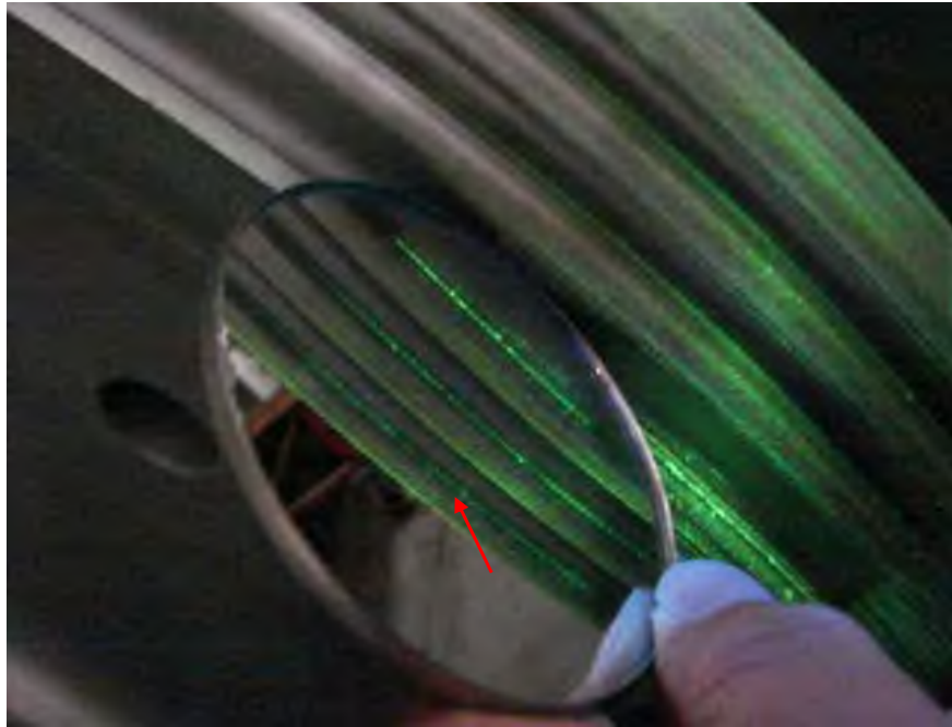
Fig. 94. Close-up blacklight photograph of low pressure turbine "A" generator end L-3 stage disk on exit side of the blade dovetail showing indication (arrow).
