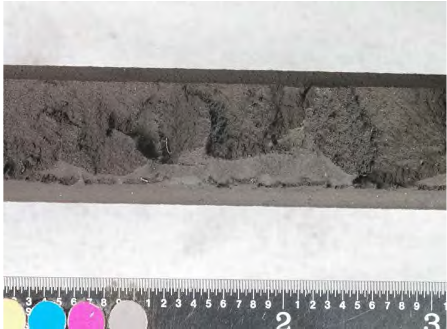
Fig. 152. Close-up of SID 14875 subsegment "B5" fracture surface shown in Fig. 150.
