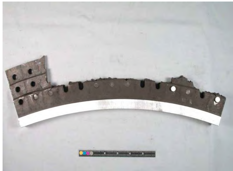
Fig. 137. SID 14875 subsegment "B3" finger pinned blade attachment, outlet side.
