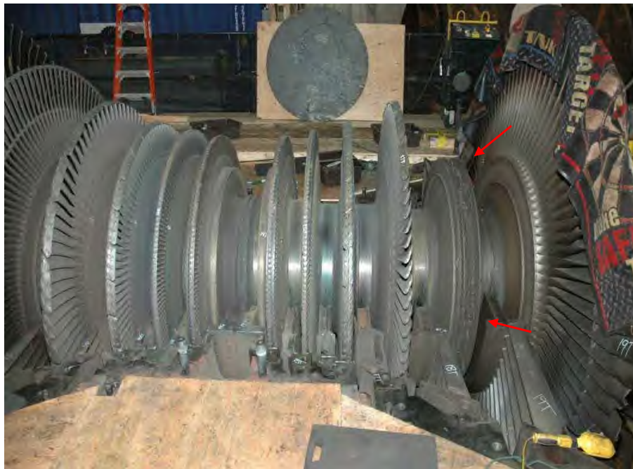
Fig. 55. Photograph of low pressure turbine rotor "B" in casing showing section of disk rim which fractured (arrows) through finger root attachments.
