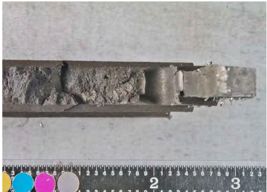
Fig. 131. Close-up of SID 14874 subsegment "A3" fracture surface shown in Fig. 128.
