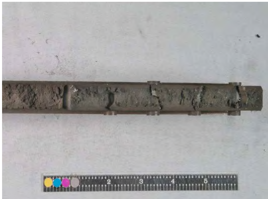
Fig. 151. Close-up of SID 14875 subsegment "B5" fracture surface.
