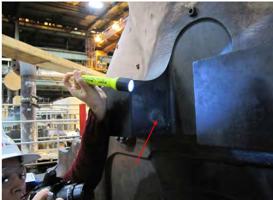
Fig. 29. Photograph of melted area (arrow) on alignment lug of outer casing from intermediate pressure turbine.
