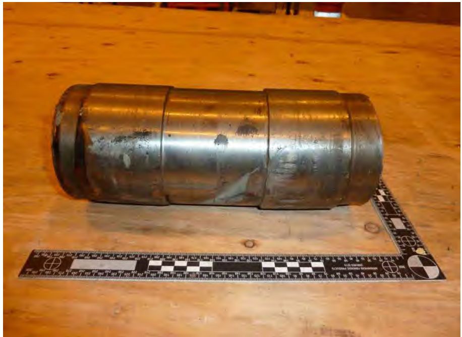
Fig. 109. Photograph of third fracture through exciter shaft at collector end.
