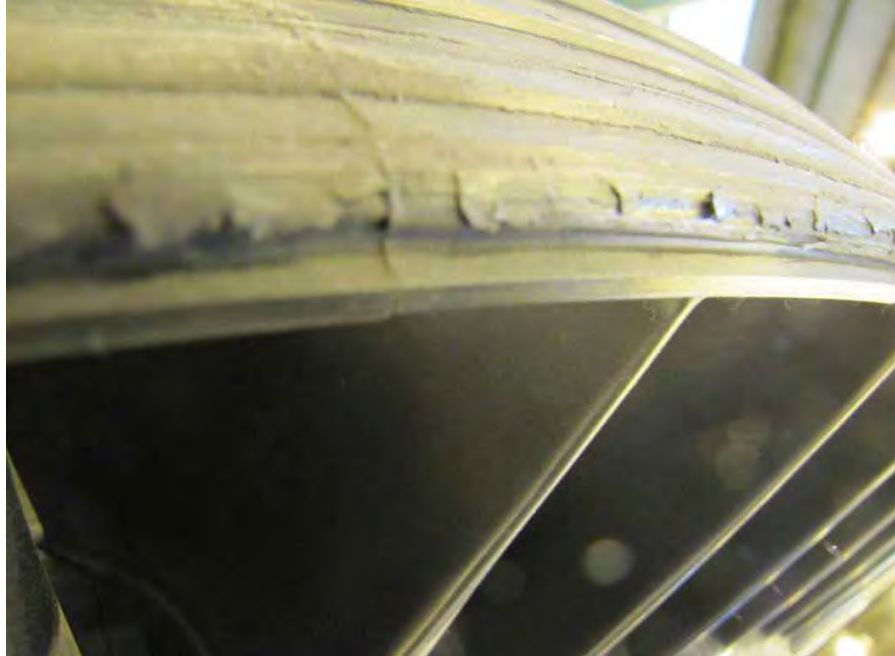
Fig. 14. Close-up photograph of high pressure turbine rotor shown in Fig. 13 showing moderate/heavy rub damage on blade integral shrouds.
