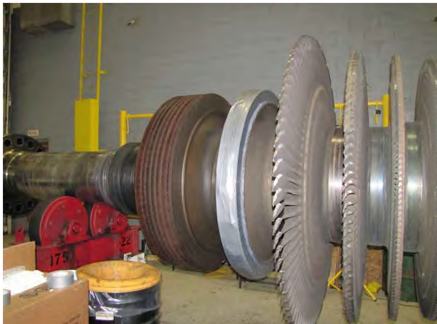
Fig. 84 Photograph of low pressure turbine "B" rotor at the GE Repair Facility in Chicago, IL., showing protective taping of fractured L-1 stage disk rim.
