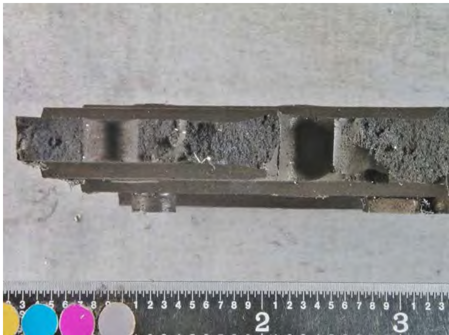
Fig. 129 Close-up of SID 14874 subsegment "A3" fracture surface shown in Fig. 128.
