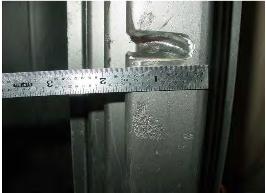
Fig. 102. Close-up photograph of low pressure turbine "A" generator end L-2 stage disk rim showing excavation of indication at 155° location.
