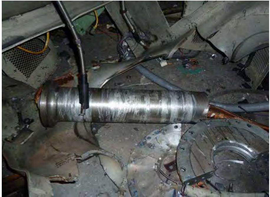
Fig. 108. Photograph of second fracture through exciter shaft.
