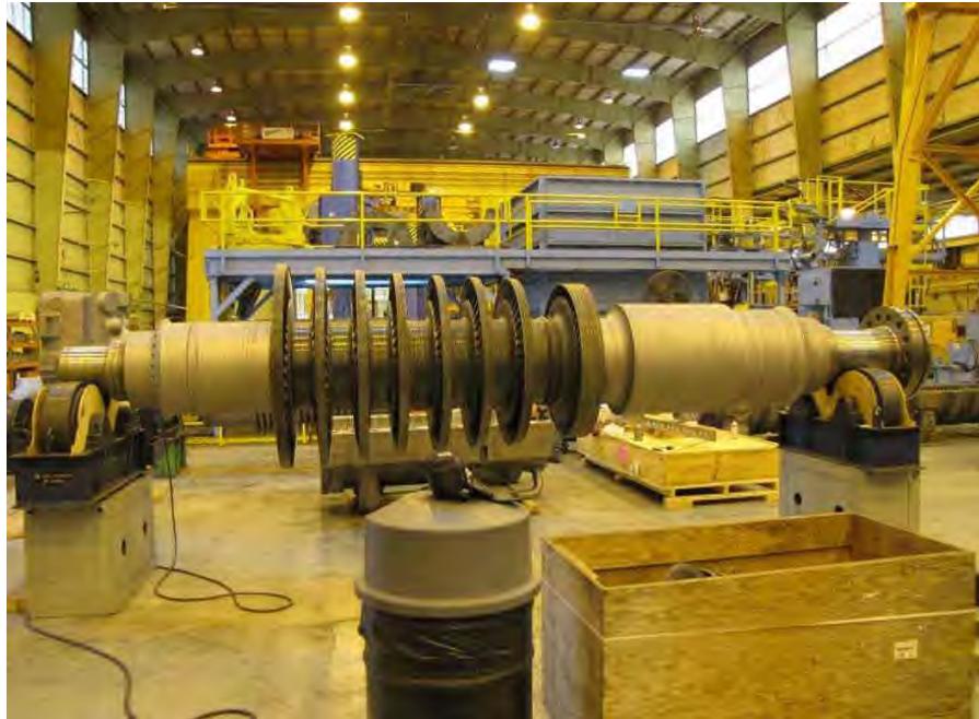
Fig. 12. Photograph of high pressure turbine rotor from Sherco Unit 3 at the Alstom Power, Inc., repair facility in Richmond, VA.
