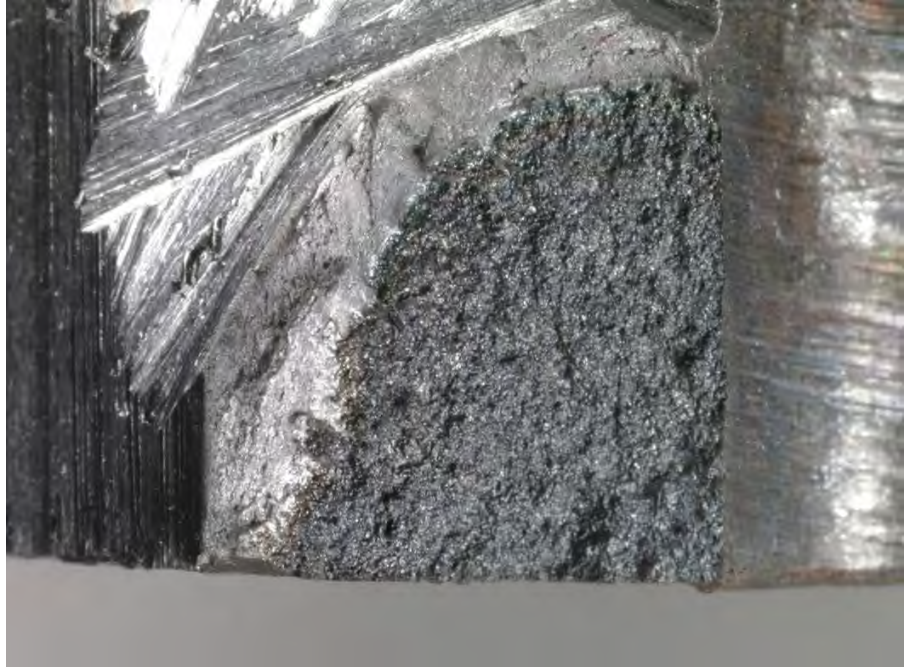
Fig 172. Close-up of surface of fracture through crack No. 3 from SID 14875 subsegment "C4" shown in Fig. 171.
