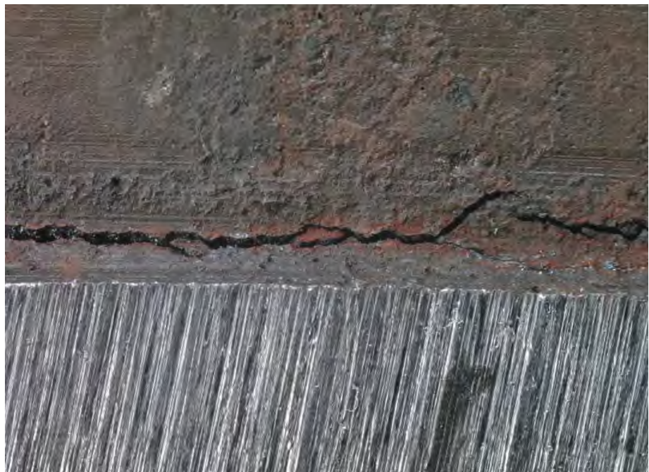
Fig 159. Close-up of SID 14875 subsegment "C4" crack No. 1 shown in Fig. 158, viewed from inlet side.
