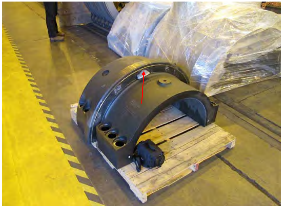
Fig. 23. Photograph of high pressure turbine inlet gland casing showing fractured casing material (arrow) attached to outer surface.
