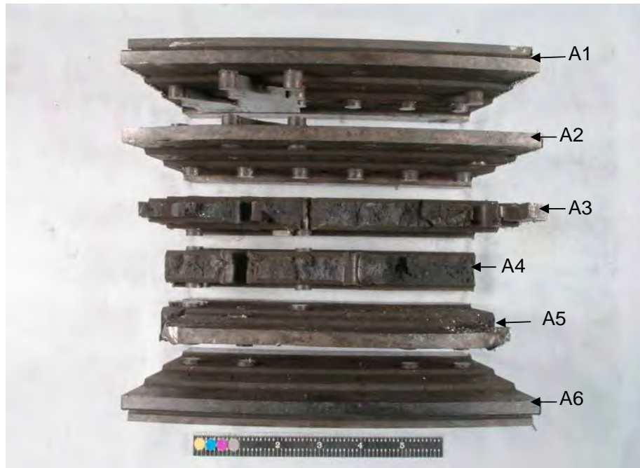
Fig. 125. SID 14874 subsegment "A" after circumferential sectioning.
