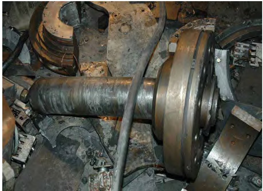
Fig. 107. Photograph of portion of fractured exciter shaft.
