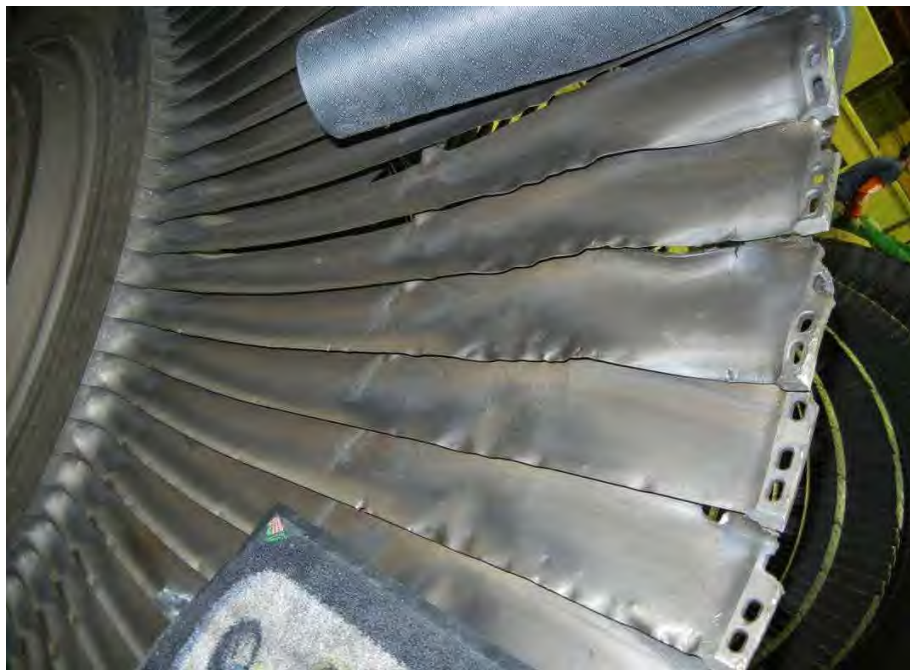
Fig. 65. Photograph of turbine end last stage blades from low pressure turbine "B".
