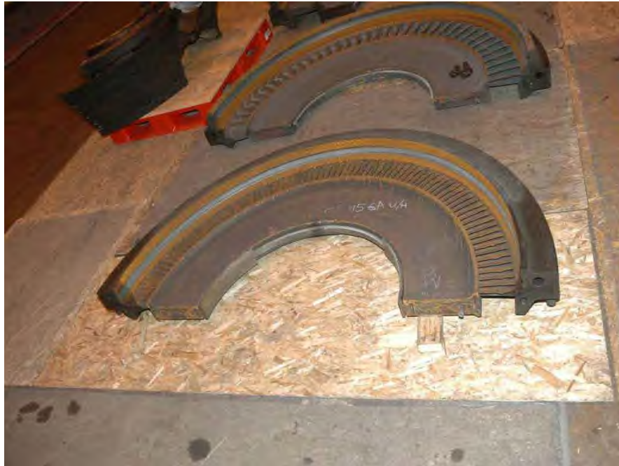
Fig. 54. Close-up of generator end L-4 upper half diaphragm from low pressure turbine "A" showing rub damage to vanes.
