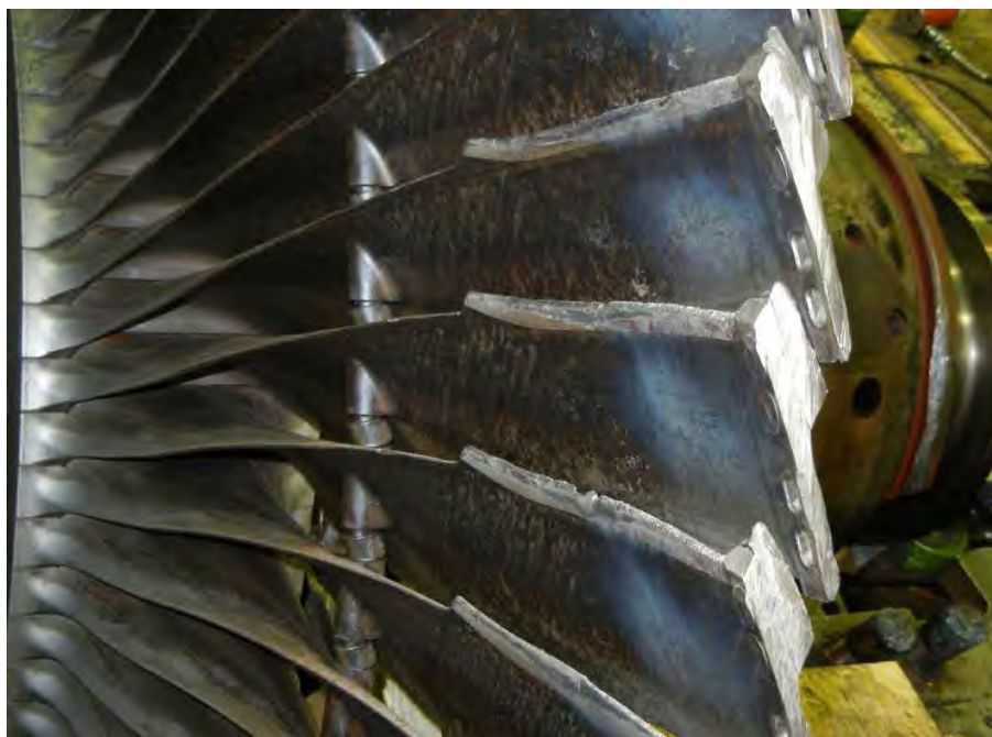
Fig. 73. Photograph of low pressure turbine "B" generator end last stage blades.
