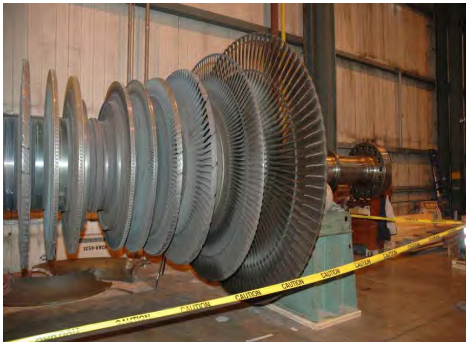
Fig. 45. Photograph of low pressure turbine rotor "A" shown in Fig. 44.
