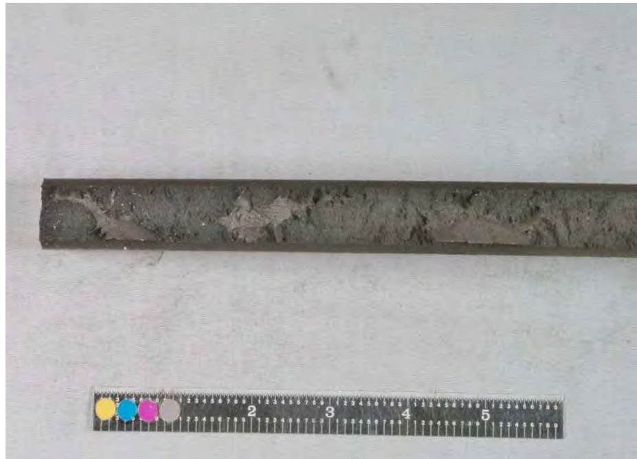
Fig 146. Close-up of SID 14875 subsegment "B4" fracture surface.
