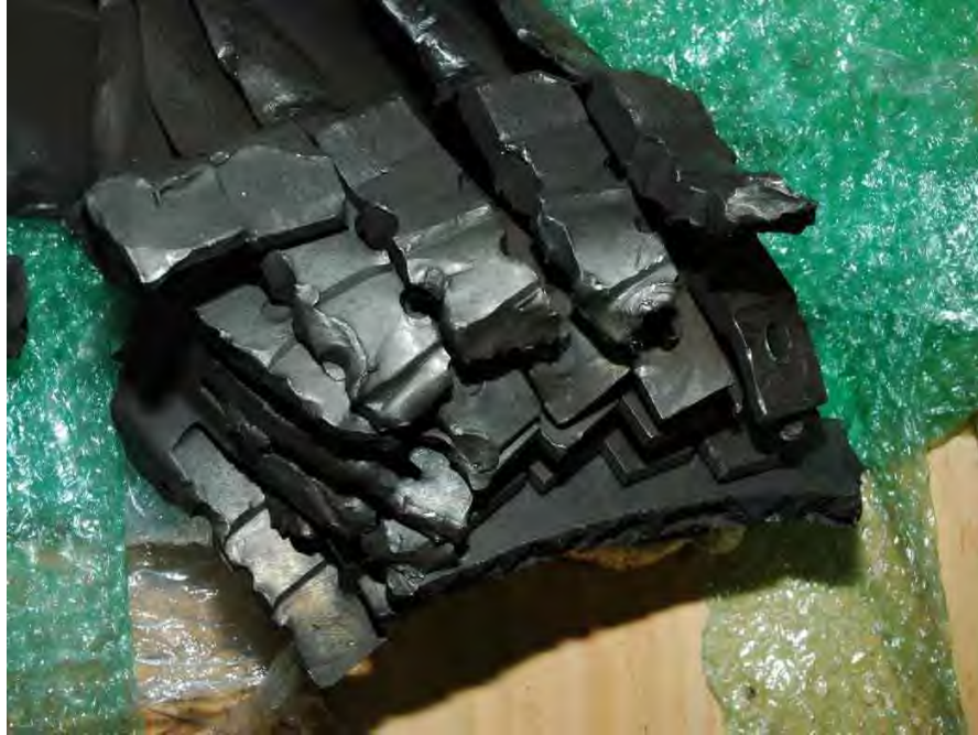
Fig. 62. Photograph of liberated turbine end L-1 blades from the low pressure turbine "B" rotor which section of fractured inner finger root attachment from disk rim.
