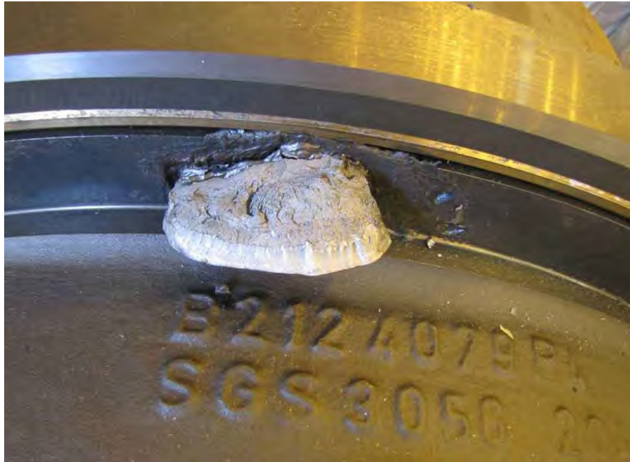
Fig. 24. Close-up photograph of fractured casing material shown in Fig. 23.
