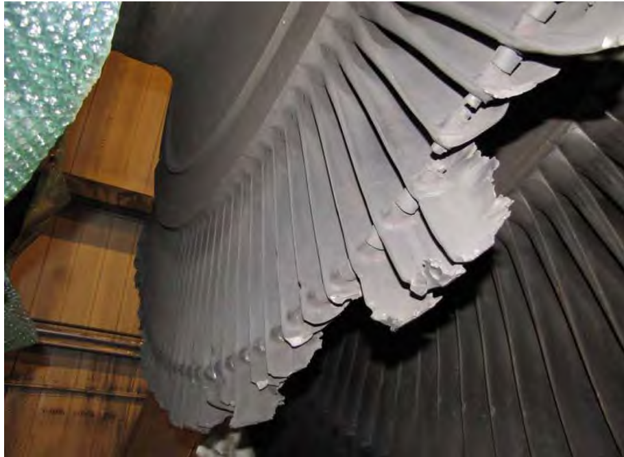
Fig. 60. Photograph of turbine end L-1 stage blades from low pressure turbine "B" rotor showing extent of damage.
