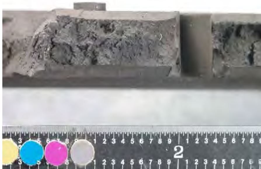
Fig. 149. Close-up of SID 14875 subsegment "B4" fracture surface shown in Fig. 148.
