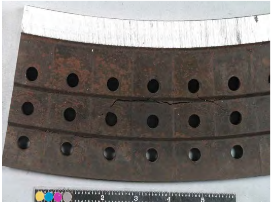
Fig 156 Close-up of SID 14875 subsegment "C4"finger pinned blade attachment shown in Fig. 155, viewed from inlet side.
