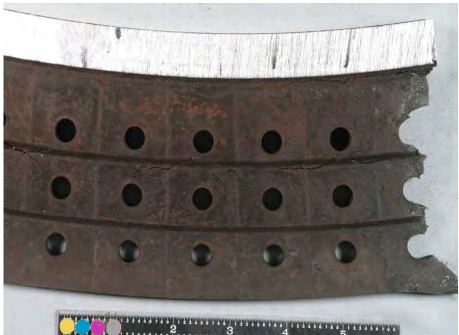
Fig. 157 Close-up of SID 14875 subsegment "C4" finger pinned blade attachment shown in Fig. 155, viewed from inlet side.
