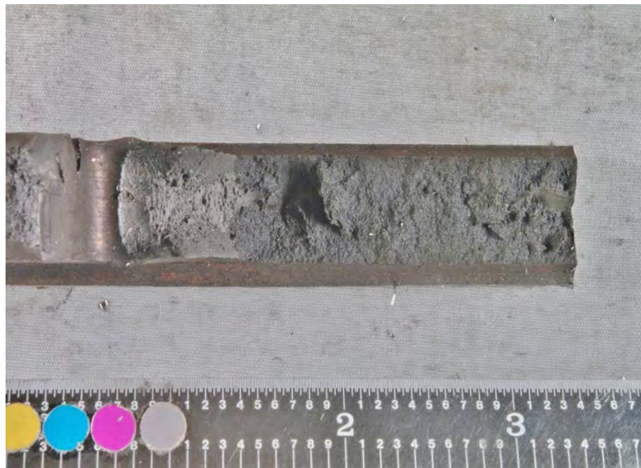
Fig. 135. Close-up photograph of SID 14874 subsegment "A4" fracture surface shown in Fig. 132.
