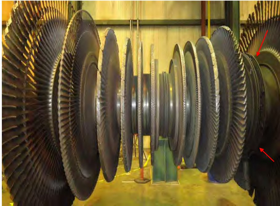
Fig. 56. Photograph of low pressure turbine "B" Rotor showing section of turbine end L-1 stage disk rim which fractured (arrows) through finger root attachments.
