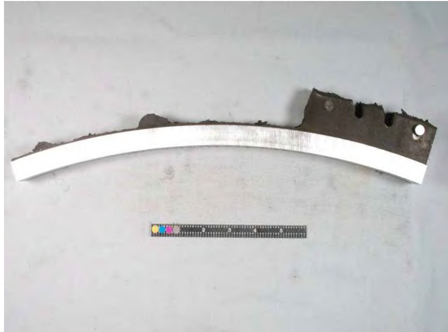
Fig. 138. SID 14875 subsegment "B4" finger pinned blade attachment, outlet side.
