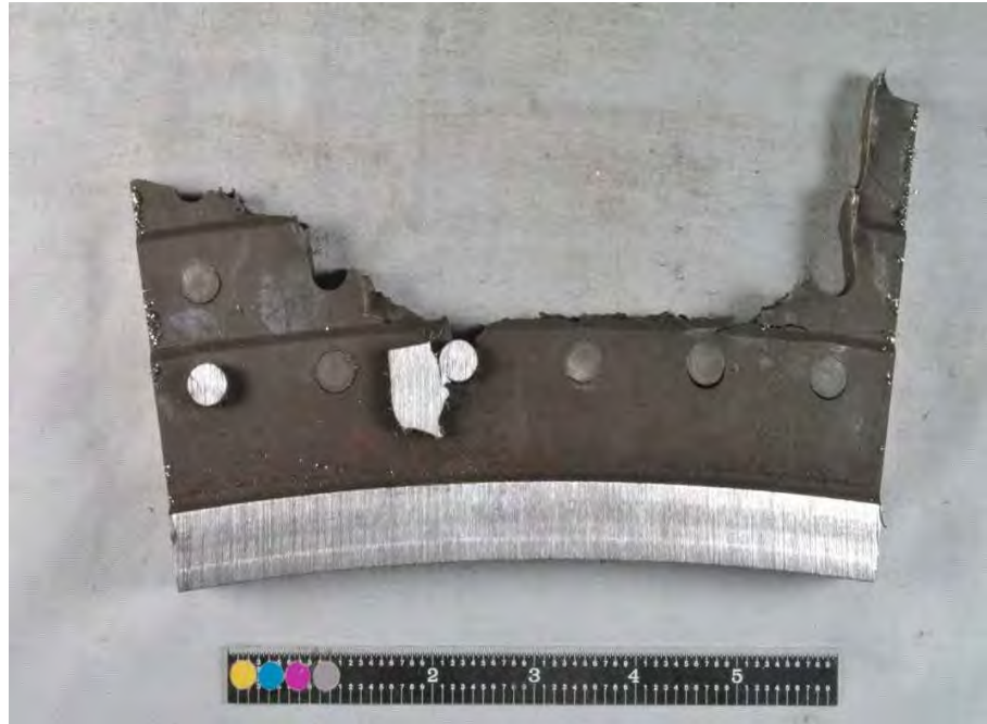
Fig. 126. SID 14874 subsegment "A3" finger pinned blade attachment.
