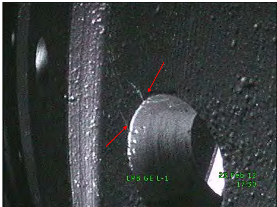
Fig. 89 Close-up blacklight photograph of low pressure turbine "B" L-1 disk rim showing MPI indication (arrows) in finger-root attachment.
