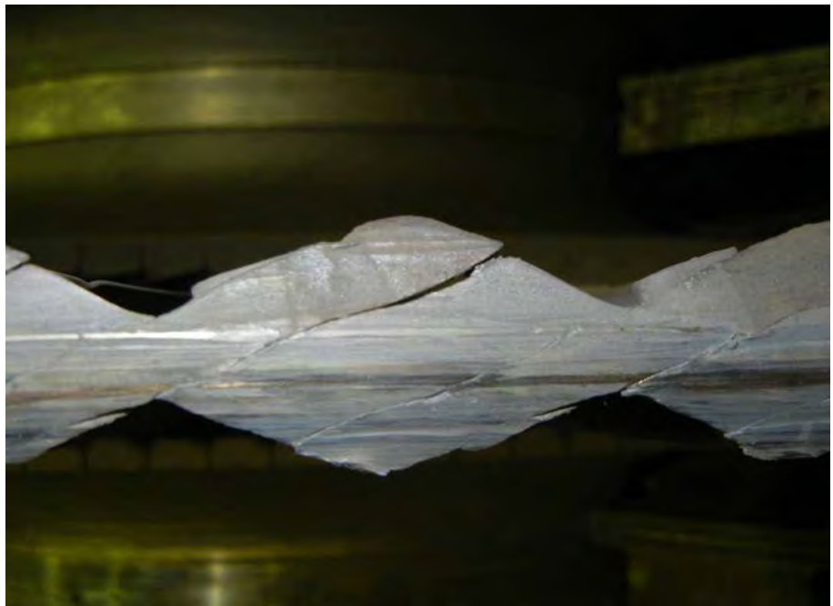
Fig. 71. Close-up photograph of low pressure turbine "B" generator end L-1 blade tips and spacers showing severe rub damage.
