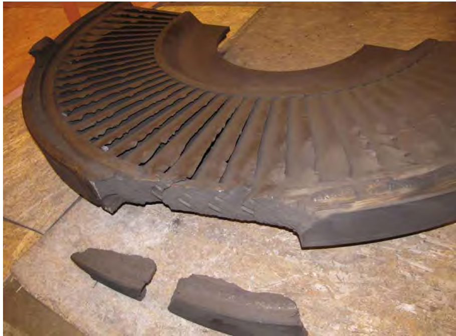
Fig. 78. Photograph of turbine end L-1 stage diaphragm from low pressure turbine "B" rotor showing extent of damage.
