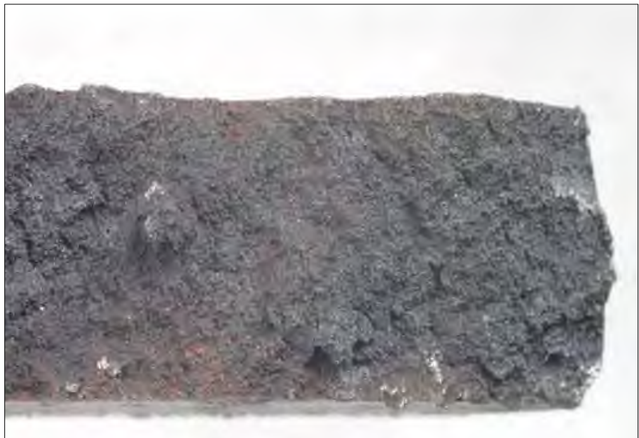
Fig 167. Close-up of surface of fracture through crack No. 1 from SID 14875 subsegment "C4" shown in Fig. 166.
