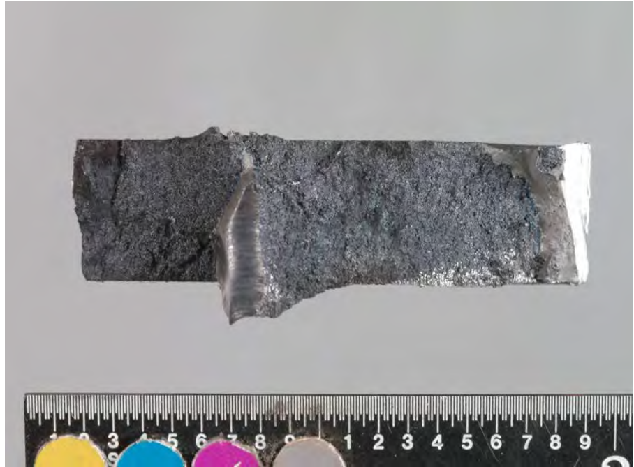
Fig. 168. Close-up of surface of fracture through crack No. 2 from SID 14875 subsegment "C4".
