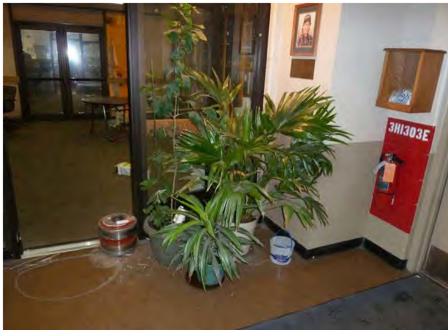
Fig. 110. Photograph of liberated exciter collector which came to rest in operator's room.
