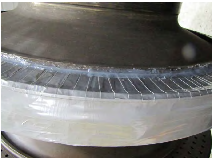
Fig. 85. Close-up of protective tape on fractured L-1 disk rim.
