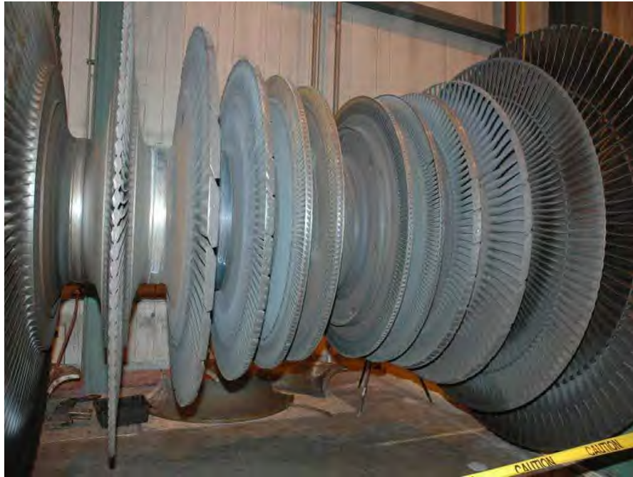
Fig. 46 Photograph of low pressure turbine rotor "A" shown in Fig. 44.
