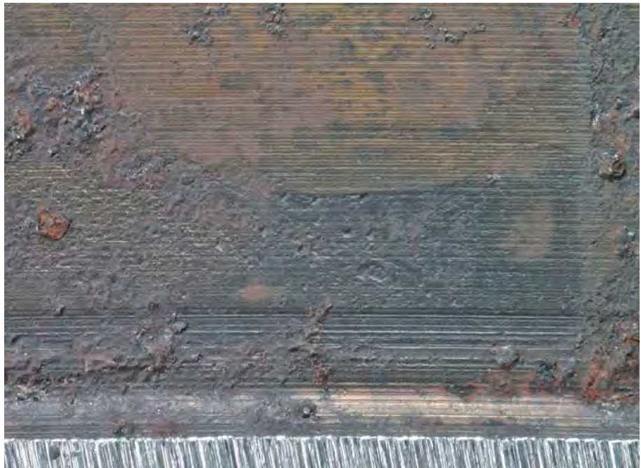
Fig 173. Close-up of finger pinned blade attachment from SID 14875 subsegment "C4" showing extent of corrosion/oxidation, viewed from inlet side.
