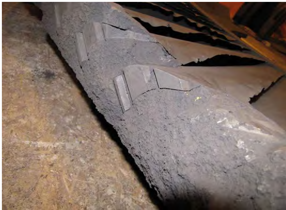
Fig. 79. Close-up photograph of diaphragm fracture surface shown in Fig. 78.
