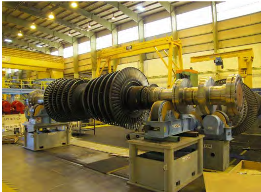
Fig. 31. Photograph of reheat intermediate pressure turbine rotor from the Sherco 3 steam turbine generator train at the Alstom Power, Inc. repair facility.
