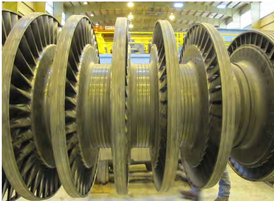
Fig. 13. Close-up photograph of high pressure turbine rotor shown in Fig. 12.
