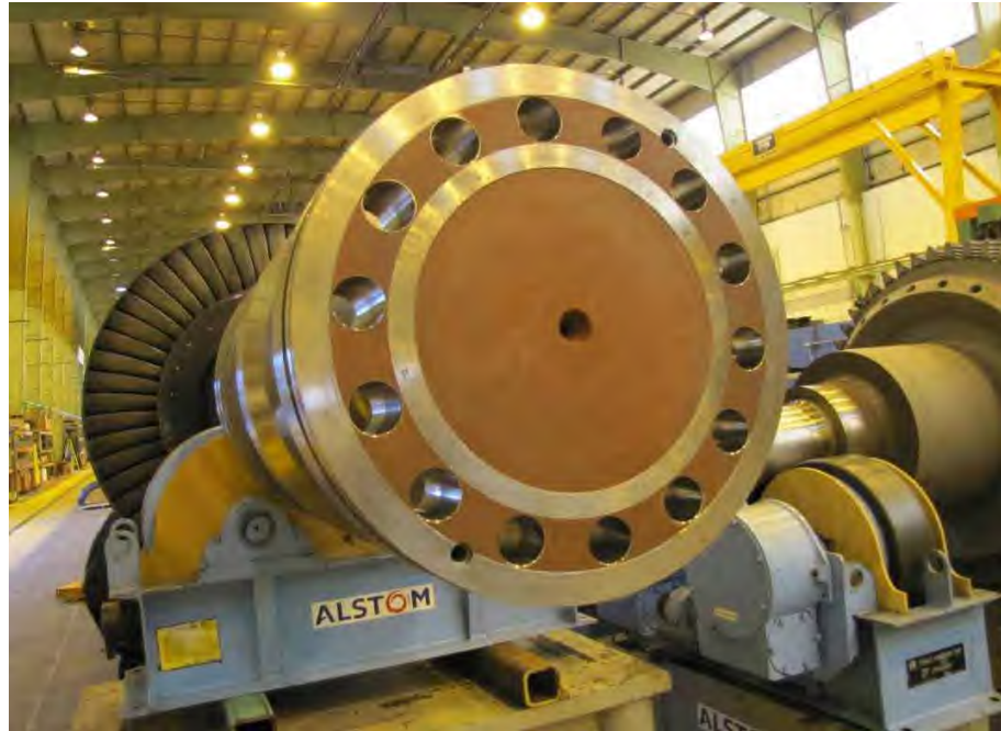
Fig. 42. Photograph of intermediate pressure turbine rotor turbine end coupling.
