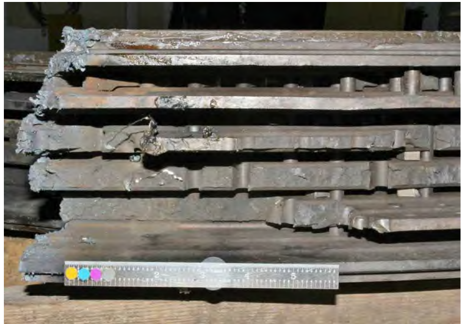
Fig. 121. Close-up photograph of fractures through internal finger pinned blade attachments of the low pressure turbine "B" L-1 disk rim.
