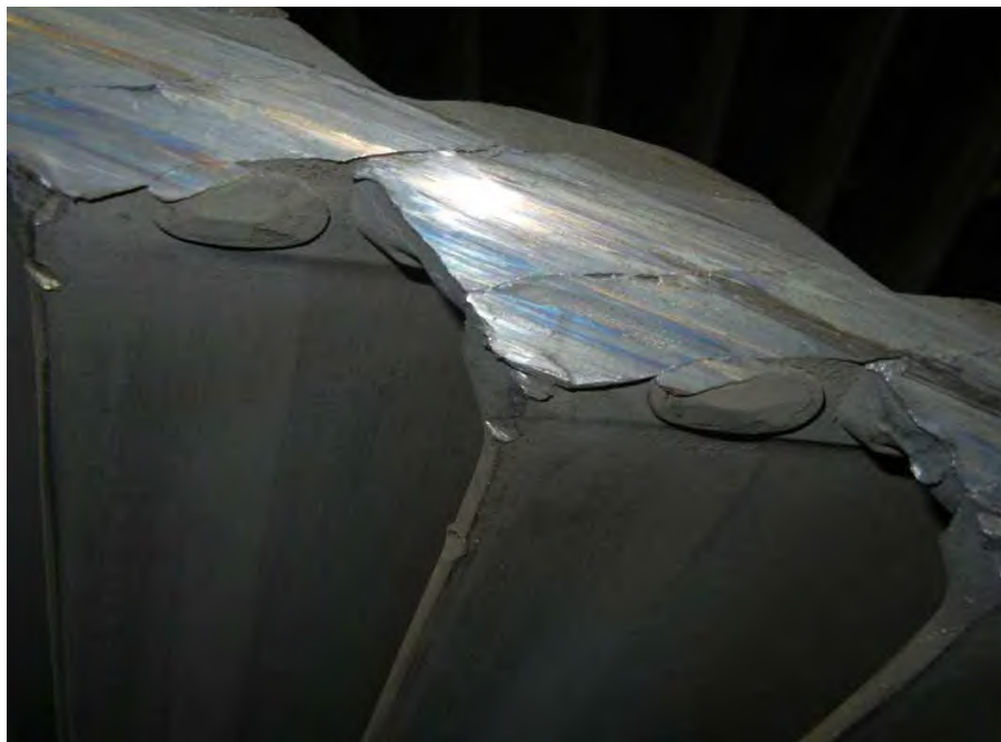
Fig. 72. Close-up photograph of low pressure turbine "B" generator end L-1 blade tips and spacers showing severe rub damage.
