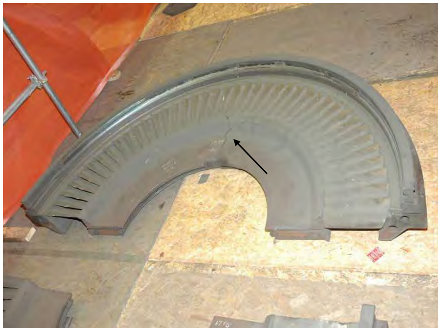
Fig. 75. Photograph of low pressure turbine "B" rotor L-2 stage diaphragm showing radial crack (arrow) through center section and inner wall.
