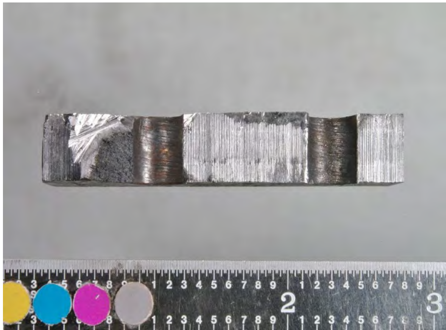
Fig 171. Close-up of surface of fracture through crack No. 3 from SID 14875 subsegment "C4".
