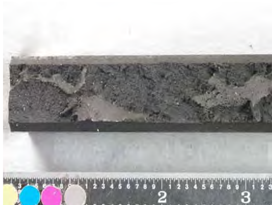
Fig. 147. Close-up of SID 14875 subsegment "B4" fracture surface shown in Fig. 146.
