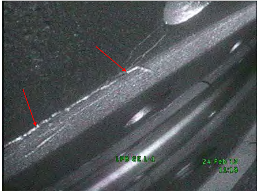
Fig. 88 Close-up blacklight photograph of Low Pressure Turbine "B" L-1 disk rim showing MPI indications (arrows) in finger-root attachment.
