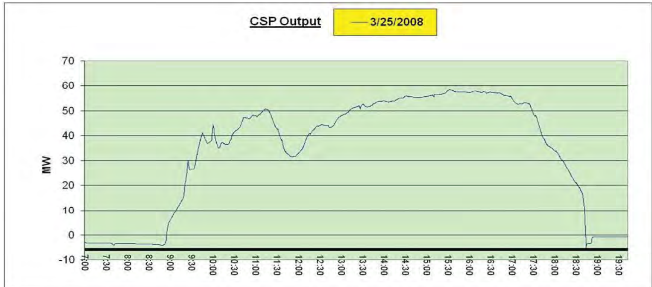
Figure 2.10: Parabolic trough CSP plant on a partly-cloudy day (Sampling time of 10 sec.)
