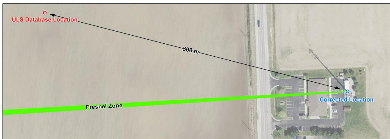
Figure 3: Example of using aerial imagery to correct erroneous ULS database antenna location
