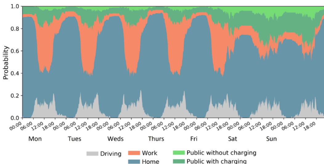
Figure 1. A weekly driving profile generated for personal LDV drivers using 2017 NHTS data and the Markov Chain methodology
