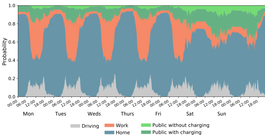
Figure 3. A weekly driving profile generated for personal LDV drivers using 2017 NHTS data and the Markov Chain methodology
