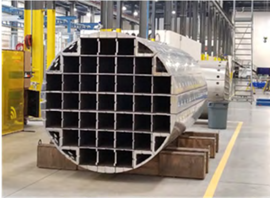
Figure 3. Spent Fuel Canister – End View with Basket for Spent Fuel Assemblies
