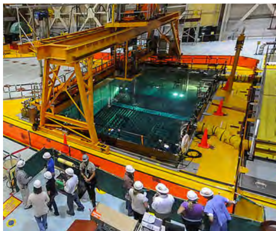
At least 23 feet of water covers the fuel assemblies in the spent fuel pool of Unit 2 at the Brunswick Nuclear Power Plant in Southport, NC. (Courtesy: Matt Born/Wilmington Star-News)
