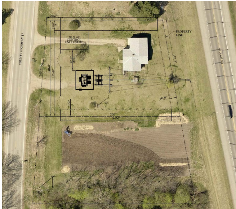
Figure 3 Proposed Substation Layout
