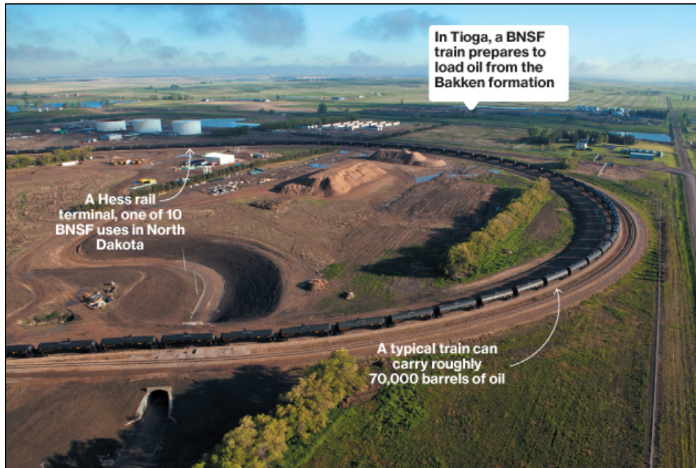
Figure 4. Example of an Origination Terminal
