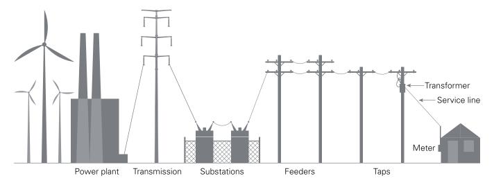
Power is carried to homes or businesses through an electric distribution system. Electricity is generated at a power plant and distributed by high-voltage transmission lines through various distribution systems until it reaches homes or businesses.
