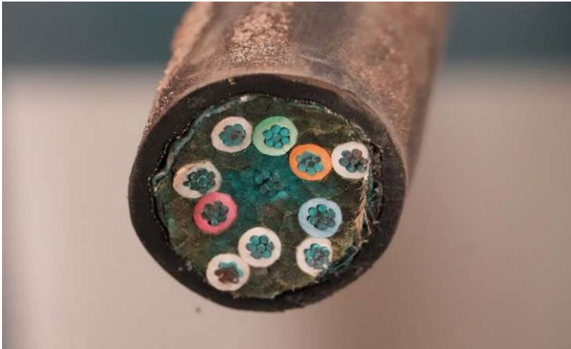
Figure 1 – Control Cable Cross-Section 32
