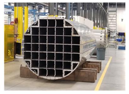
A dry fuel storage system consisting of a canister and other components provides spent fuel containment, radiation shielding, and transportation. Spent fuel assemblies are stored inside a DFS system canister. The specific vendor and spent fuel storage technology selected by Xcel Energy was the NUHOMS. 45 They are designed to store and transport spent fuel and are approved under a general license from the NRC for storage and transport. 46
