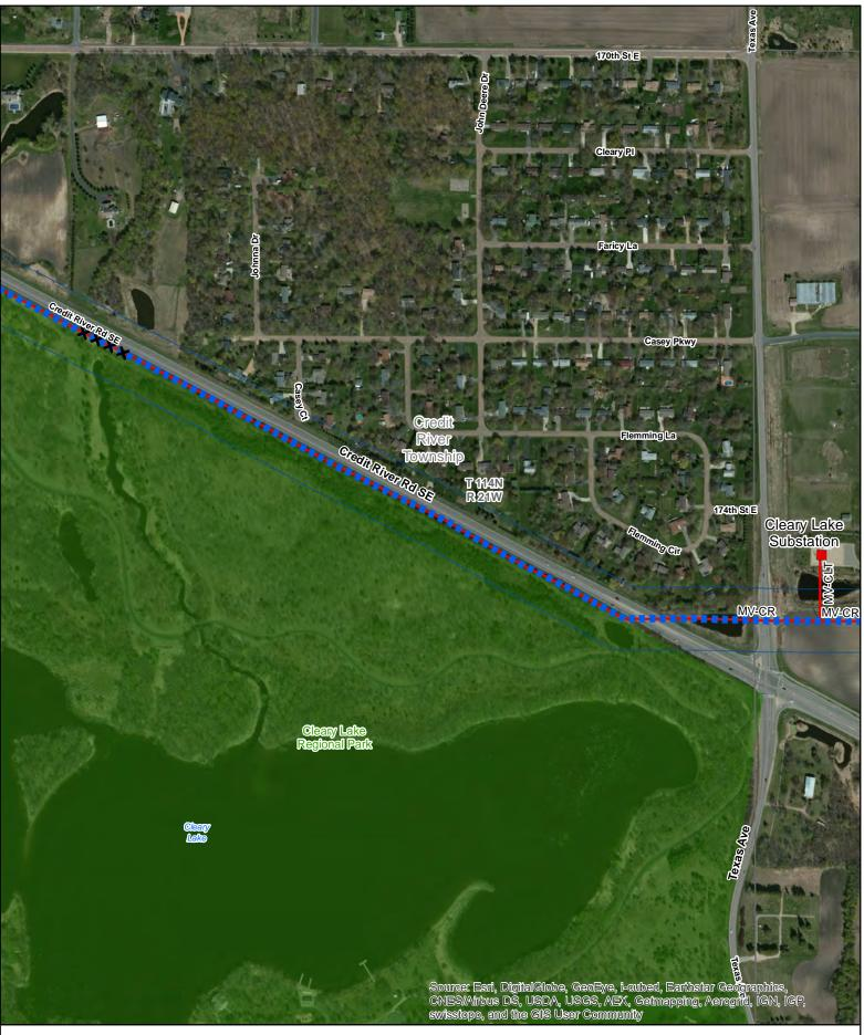
Proposed Great River Energy 115 kV Transmission Line MV-CR Segment Existing Cooperative Distribution Substation Existing Great River Energy 69 kV Transmission Line 300' route width
