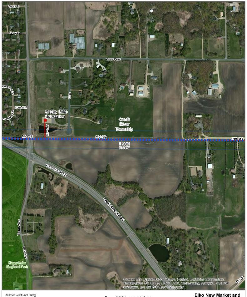
Proposed Great River Energy 115 kV Transmission Line WV-CR Segment Existing Cooperative Distribution Substation Existing Great River Energy 69 kV Transmission Line 300° route width Park
