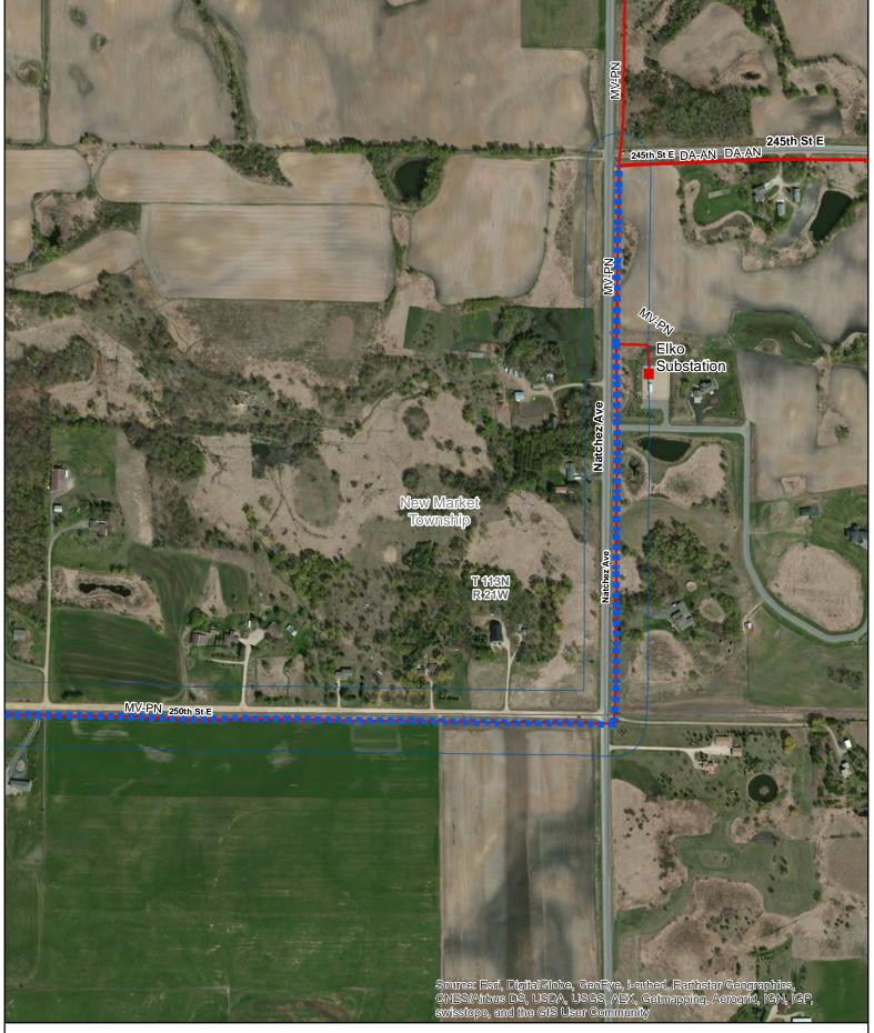
Proposed Great River Energy 115 kV Transmission Line MV-PN South Segment Existing Cooperative Distribution Substation Existing Great River Energy 69 kV Transmission Line 300' route width
