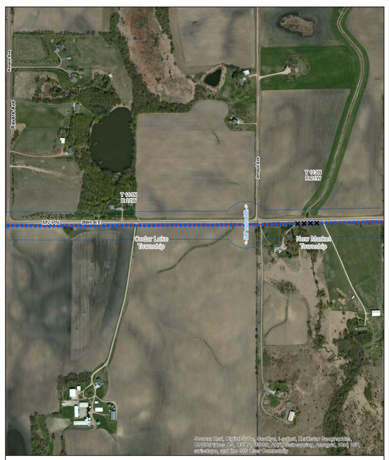
Proposed Great River Energy XX Potential Bird Diverter Locations 115 kV Transmission Line MV-PN South Segment Existing Great River Energy 69 kV Transmission Line 300' route width 500' route width portion
