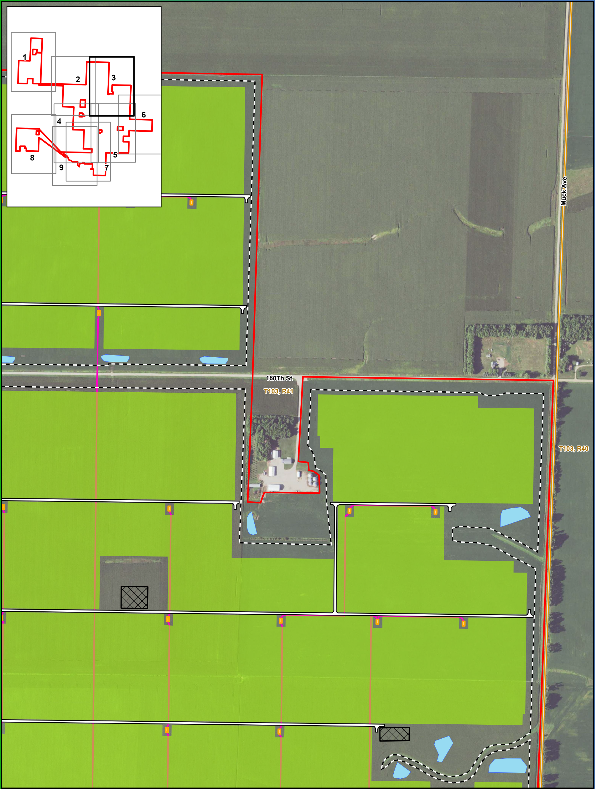
Figure 4 Detailed Preliminary Project Layout Summit Lake Solar and BESS Projects Nobles County, MN
