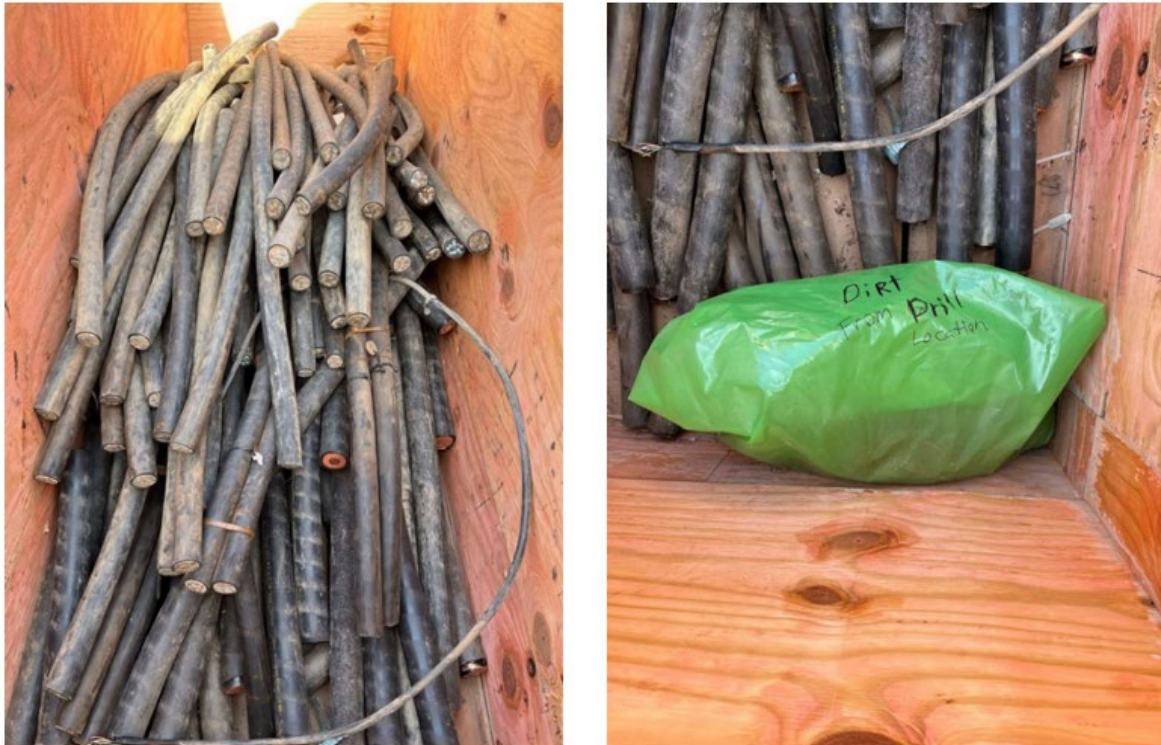
Figure 2 – Cable and Soil Samples Received by EPRI from Xcel 55
