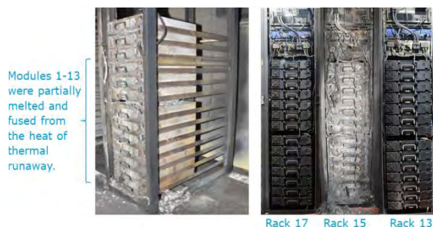
Figure 4: All modules in Rack 15 were severely damaged by thermal runaway while leaving nearby racks mostly intact (image credit: APS)
