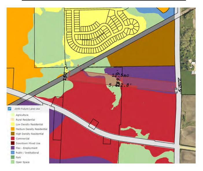
The assumed easement measurements extend 75 feet south and 150 feet north of the existing centerline of the Xcel Energy power line, resulting in an easement width of 225 feet, The total acreage encumbered by easement would be approximately 12.5 acres of anticipated commercial and flex-employment land.
