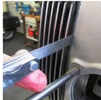
Figure 2 - Example Feeler Gauge Use
