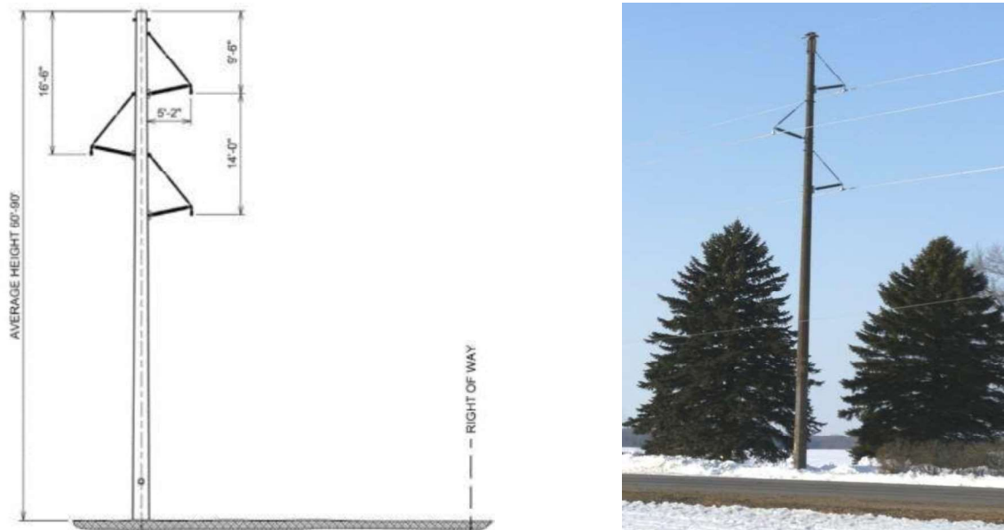
Image 4: Typical Overhead Transmission Line Structure
