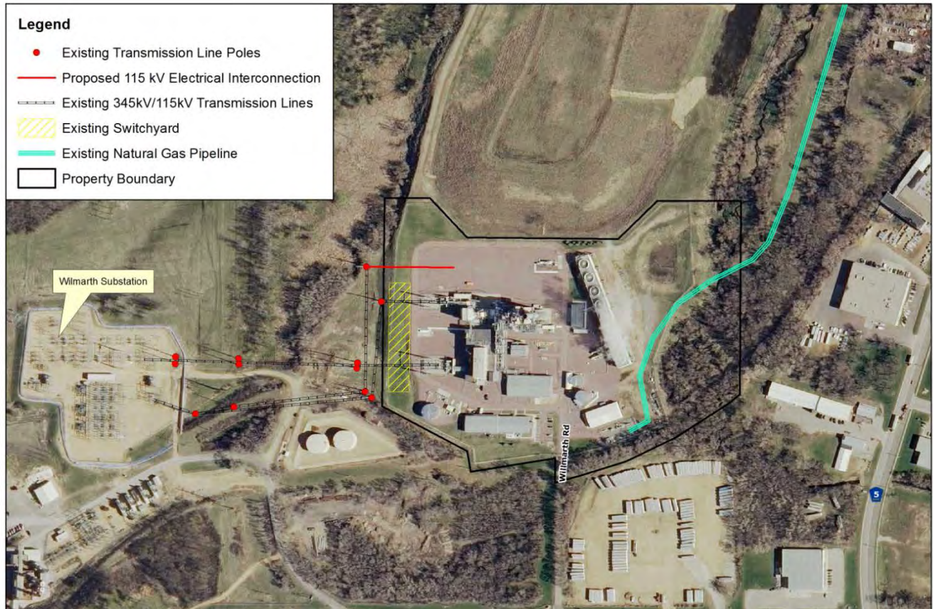
Figure 7. Electrical Interconnection at Mankato Energy Center
