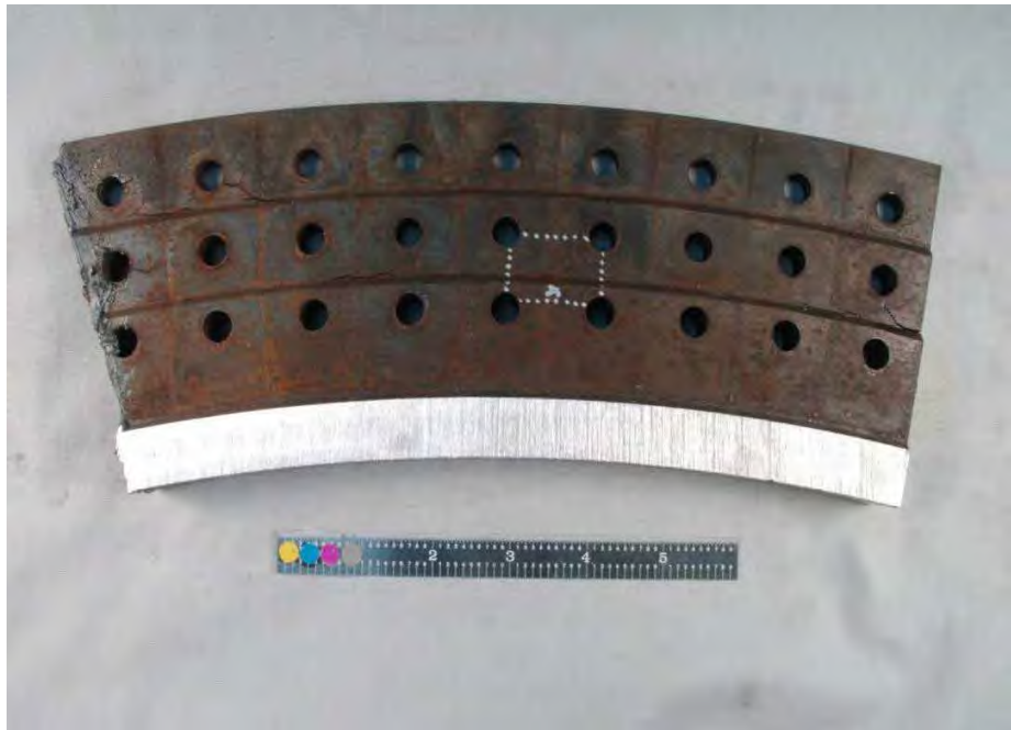
Fig. 241. SID 18475 "D3" finger pinned blade attachment showing location of met Sample L349102.
