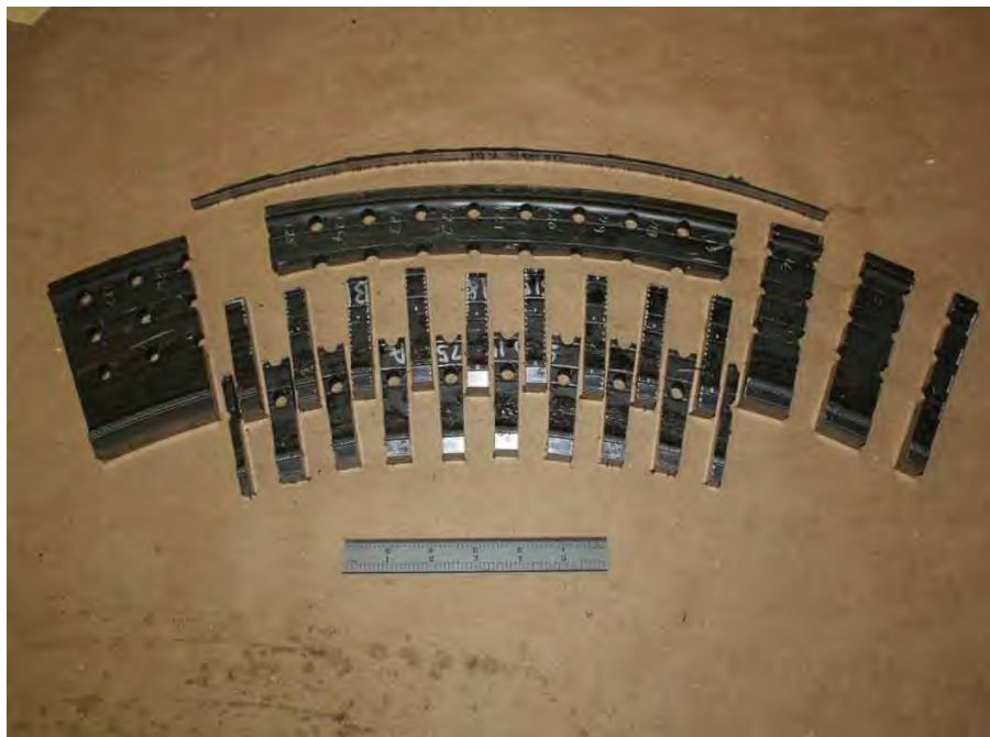
Fig. 227. Mechanical test coupons removed from SID 14875 subsegment "B1".
