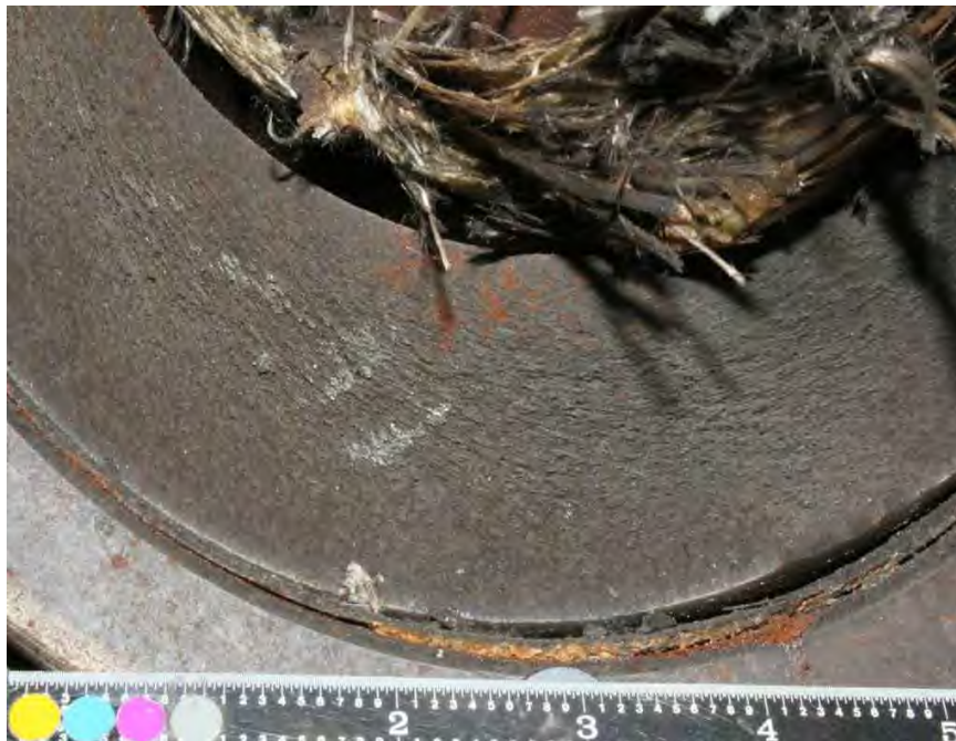
Fig. 314. Close-up photograph of fracture surface of generator shaft aft end fracture half.
