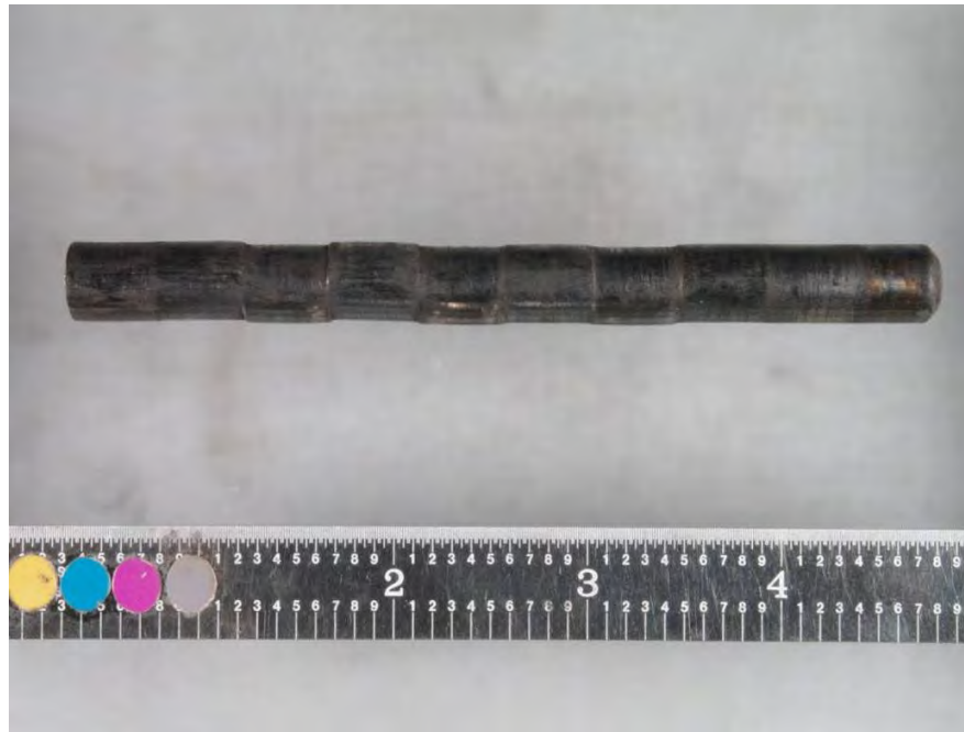
Fig. 296. Photograph of blade pin SID 14936 Pc "C" showing extent of yielding.
