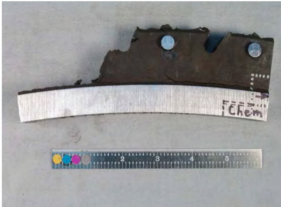
Fig. 267. SID 18474 "A4" finger pinned blade attachment showing location of met Sample L349106.
