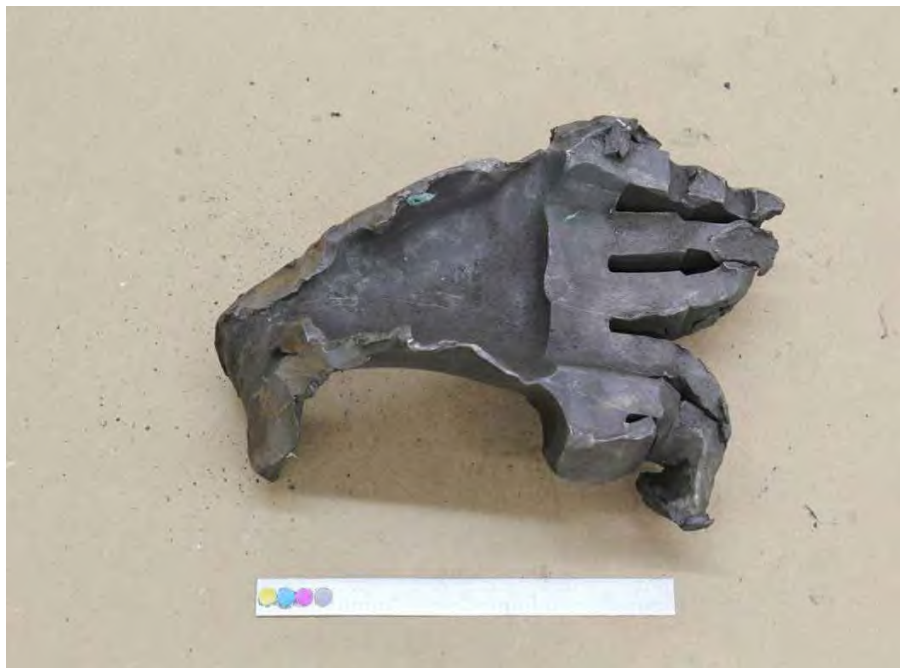
Fig. 279. Photograph of low pressure turbine "B" turbine end L-1 blade which had fractured through the airfoil.
