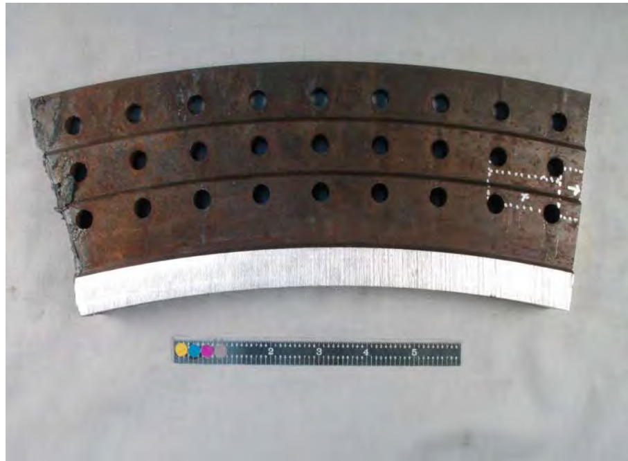
Fig. 248. SID 18475 "D5" finger pinned blade attachment showing location of met Samples L349103 and L349104.
