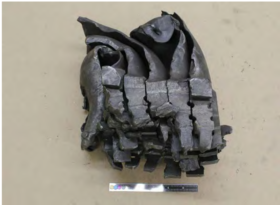
Fig. 275. Photograph of low pressure turbine "B" turbine end L-1 blades recovered at the plant site and received for forensic examination.
