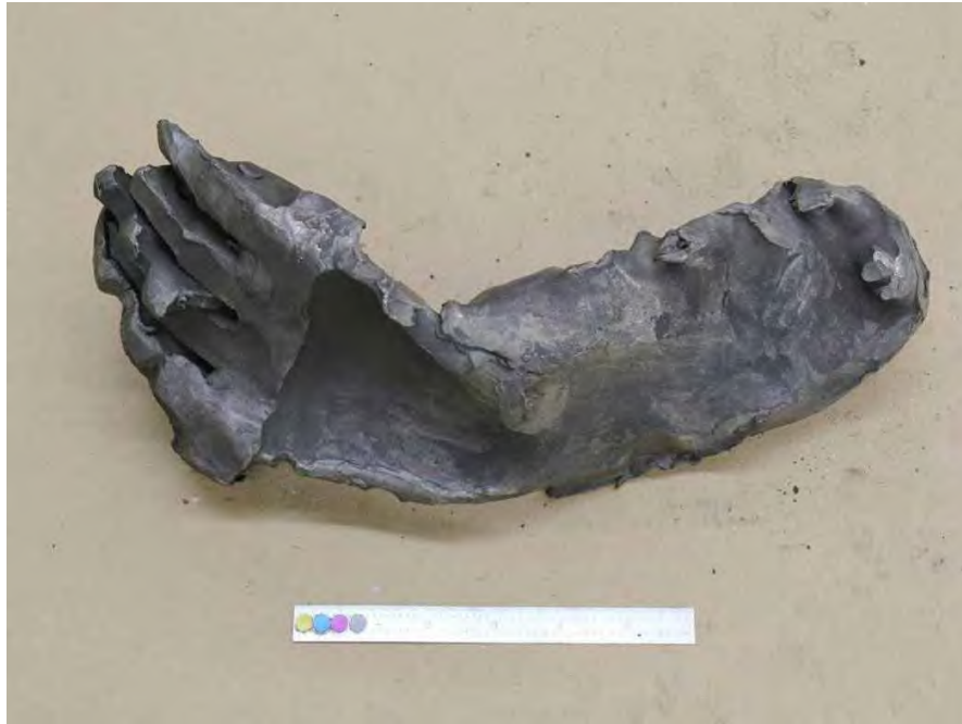
Fig. 276. Photograph of low pressure turbine "B" turbine end L-1 blade recovered at the plant site and received for forensic examination.
