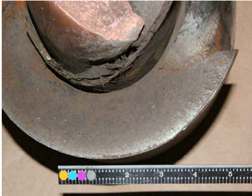
Fig. 317. Close-up photograph of fracture surface of generator shaft forward end fracture half with leads intact.
