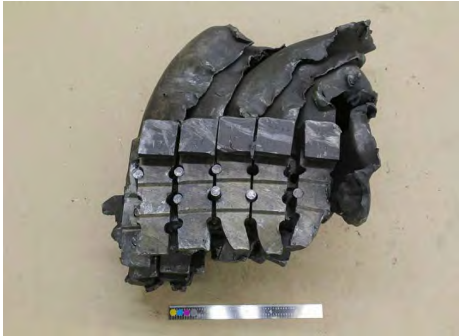
Fig. 274 . Photograph of low pressure turbine "B" turbine end L-1 blades recovered at the plant site and received for forensic examination.
