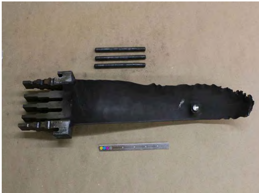
Fig. 277. Photograph of low pressure turbine "B" turbine end L-1 blade removed at the GE Repair Facility in Chicago, IL and received for forensic examination.
