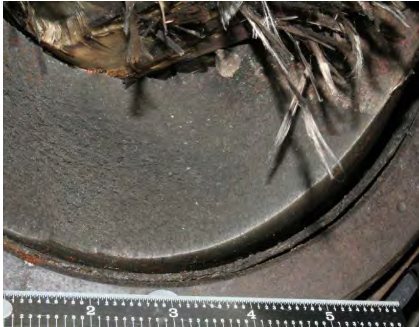
Fig. 315. Close-up photograph of fracture surface of generator shaft aft end fracture half.
