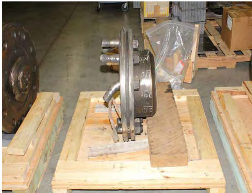
Fig. 312. Generator shaft coupling half which was liberated from generator shaft during turbine event of Nov. 19, 2011.
