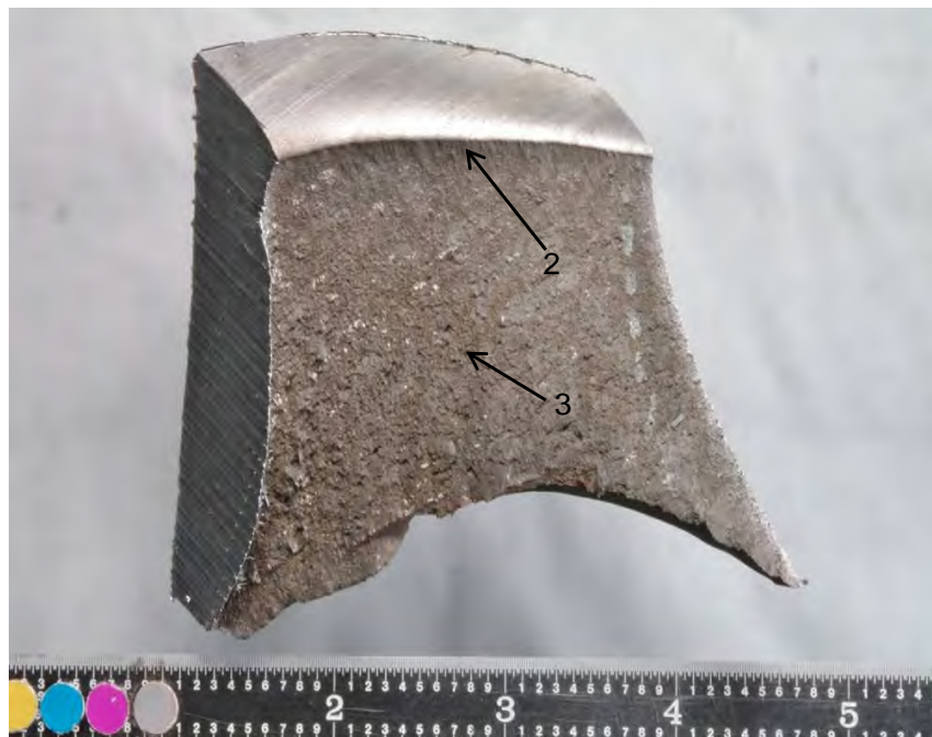
Fig. 324. Close-up photograph of generator shaft fracture subsegment "B" showing locations of scanning electron microscope photograph.
