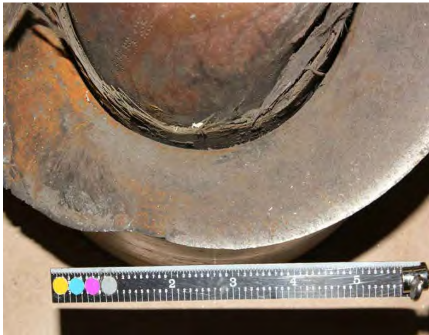
Fig. 318. Close-up photograph of fracture surface of generator shaft forward end fracture half with leads intact.
