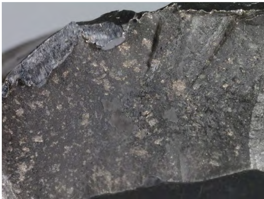
Fig. 285. Close-up photograph of blade airfoil fracture surface shown in Fig. 283.
