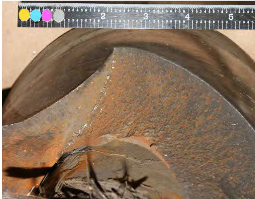
Fig. 319. Close-up photograph of fracture surface of generator shaft forward end fracture half.
