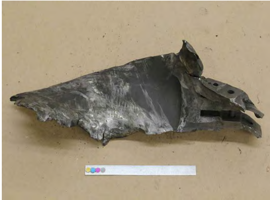
Fig. 280. Photograph of low pressure turbine "B" turbine end L-1 blade which had fractured through the airfoil.
