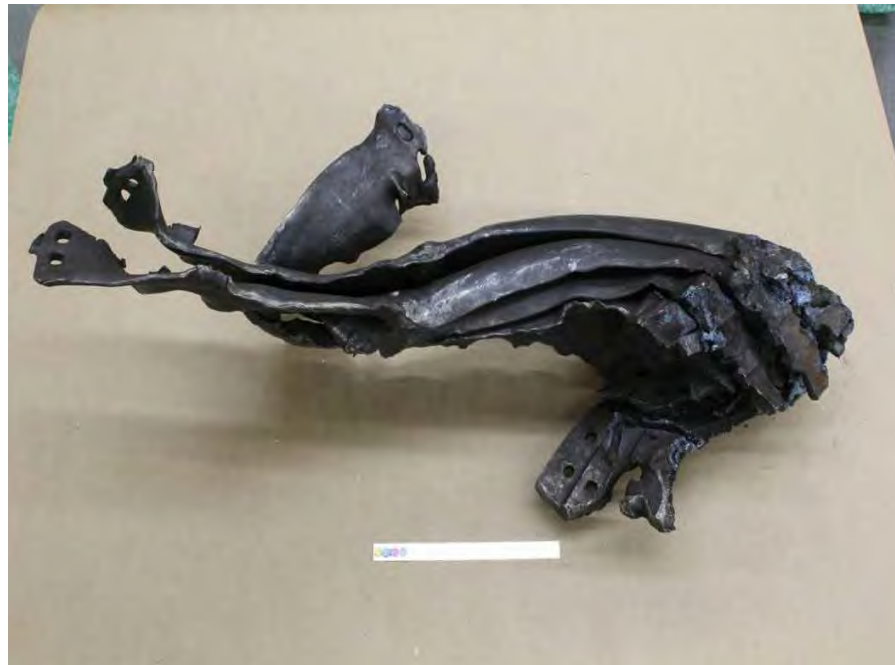
Fig. 273. Photograph of low pressure turbine "B" turbine end L-1 blades recovered at the plant site and received for forensic examination.
