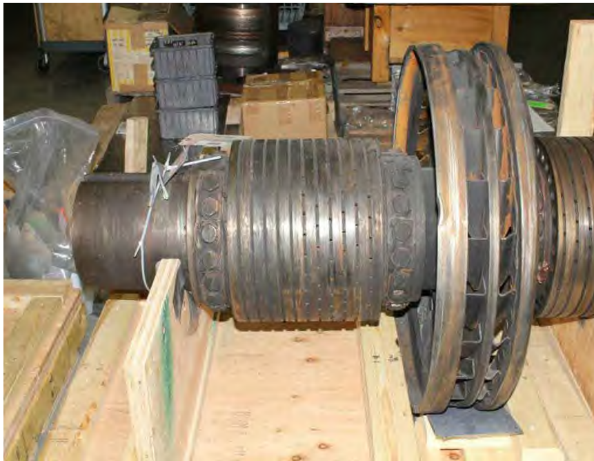
Fig. 309. Aft end of generator shaft.
