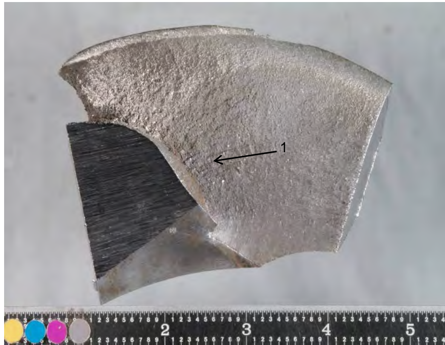
Fig. 323. Close-up photograph of generator shaft fracture subsegment "A" showing location of scanning electron microscope photograph.
