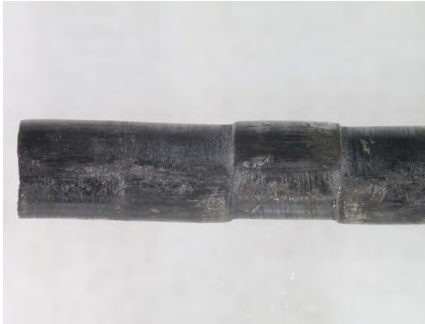
Fig. 298. Photograph of blade pin SID 14936 Pc "C" showing extent of yielding.
