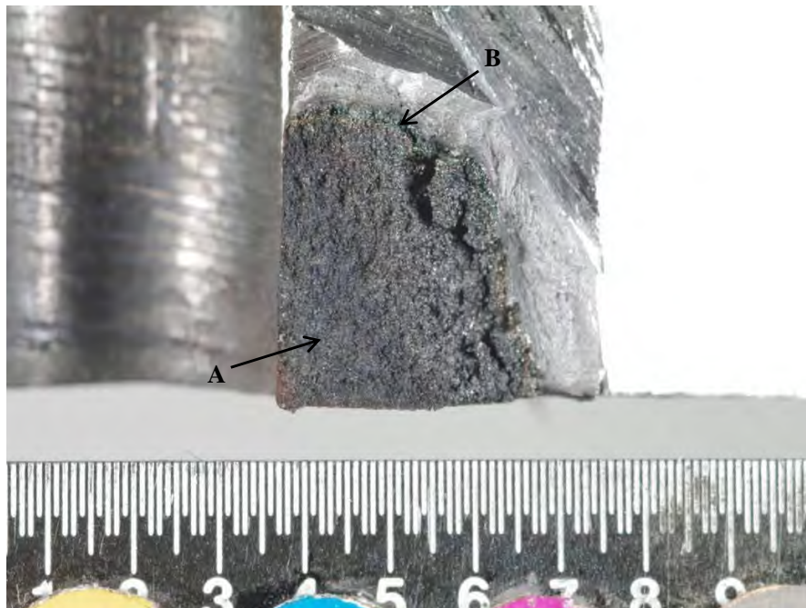
Fig. 190. Photograph of fracture through crack at pin hole in SID 14875 subsegment "C4b" showing areas examined by scanning electron microscope.
