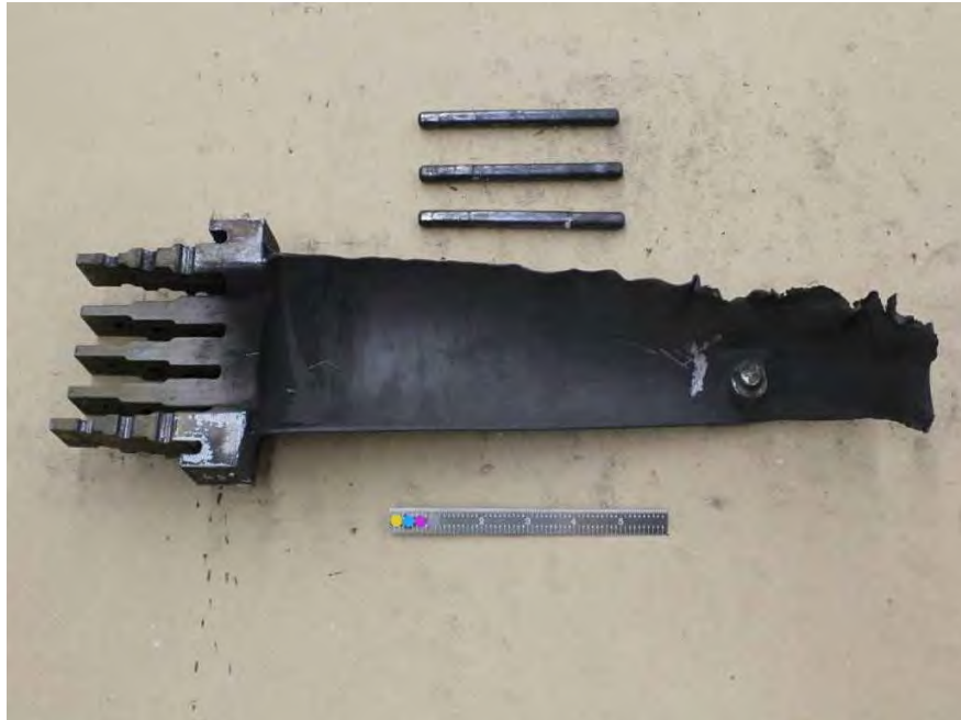
Fig. 292. Photograph of low pressure turbine "B" turbine end L-1 blade and pins received for forensic examination.
