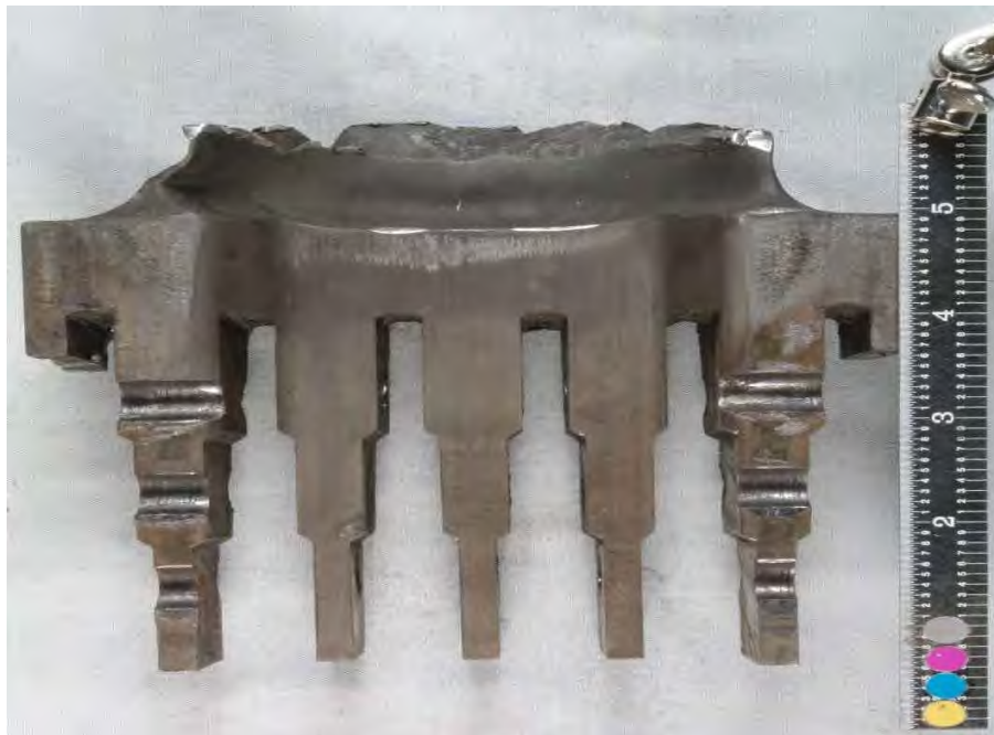
Fig. 281. Photograph of low pressure turbine "B" turbine end L-1 blade which fractured transversely through airfoil just above root platform.
