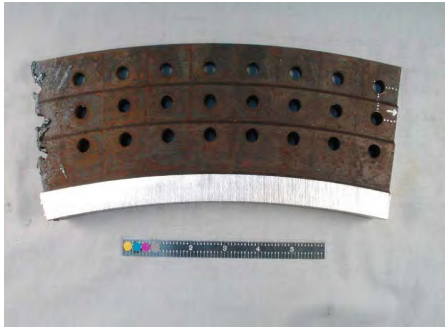
Fig. 228. SID 18475 "D2" finger pinned blade attachment showing location of met sample L349101. Arrow indicates mounting direction.
