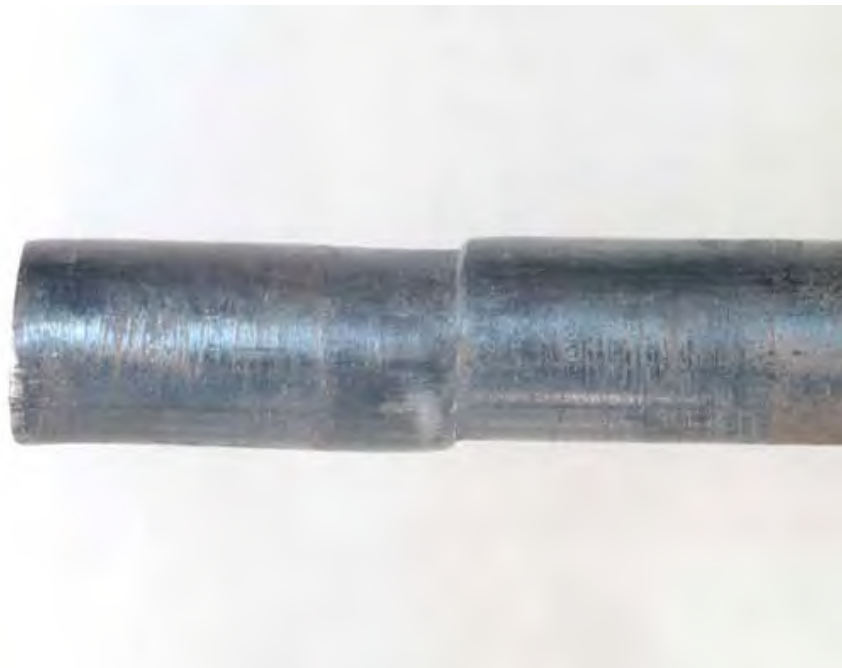
Fig 297. Photograph of blade pin SID 14936 Pc "B" showing extent of yielding.
