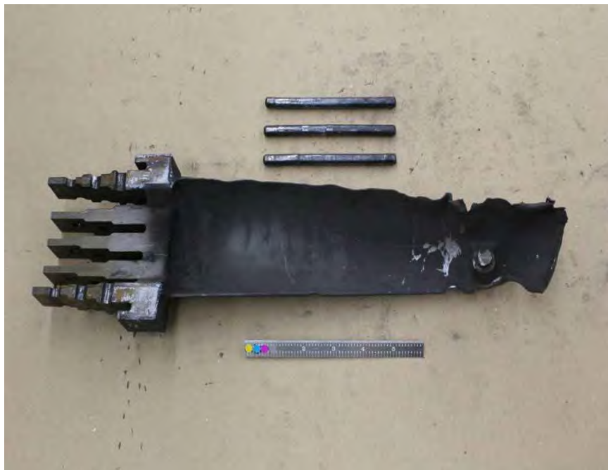
Fig. 293. Photograph of low pressure turbine "B" turbine end L-1 blade and pins received for forensic examination.
