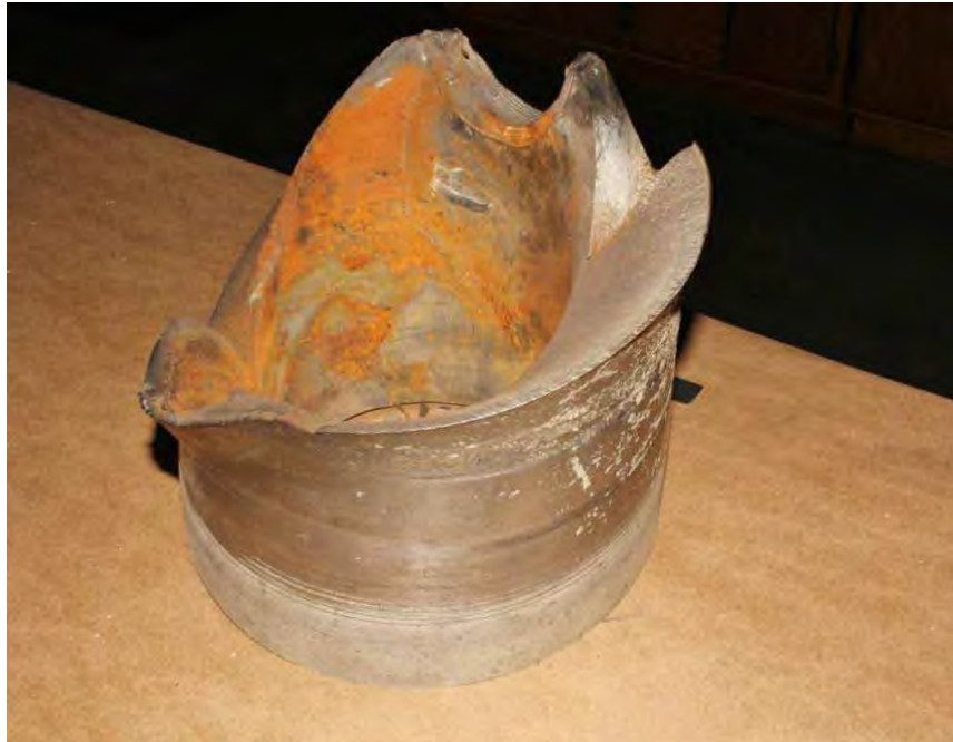
Fig. 311. Forward half of generator shaft fracture with leads removed.
