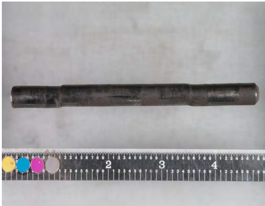
Fig. 295. Photograph of blade pin SID 14936 Pc "B" showing extent of yielding.
