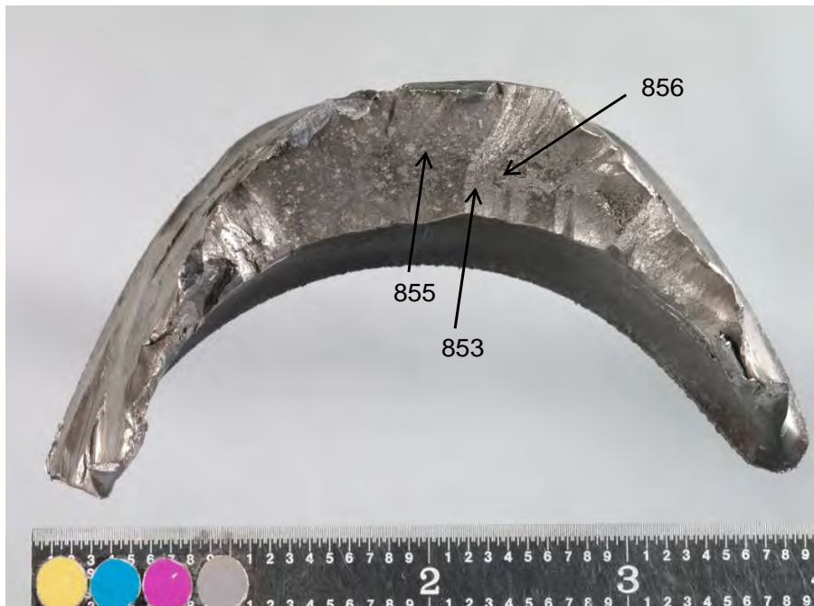
Fig. 283. Close-up photograph of blade airfoil fracture shown in Fig. 281.
