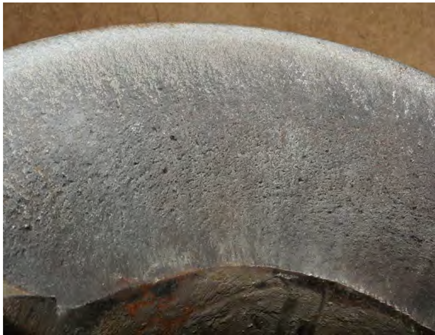
Fig. 320. Close-up photograph of fracture surface of generator shaft forward end fracture half.
