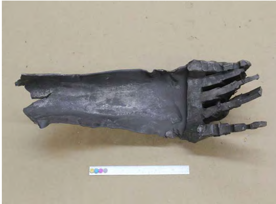
Fig. 278. Photograph of low pressure turbine "B" turbine end L-1 blade which had fractured through the airfoil.
