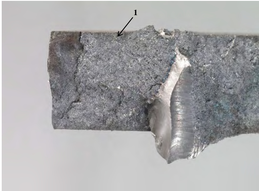
Fig. 219. Photograph of SID 14875 "C4d" fracture, after cleaning, showing areas examined by Scanning Electron Microscopy.
