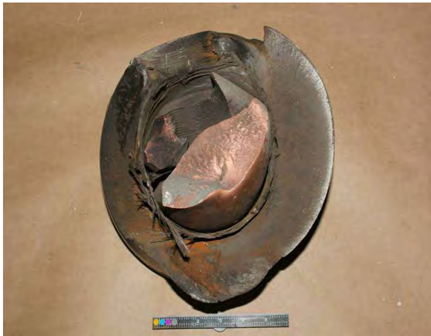
Fig. 316. Close-up photograph of fracture surface of generator shaft forward end fracture half with leads intact.
