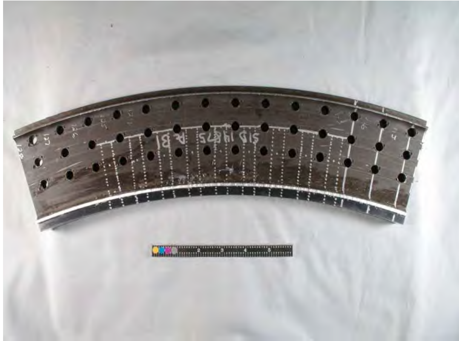
Fig. 226. SID 14875 subsegment "B1" showing layout of mechanical test coupons.
