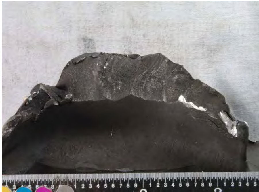
Fig. 282. Close-up photograph of blade airfoil fracture shown in Fig. 281.
