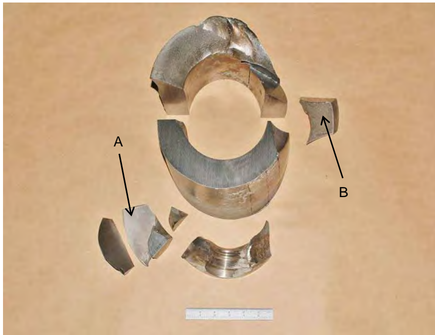
Fig. 322. Close-up photograph of generator shaft forward end fracture half showing two subsegments removed for scanning electron microscope examination.
