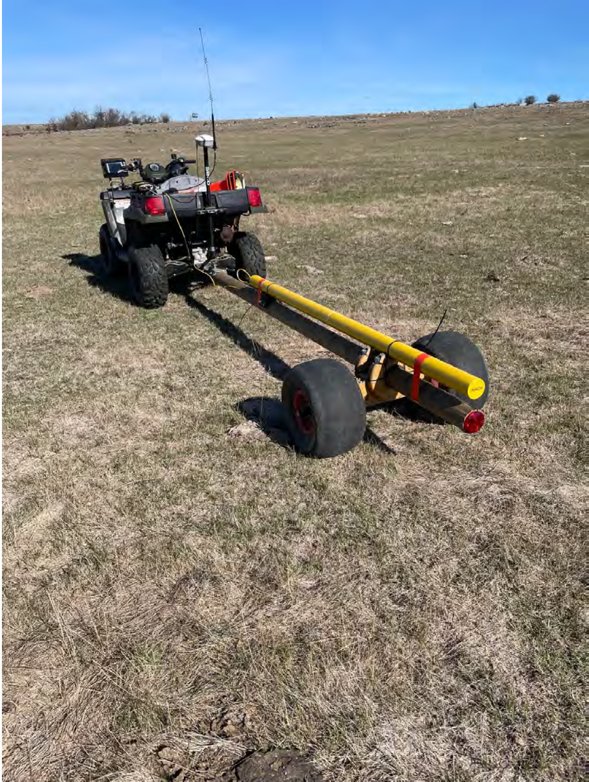
Figure 3. The Tremaine DualEM 21 frequency-domain electromagnetic induction (EMI) instrument utilized in the geophysical survey.
