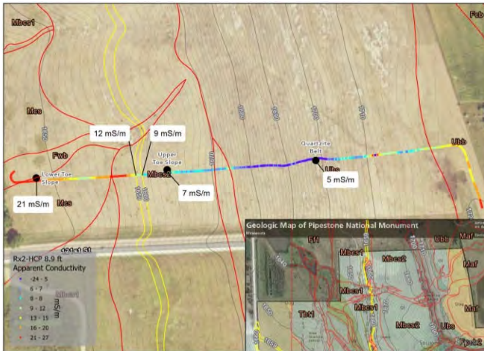
Figure 9. Apparent conductivity at Location A showing locations of baseline data collection.
