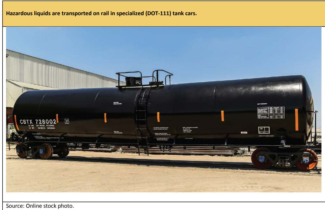
Figure 2-2 Example of DOT-111 Tank Car
