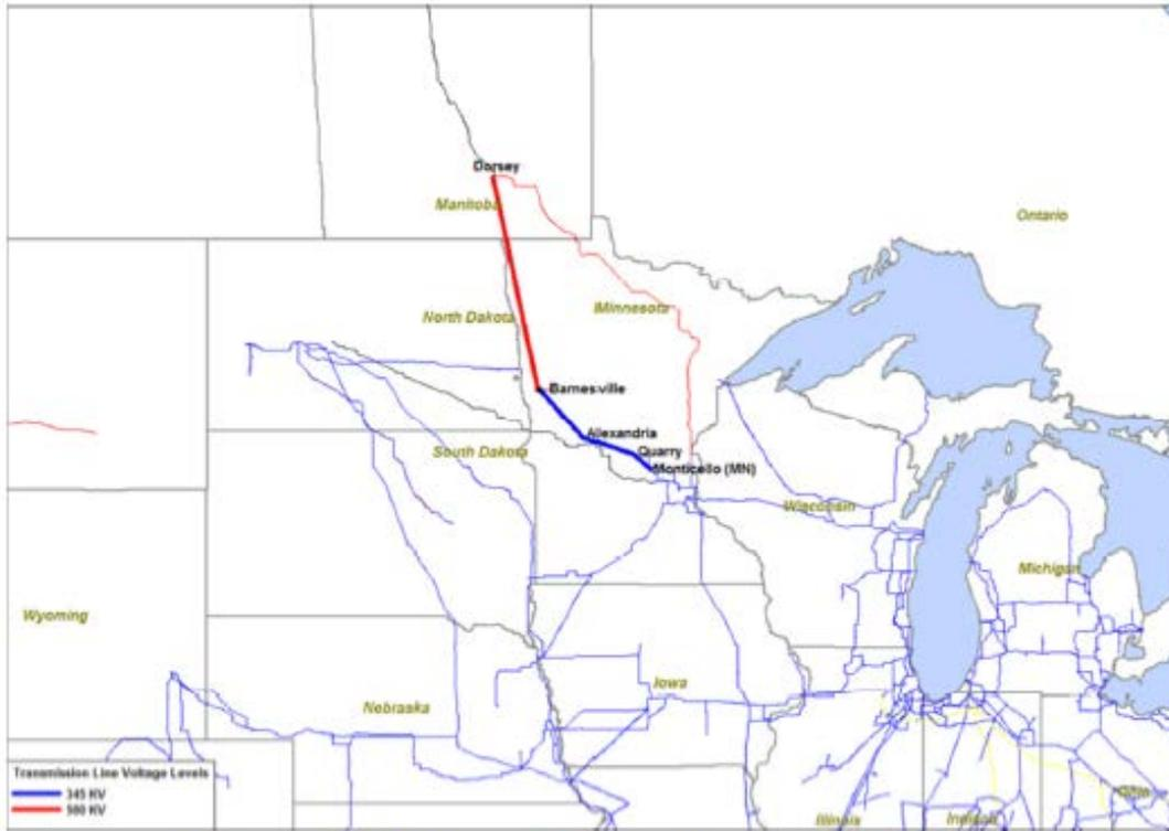
Figure 1-4: Manitoba – Fargo Area 500 kV Tie-Line
