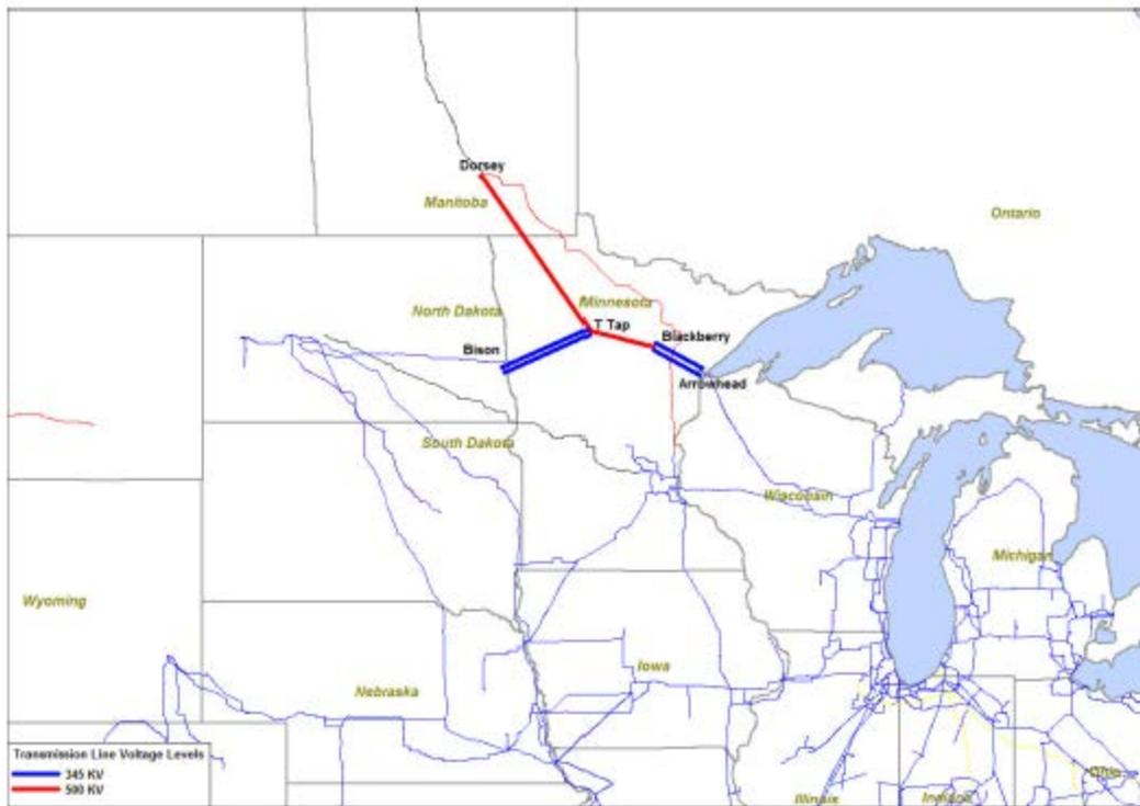
Figure 1-5: Manitoba – Fargo and Duluth “T” 500 kV Tie-Line
