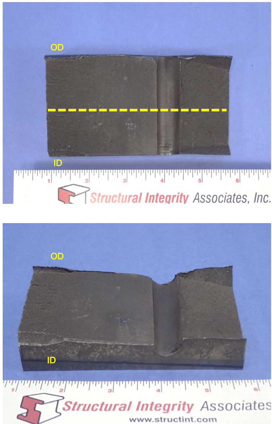
Figure 58. Views of a reduced section that was cut from the sample shown in Figure 55. The dashed line shows the location where this sample was cut to remove the area of interest near the retaining ring ID surface.
