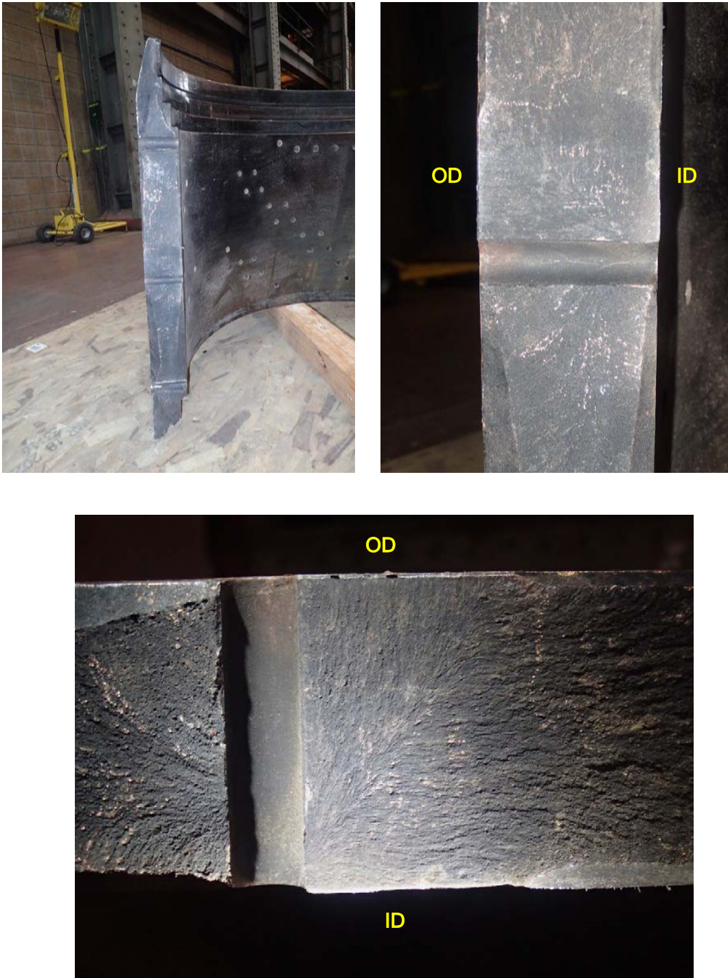
Figure 32. Views of the lower fracture surface on the retaining ring. The upper right image is a closer view of the area near the central cooling passage, and the lower image is a closer view of the same area (rotated 90 degrees clockwise) with side lighting to highlight the fracture surface texture.
