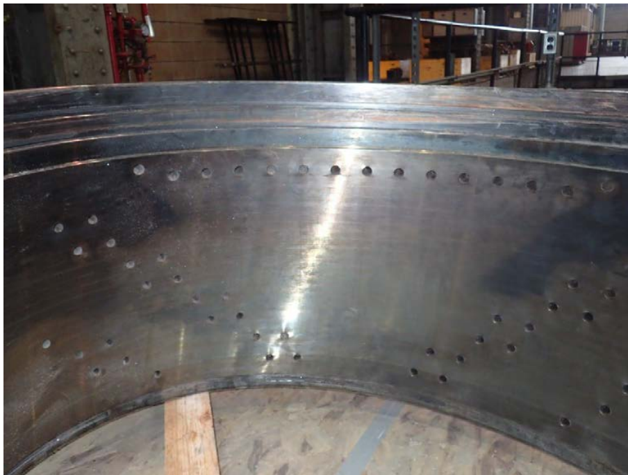
Figure 26. Views of the ID surface of the retaining ring showing the lower fracture surface (arrow) and a location near the lower fracture surface (lower image). The outboard edge of the retaining ring is oriented down in these images.
