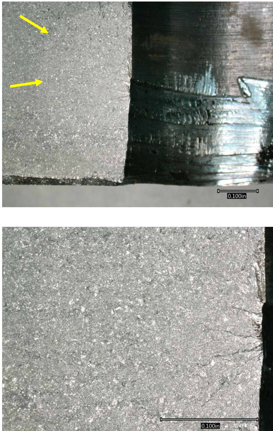
Figure 67. Digital microscope images of the cleaned crack origin area. The lighter thumbnail feature is visible in the upper image (arrows), and the lower image is a closer view of the origin at the cooling passage. Ridges (ratchet marks) extending outward from the origin area are approximately 50 mils (0.050 inches) in length.
