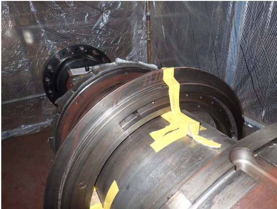
Figure 22. Closer views of the centering ring, which is temporarily supported by wooden blocks and tape.
