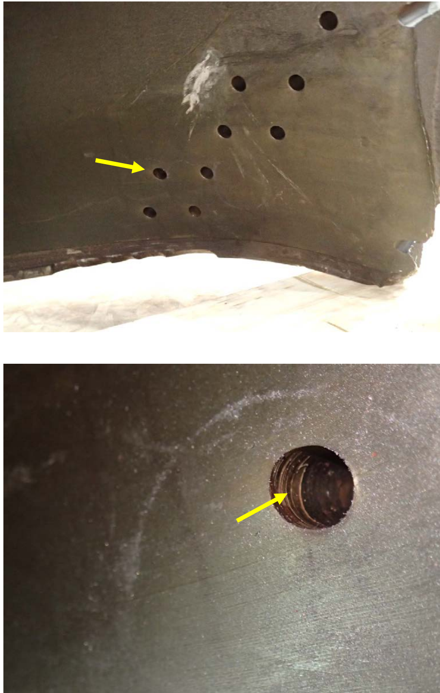
Figure 43. Additional views of a cooling passage hole with internal damage near the ring ID surface (arrow). The area shown is close to the upper fracture surface, which is toward the right in each image.
