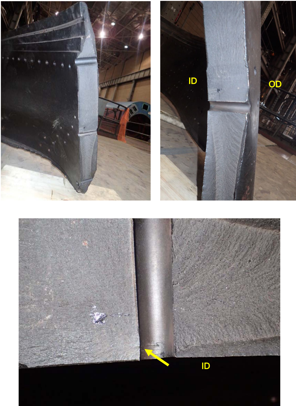
Figure 37. Views of the upper fracture surface on the retaining ring. The upper right image is a closer view of the area near the central cooling passage, and the lower image is a closer view of the same area (rotated 90 degrees counterclockwise); the shiny spot in the lower image is remnant material from the RepliSet sampling. The apparent origin area at the edge of the cooling passage hole is indicated by the arrow.
