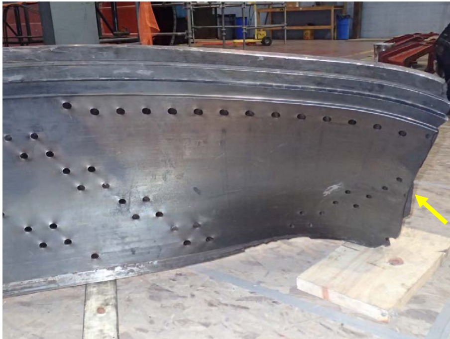
Figure 27. Additional views of the ID surface of the retaining ring, including the upper fracture surface (arrow). In the upper image, visible light variations around the cooling passage holes are due to deformation (elongation) of the ring metal in the areas around the holes.
