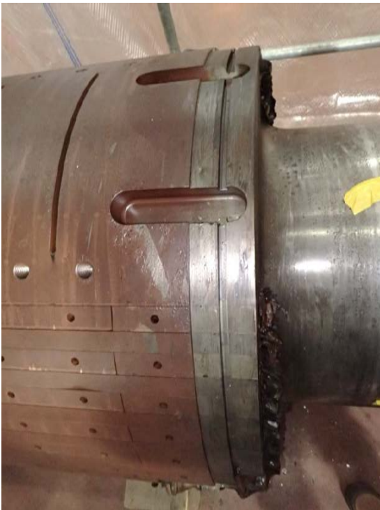
Figure 23. Additional views of the centering ring (upper image) and rotor windings in proximity to the snap ring slot. Localized damage to the rotor is visible in the lower-right image.
