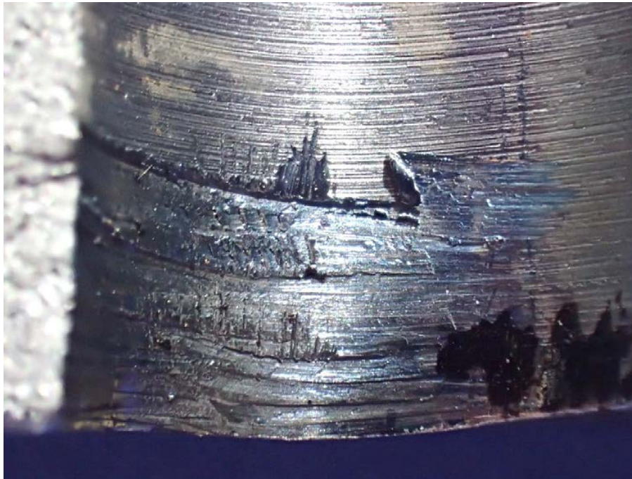
Figure 65. Close views of the cooling passage near the ring ID surface, after cleaning in an ultrasonic bath. Locations with mechanical damage exhibited a bluish tint after cleaning.
