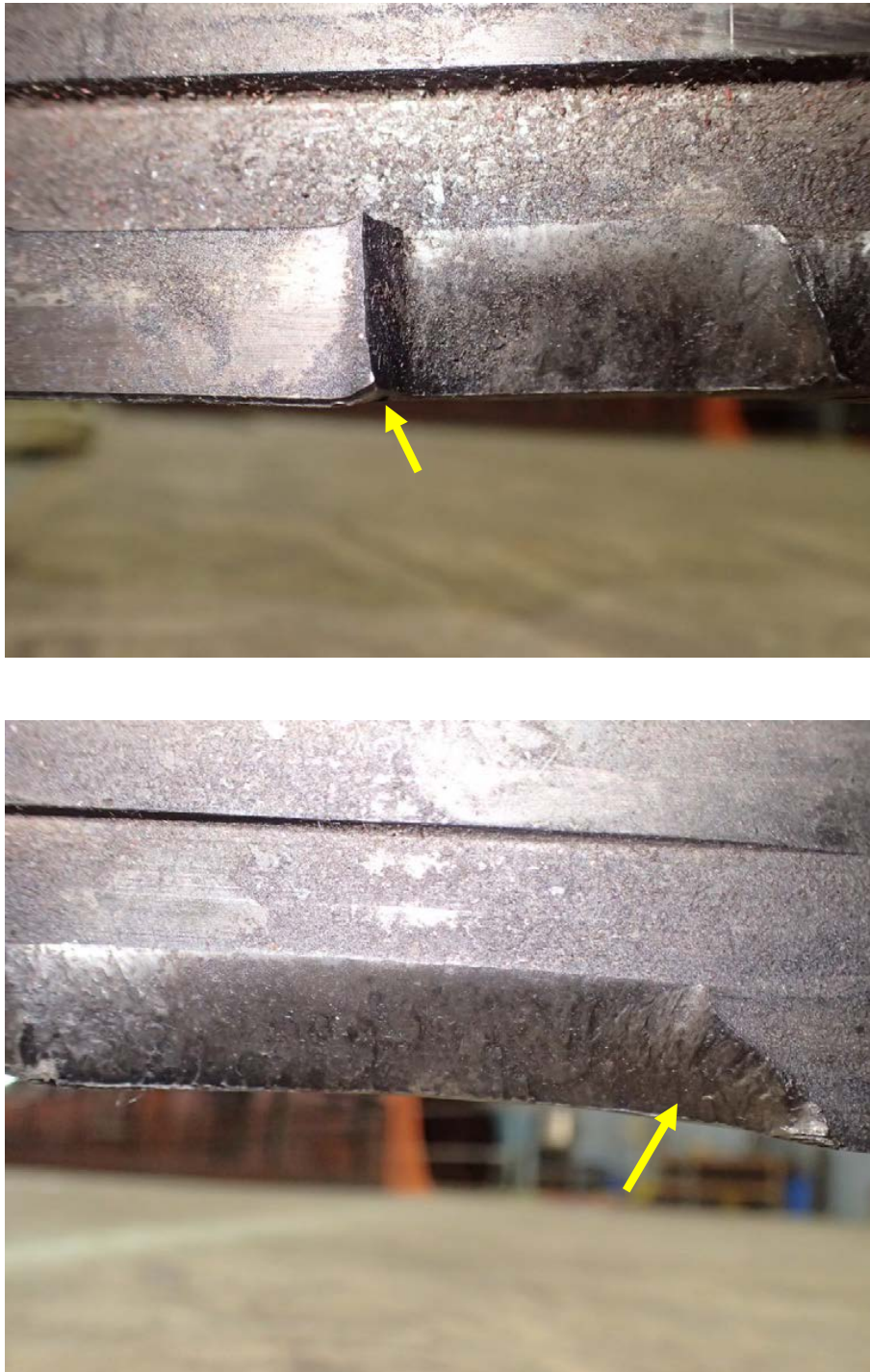
Figure 31. Close views of the mechanical damage at the outboard edge of the retaining ring. These features were along one side of one of the intermittent slots, and exhibited deformation and sheared metal (indicated by the arrows) that indicated mechanical impact from the outside toward the inside.
