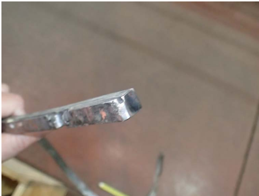
Figure 48. Close views of the other end of the snap ring shown in Figure 45. This end was damaged but not fractured, and the tool fitting has broken off at the location of the pins (visible in the upper image).
