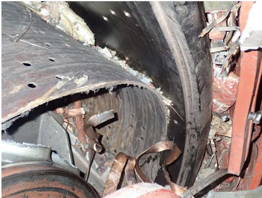
Figure 7. Closer views of the ID surface and outboard (south) edge of the retaining ring. These images also show portions of the fiberglass liner that was situated just on the inside of the retaining ring prior to the failure event.
