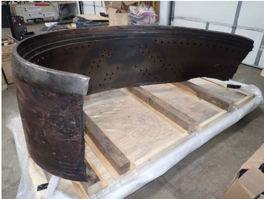
Figure 51. Additional views of the retaining ring in the as-received condition at SI's metallurgical laboratory.
