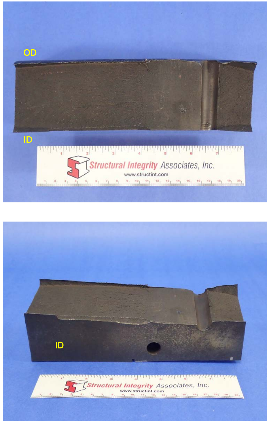
Figure 55. Views of the fracture region of interest (adjacent to the central cooling hole on the upper fracture surface) after removal from the retaining ring.
