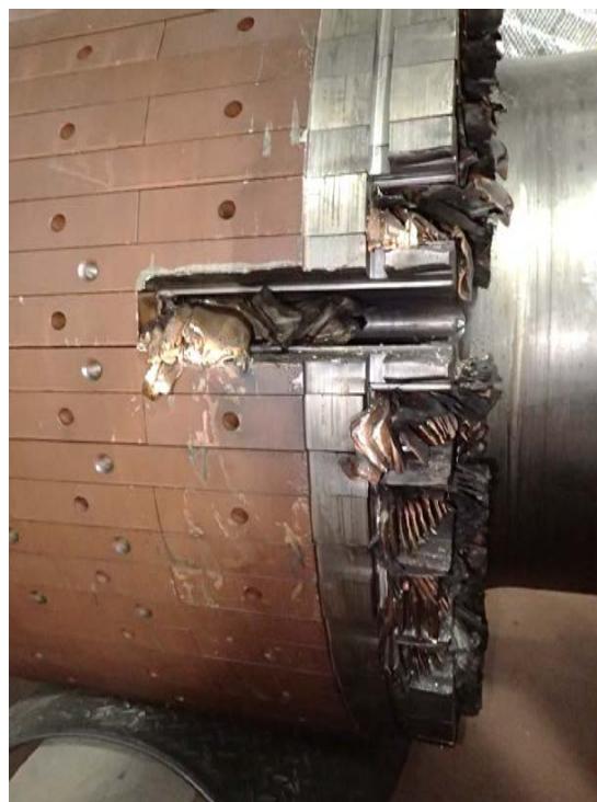
Figure 23. Additional views of the centering ring (upper image) and rotor windings in proximity to the snap ring slot. Localized damage to the rotor is visible in the lower-right image.
