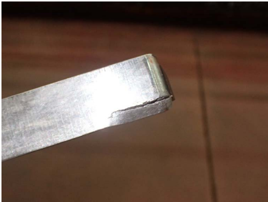
Figure 49. Views of deformation and damage on a ring attachment (key) component.
