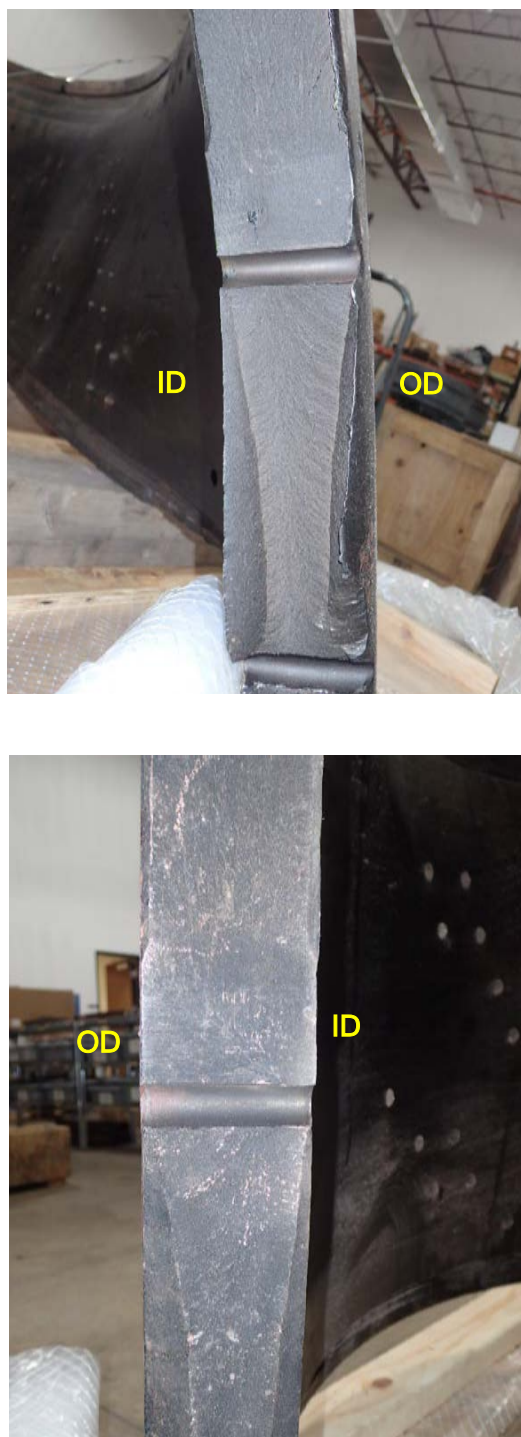
Figure 52. Views of the central cooling passage on the upper (upper image) and lower (lower image) fracture surfaces of the retaining ring, in the as-received condition.
