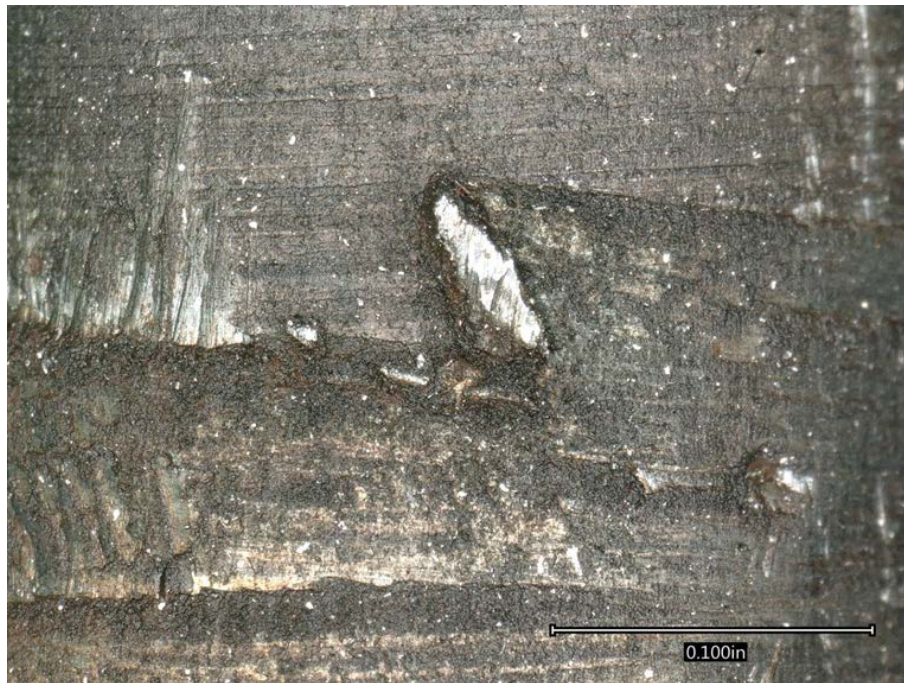
Figure 60. Additional close images of damage at the cooling passage surface. The lower image shows a close view of an angled feature with metal that has been piled up at the edge of the gouge.
