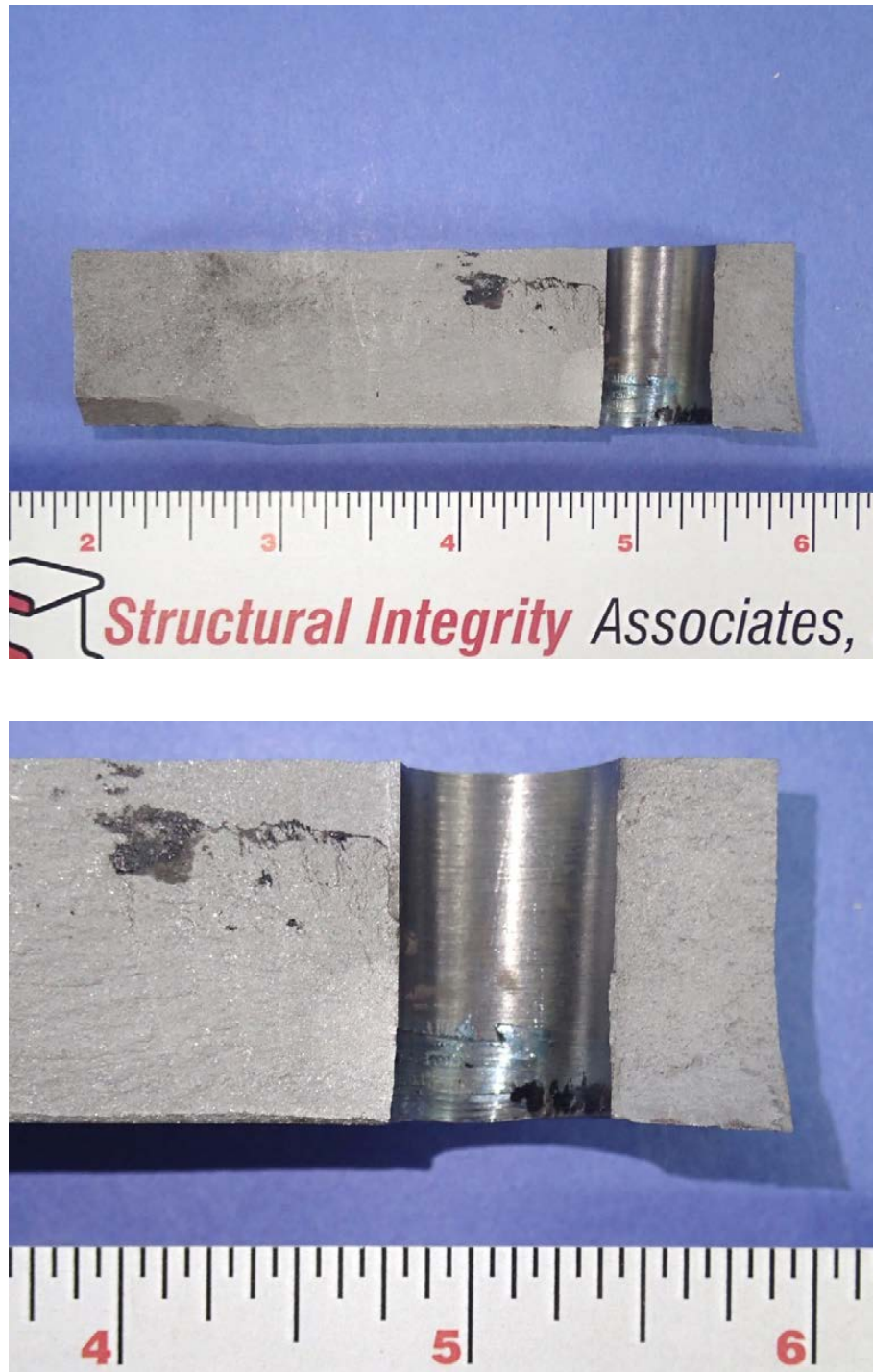
Figure 63. Views of the fracture surface section from the location below the dashed line in the upper image of Figure 58. The removed section is shown after cleaning in an ultrasonic bath with a mild Alconox solution.
