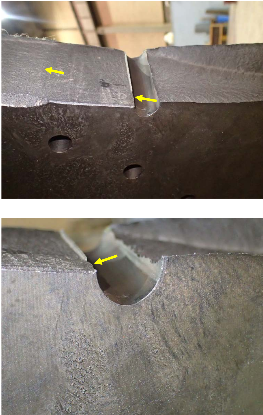
Figure 40. Alternate views of the central cooling passage hole at the upper fracture surface. The ID surface of the retaining ring is visible in each image. In the upper image, the right arrow indicates the crack origin area and the left arrow indicates the location of an apparent beach mark; other possible beach marks are visible between the left and right arrows. The arrow in the lower image also indicates the location of the apparent crack origin.
