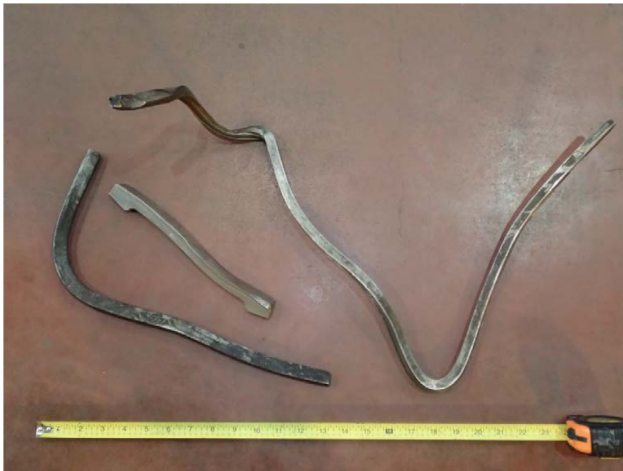
Figure 45. Views of the parts and fragments of material that appeared to be part of the ring retention snap ring and keys. The parts were deformed to various degrees and one of the ends of the snap ring was fractured.
