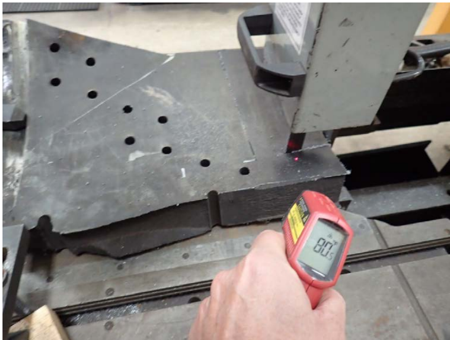
Figure 54. Views of the dry (bandsaw) cutting process during sectioning of the upper end of the ring. The metal temperature was monitored during cutting to ensure that no significant heating occurred.
