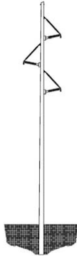
SINGLE CIRCUIT BRACED POST
