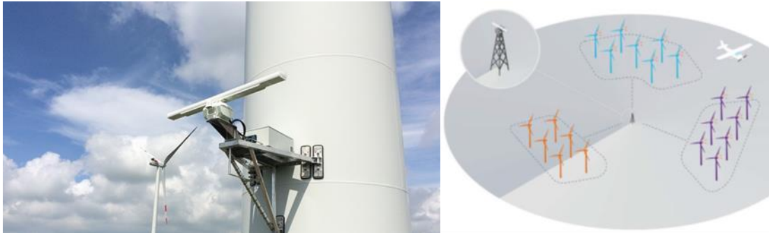
Figure 7. Aircraft Detection Lighting System 177
