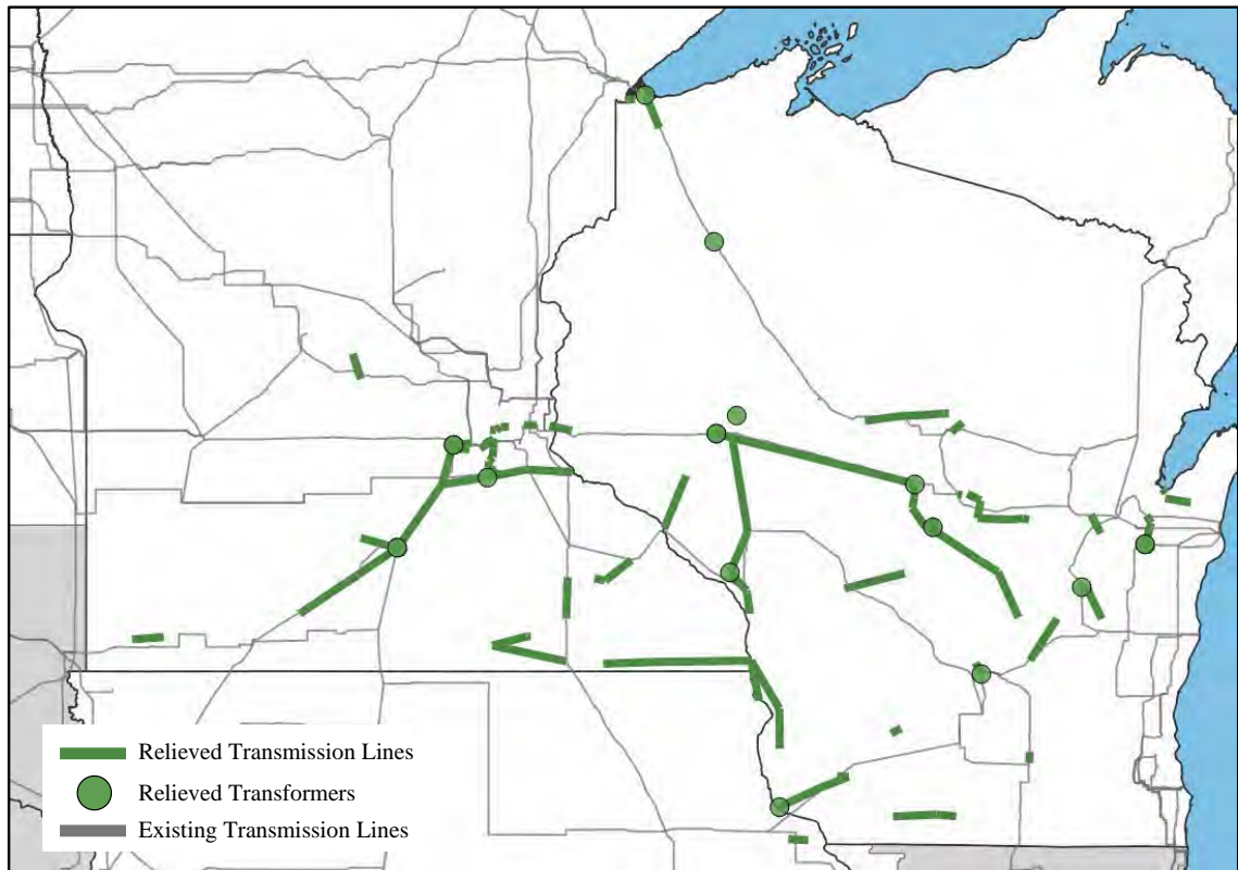
Figure 6-8: Map of facilities relieved in Future 1 power flow cases, for either N-1 or N-1-1 overloads. Transformers in green circles, and lines in green lines.
