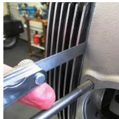
Figure 2 - Example Feeler Gauge Use
