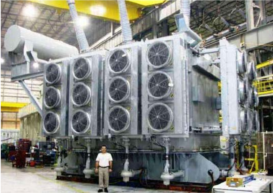
New Main Power Transformer (790,000 lbs)
