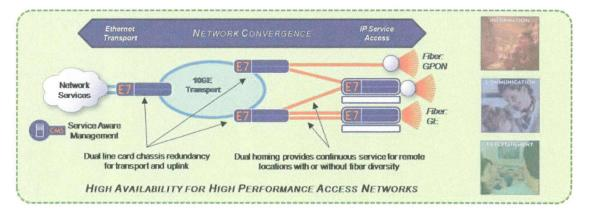
**FULL SPECTRUM OF SERVICES:** The E7 delivers a full spectrum of access services over GPON and Point-to-Point Ethernet using the family of Calix 700 ONTs, including Single Family Unit (SFU), Small Business Unit (SBU), Multi-Dwelling Unit (MDU), and rack-mount models.
