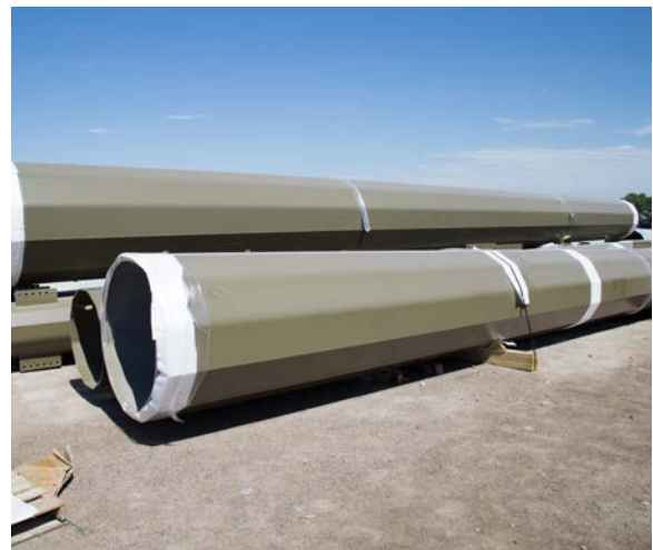
Figure 25 - Monopole ready for transport
