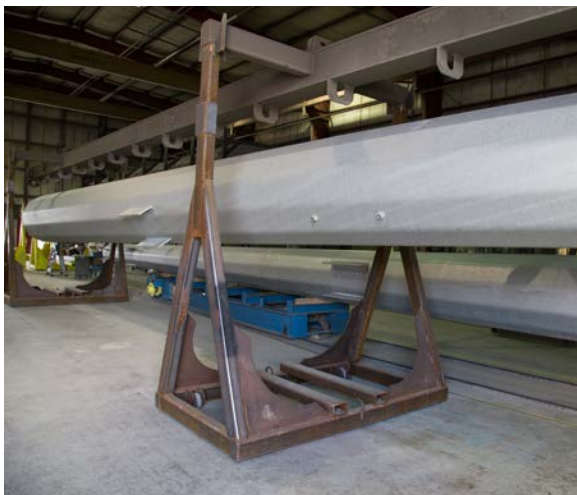
Figure 24 - Monopole ready for powder coat
