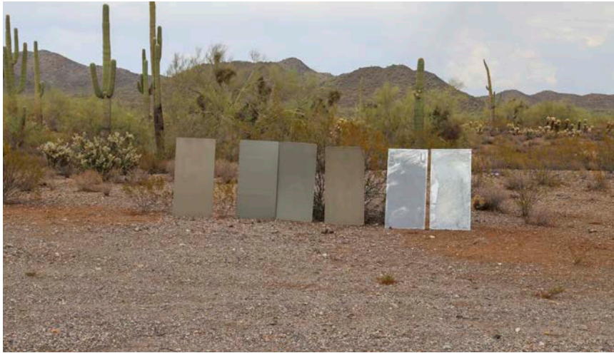
Figure 20 - Sample galvanized steel and powder coated panels
