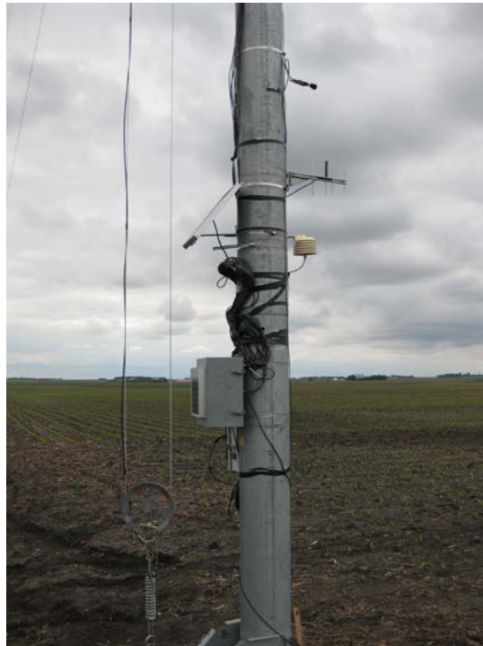
Photo 4. Tower 3 3m microphone, monitoring assembly, and landscape setting.
