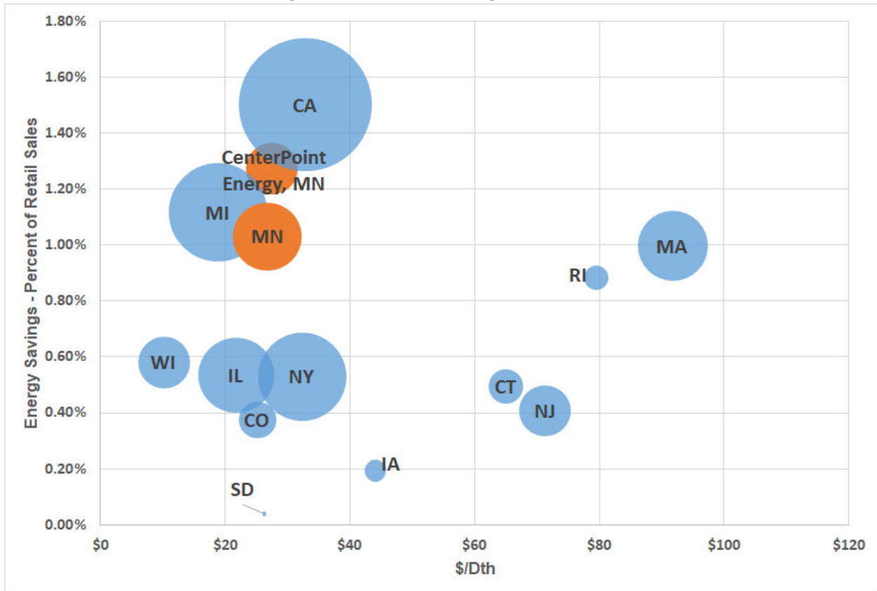
Figure 3: 2019-2021 Average Energy Efficiency Performance of Natural Gas Utilities, Average Annual Dth Savings (bubble size) 12
