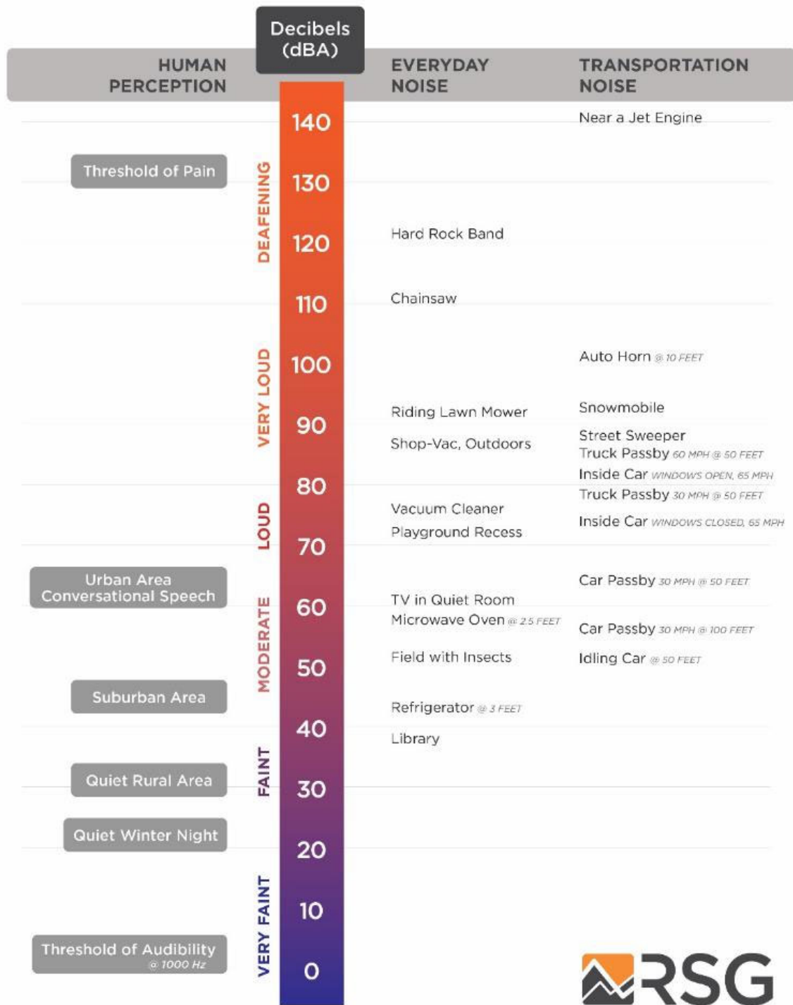
FIGURE 4: A SCALE OF SOUND PRESSURE LEVELS FOR TYPICAL SOUND SOURCES
