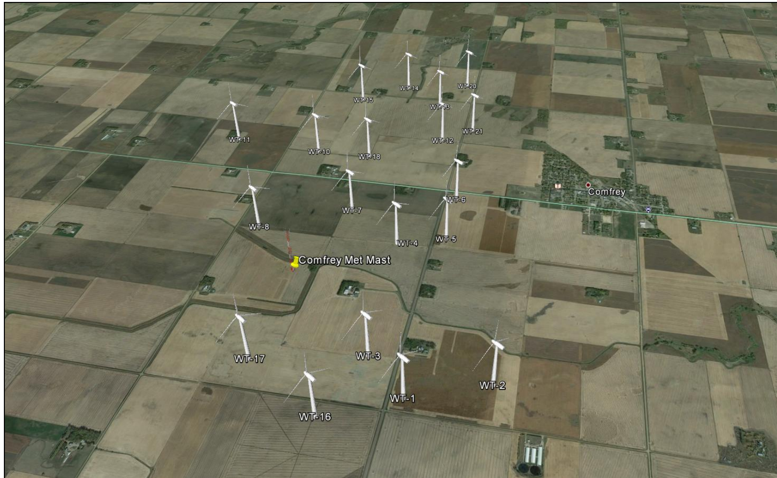
Figure 4. Comfrey wind farm, 19 General Electric wind turbines layout and met mast location, source Google Earth.
