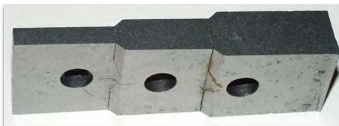
Figure 3: Example of stress corrosion cracking at the step down regions of a wheel finger.
