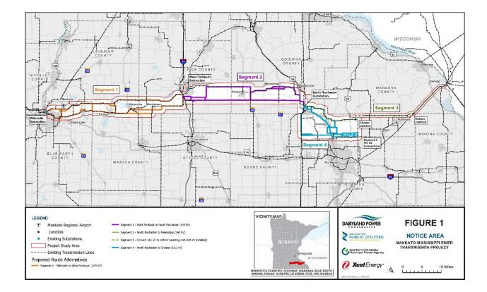
The proposed relocated 161kv line is currently double-circuited alongside a 354kv line in Segment 3.
