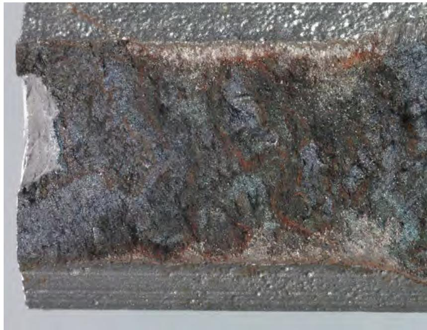
Fig. 401 Close-up photograph of crack surface from subsegment A3a shown in Fig. 398.
