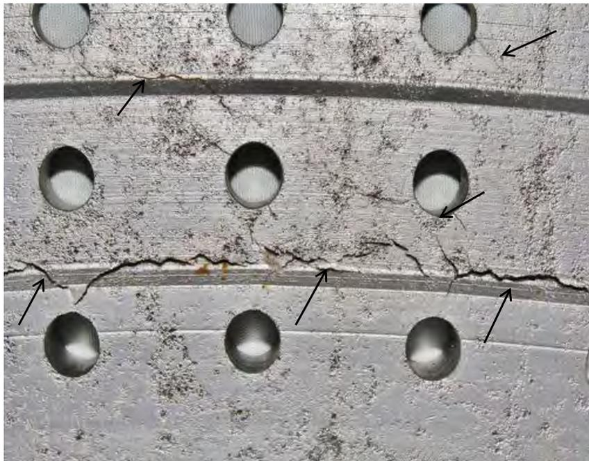
Fig. 393. Close-up photograph of generator end L-1 finger pinned blade attachment from LP turbine "B" showing location of cracks (arrows). Pc "A3", side 2.
