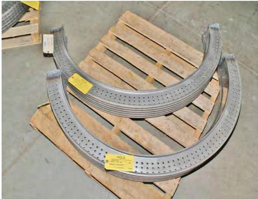
Fig. 381. Photograph of turbine end L-1 disk rim from LP turbine "A". The disk rim had been sectioned and removed at GE Repair Facility in Chicago, Illinois.
