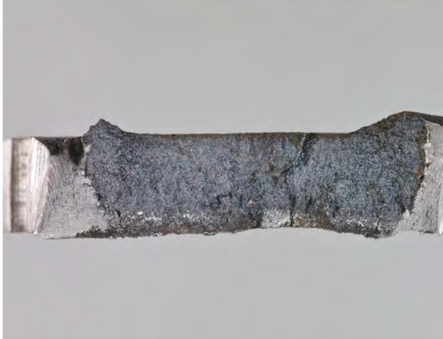
Fig. 402. Close-up photograph of crack surface from subsegment A3b shown in Fig. 399.
