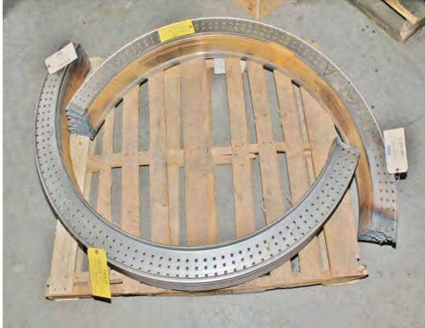
Fig. 380. Photograph of generator end L-1 disk rim from LP turbine "A". The disk rim had been sectioned and removed at GE Repair Facility in Chicago, Illinois.
