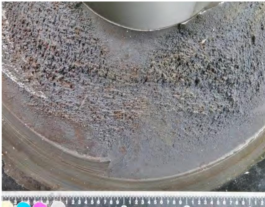
Fig. 348. Close-up of fracture surface of exciter shaft fracture adjacent to the No. 12 bearing.
