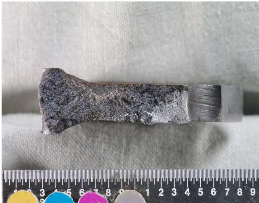
Fig. 415. Close-up photograph of crack surface from subsegment A4b shown in Fig. 411.
