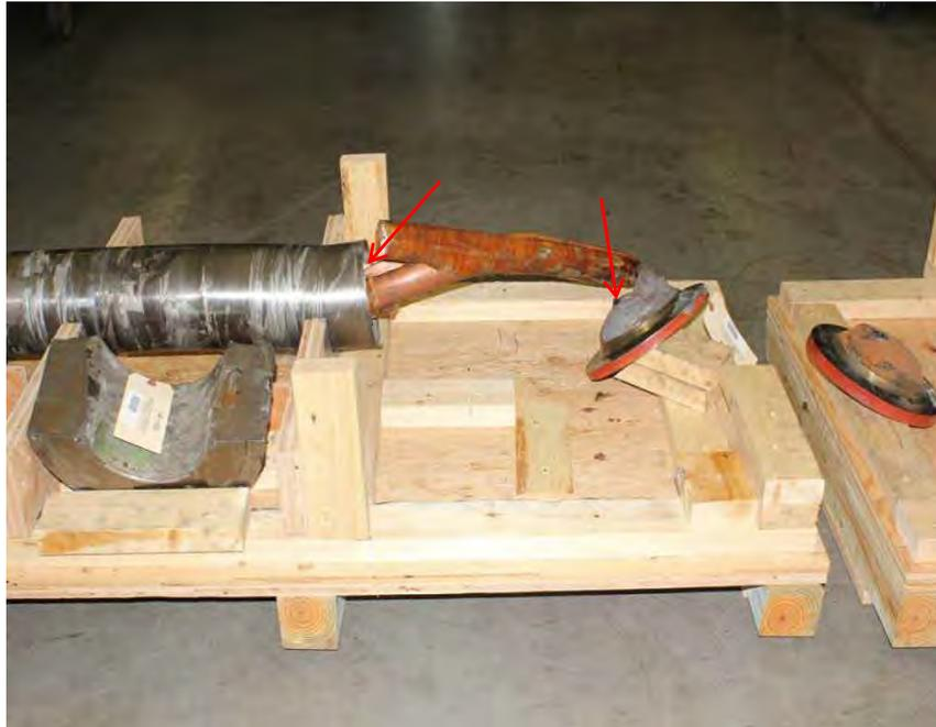
Fig. 339. Photograph of exciter shaft that fractured transversely (arrows) adjacent to the No. 12 bearing.
