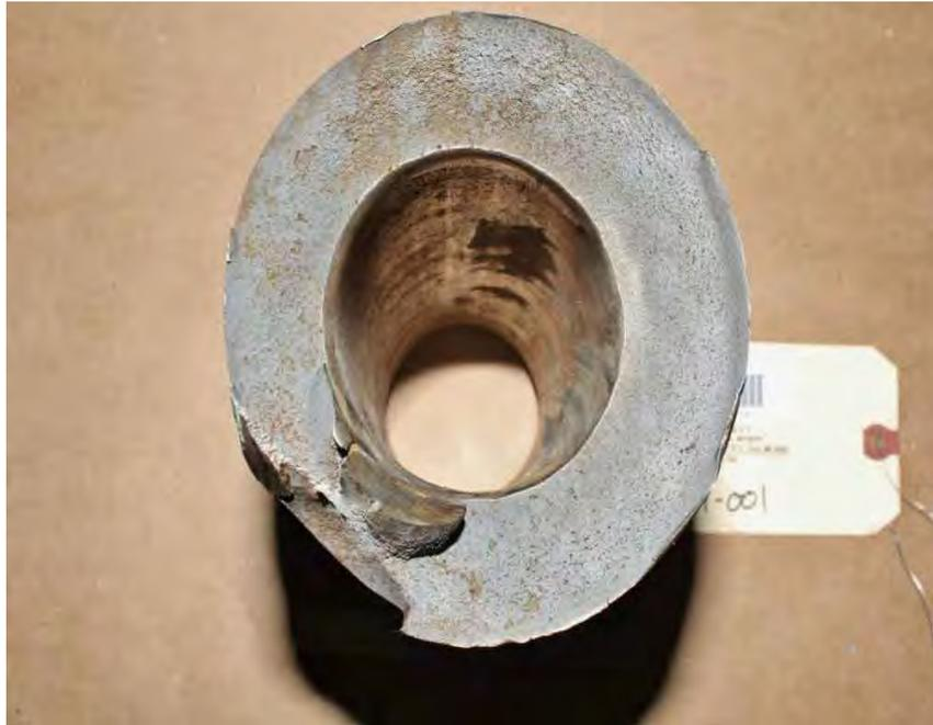
Fig. 349. Close-up of fracture surface of exciter shaft fracture adjacent to the Alterex collector ring.
