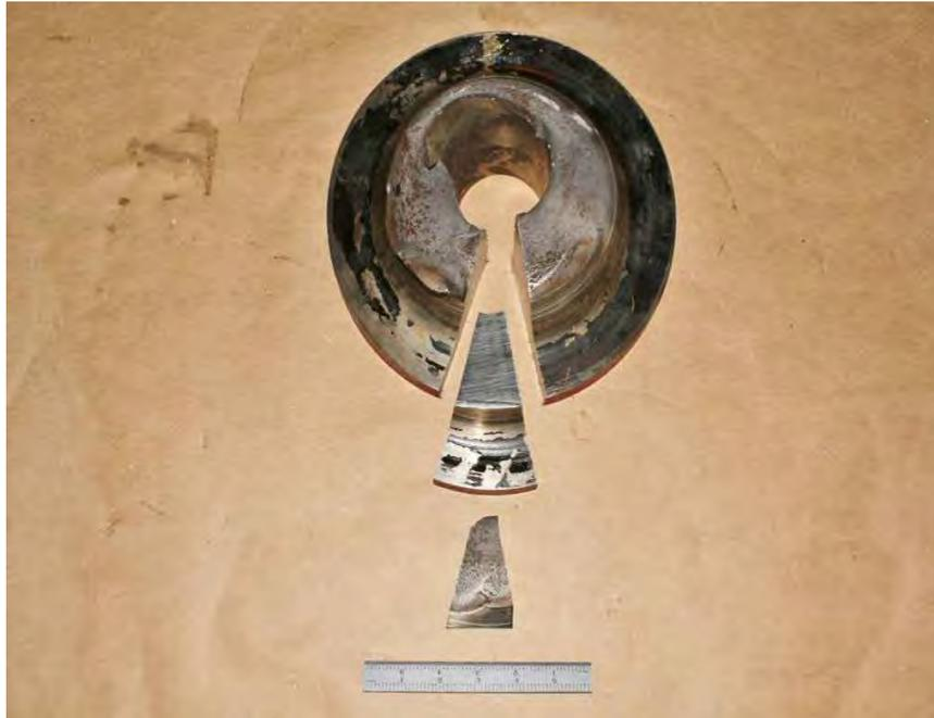
Fig. 359. Photograph of exciter shaft fracture adjacent to the No. 12 bearing showing subsegment removed for scanning electron microscope examination.
