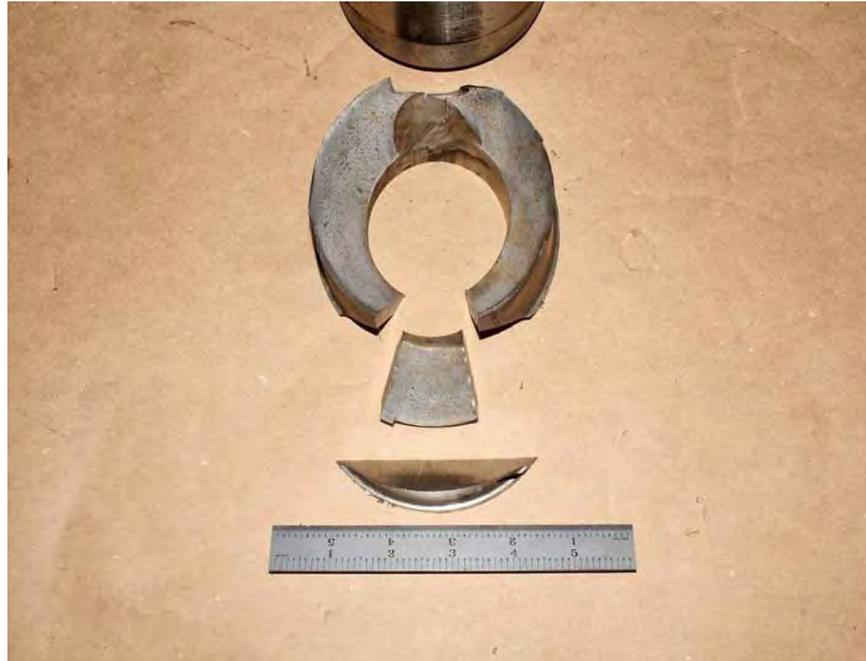
Fig. 368. Photograph of exciter shaft fracture adjacent to the Alterex collector ring showing subsegment removed for scanning electron microscope examination.
