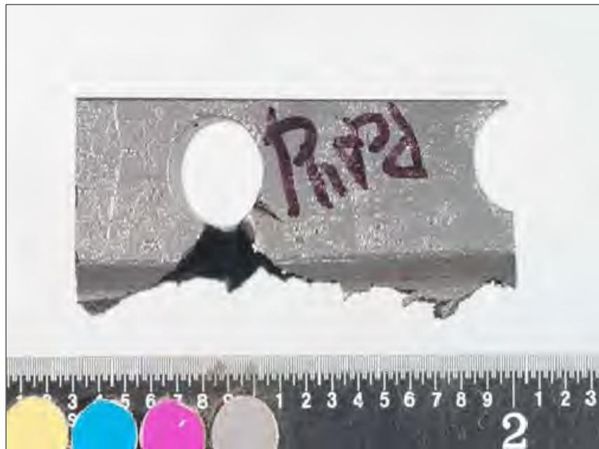
Fig. 413. Close-up photograph of subsegment A4d from LP turbine "B" containing a circumferential crack shown in Fig 409.
