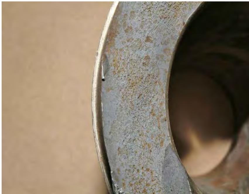
Fig. 350. Close-up of fracture surface of exciter shaft fracture adjacent to the Alterex collector ring.
