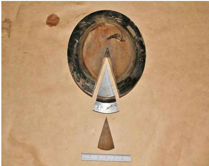
Fig 352. Photograph of exciter shaft fracture adjacent to the No. 11 bearing showing subsegment removed for scanning electron microscope examination.
