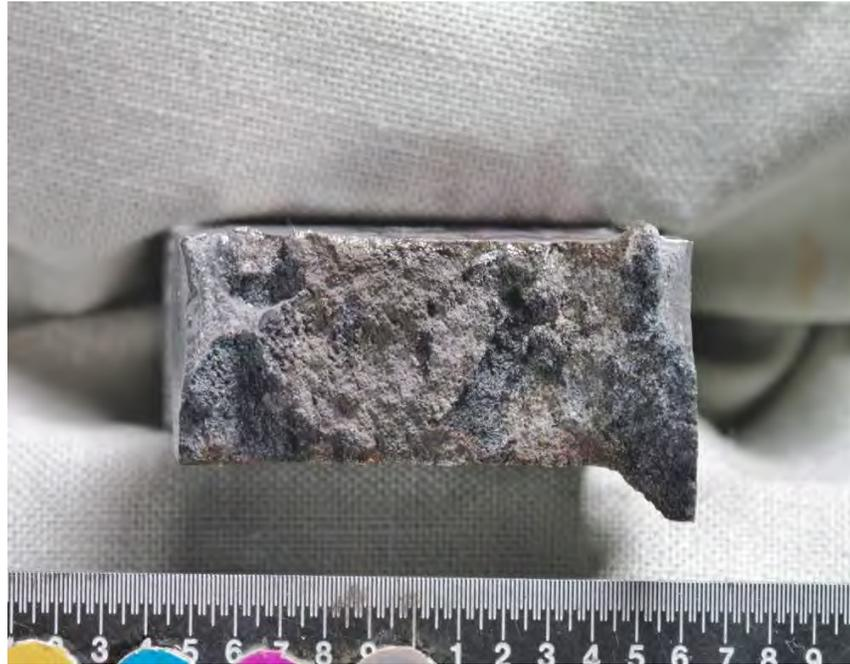
Fig. 416. Close-up photograph of crack surface from subsegment A4c shown in Fig. 412.
