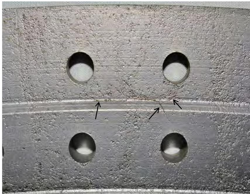
Fig. 389. Close-up photograph of generator end L-1 finger pinned blade attachment from LP turbine "A" showing location of cracks (arrows).Pc "A5", side 1.
