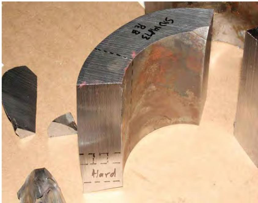
Fig. 332. Close-up photograph of generator shaft forward end fracture half showing subsegment removed for hardness testing.
