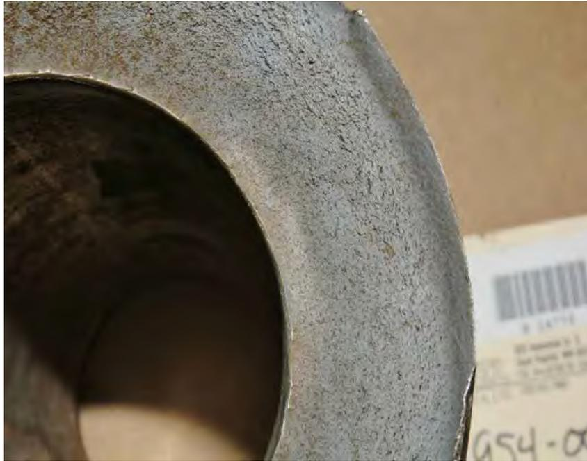
Fig. 351. Close-up of fracture surface of exciter shaft fracture adjacent to the Alterex collector ring.
