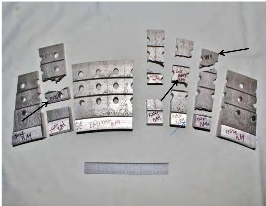
Fig. 409. Generator end finger pinned blade attachment, Pc A4, from LP turbine "B" showing sectioning of cracks (arrows) for further examination.
