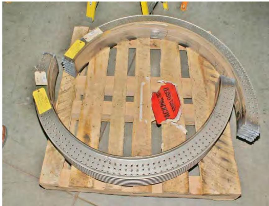
Fig. 379. Photograph of turbine end L-1 disk rim from LP turbine "A". The disk rim had been sectioned and removed at GE Repair Facility in Chicago, Illinois.
