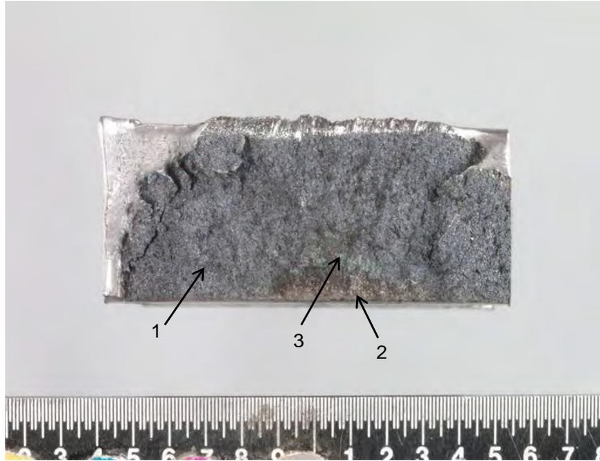
Fig. 406. Close-up photograph of crack surface from subsegment A4a shown in Fig. 404.
