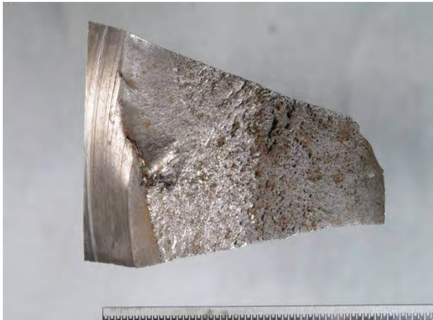
Fig. 360. Photograph of exciter shaft fracture adjacent to the No. 12 bearing showing areas examined by scanning electron microscope.
