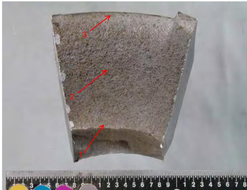
Fig. 369. Photograph of exciter shaft fracture adjacent to the Alterex collector ring showing areas examined by scanning electron microscope.
