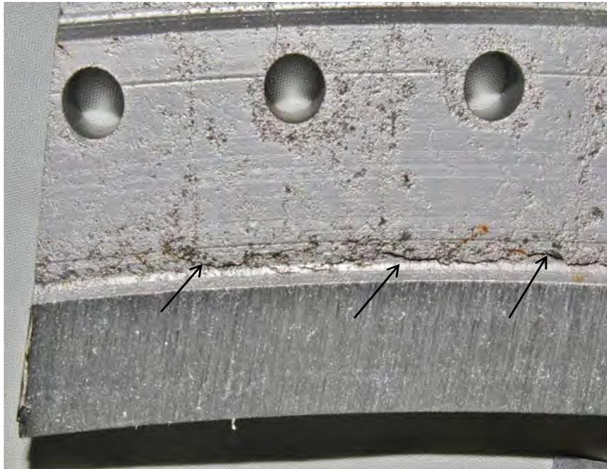
Fig 395. Close-up photograph of generator end L-1 finger pinned blade attachment from LP turbine "B" showing location of cracks (arrows). Pc "A4", side 2.
