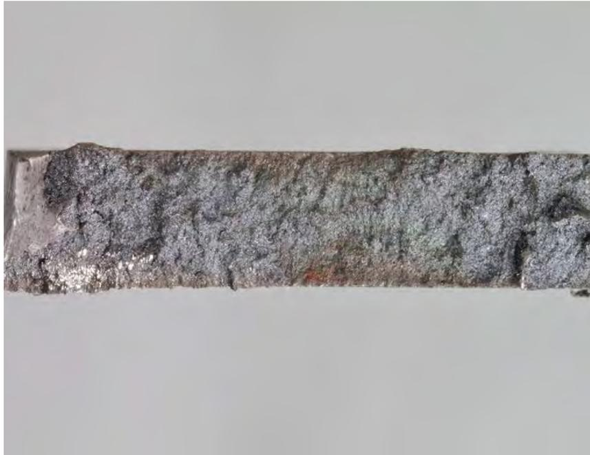
Fig. 408. Close-up photograph of crack surface from subsegment A4b shown in Fig. 405.
