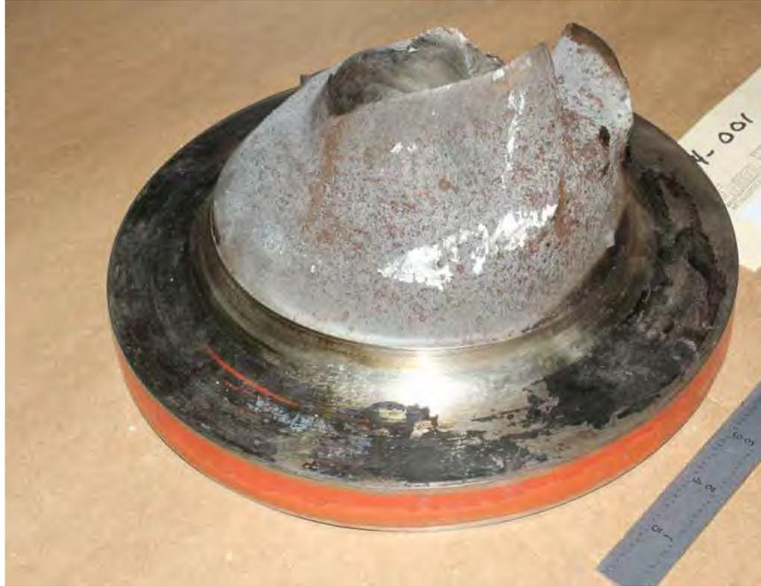
Fig. 345. Close-up of fracture surface of exciter shaft fracture adjacent to the No. 12 bearing.
