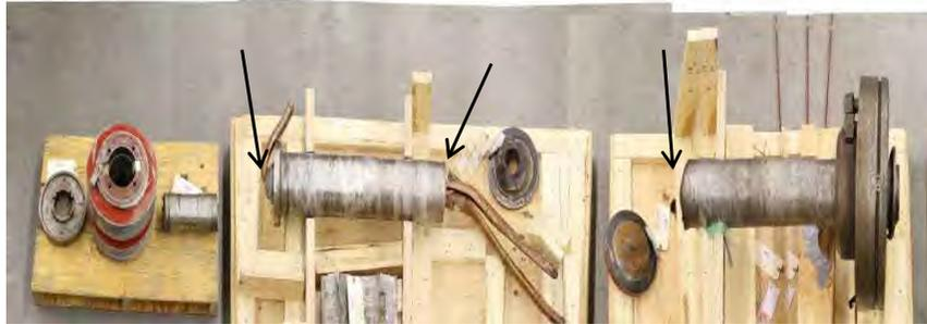
Fig. 337. Sherco Unit 3 exciter shaft that fractured transversely at three locations (arrows) during event of Nov. 19, 2011.
