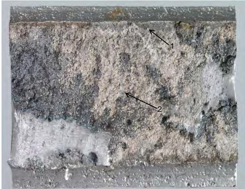
Fig. 414. Close-up photograph of crack surface from subsegment A4a shown in Fig. 410.
