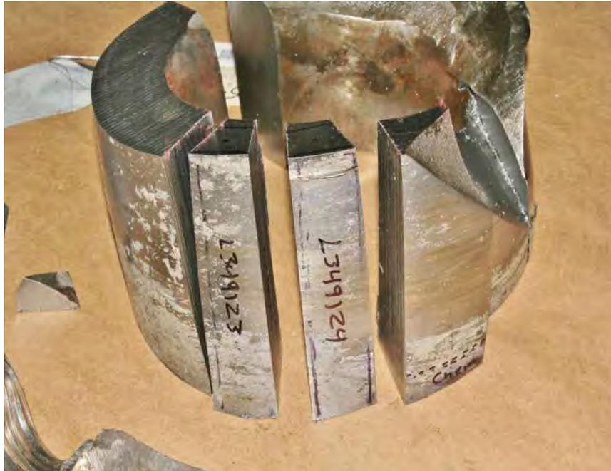
Fig. 331. Close-up photograph of generator shaft forward end fracture half showing two coupons removed for tensile specimens.
