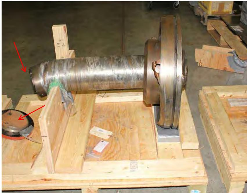
Fig. 338. Photograph of exciter shaft that fractured transversely (arrows) adjacent to the No. 11 bearing.
