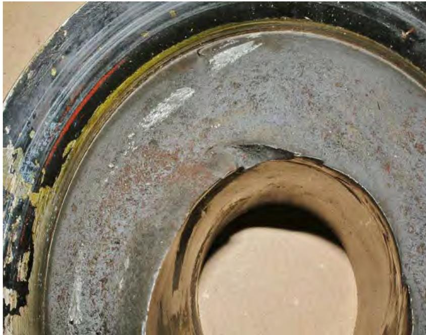
Fig. 346. Close-up of fracture surface of exciter shaft fracture adjacent to the No. 12 bearing.
