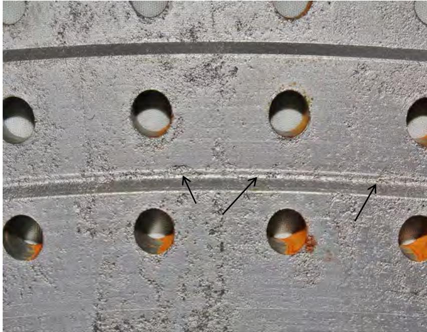
Fig. 382. Close-up photograph of turbine end L-1 finger pinned blade attachment from LP turbine "A" showing location of cracks (arrows). Pc "A2", side 2.
