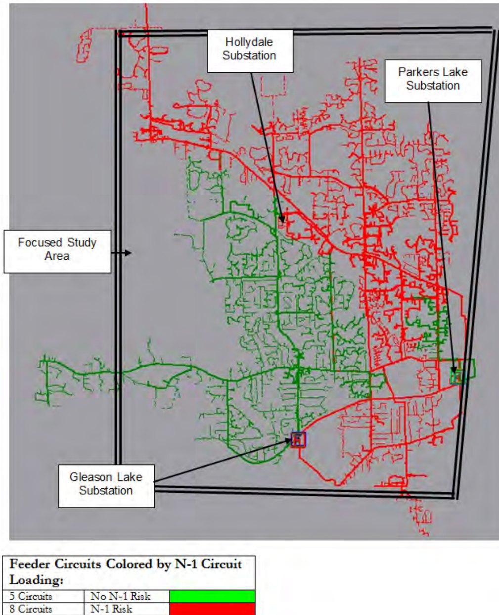
Figure 5.10: Focused Study Area 2016 N-1 Feeder Circuit Loading – Single Contingency
