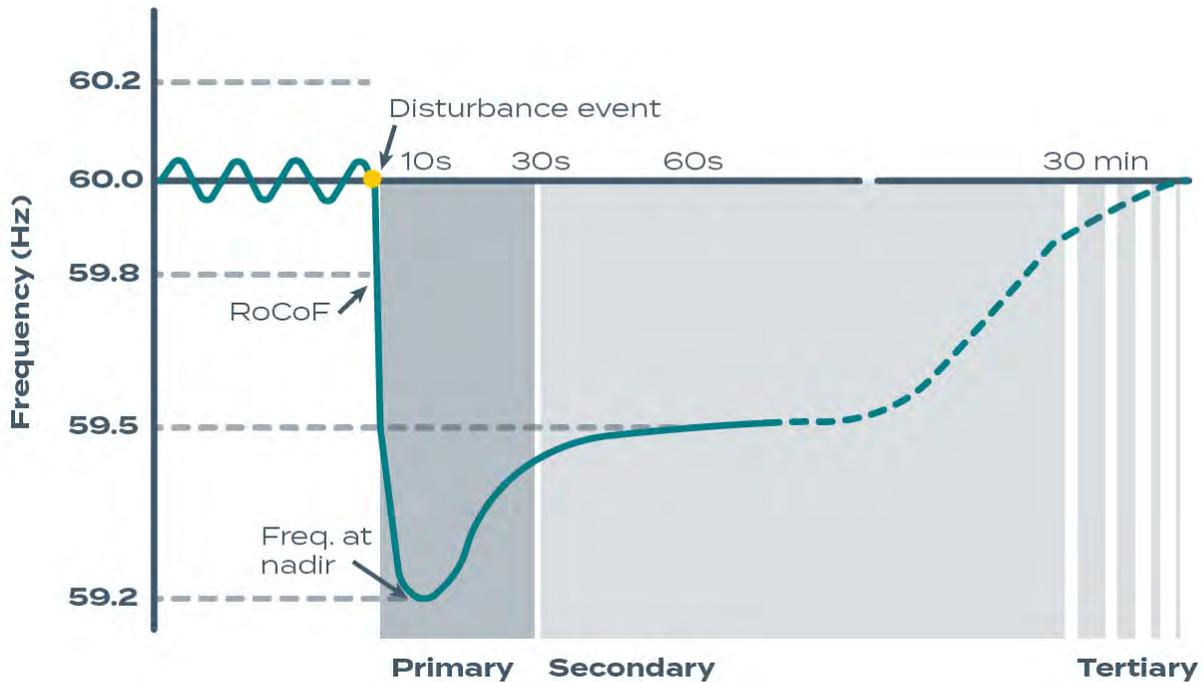
This figure shows the grid operating at 60 Hz until an incident (yellow dot) creates a disturbance. In this example, the RoCoF is how quickly the frequency dropped and the nadir is the greatest drop in frequency experienced before the primary response mechanisms were able to stop the frequency drop.
