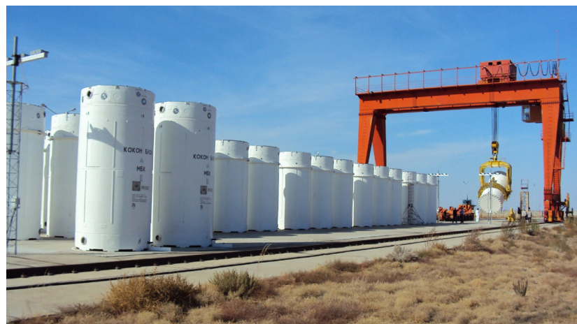
At right, a dry storage cask recently loaded with spent fuel is lifted from a horizontal transporter to be placed on a specially designed storage pad. (Courtesy: Sandia National Laboratories)
