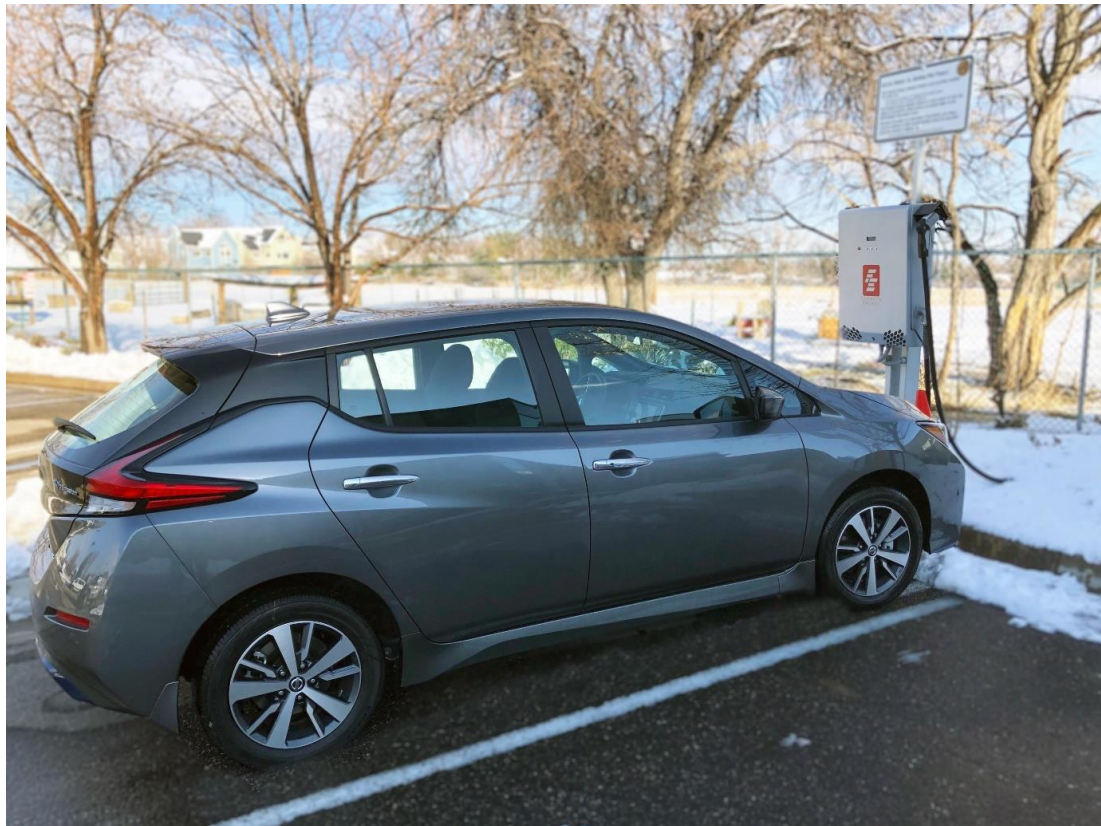
Figure 6: Nissan Leaf with Fermata Bidirectional Charger at Boulder Recreation Center
