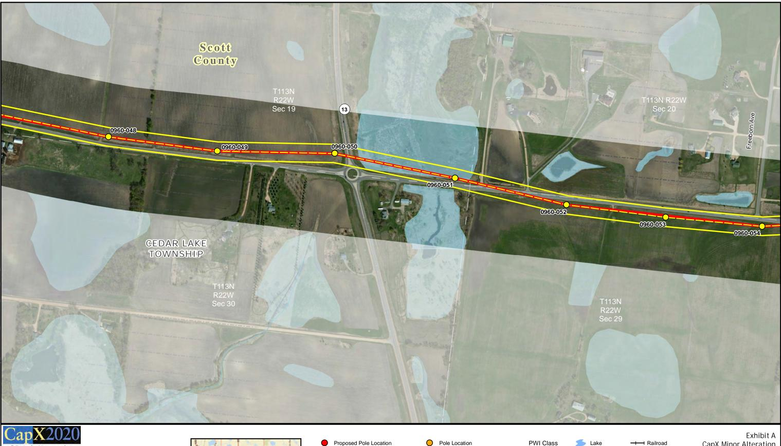
Proposed Substation and Cedar Lake transmission structure locations are approximate. Final locations are subject to revisions based on engineering design
