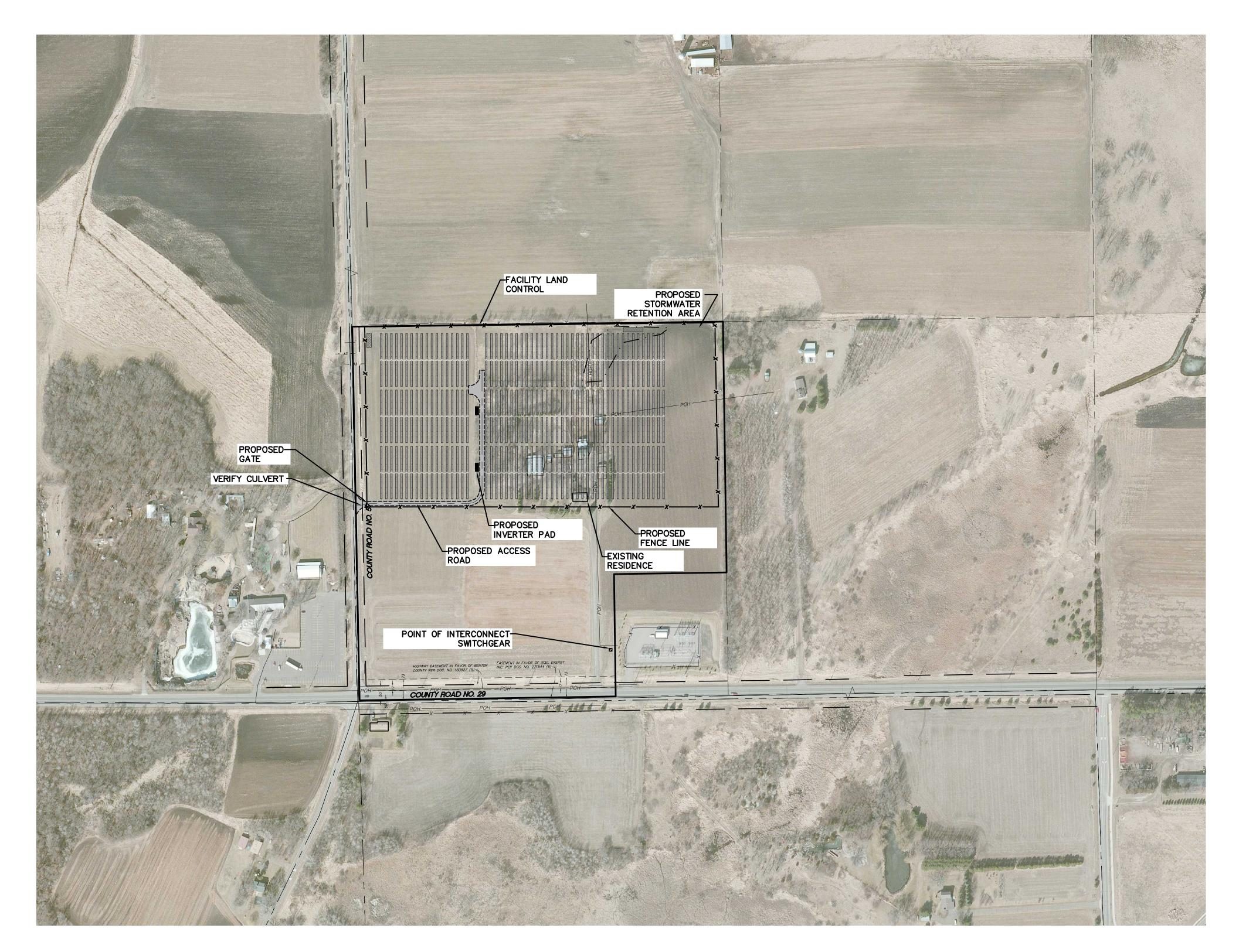
PROPOSED LEASED AREA PROPOSED SOLAR ARRAY PROPOSED ACCESS ROAD PROPOSED INVERTER PAD ——x——x—— PROPOSED FENCE LINE PROPOSED STORMWATER RETENTION ——x———x—— EXISTING FENCE LINE POH EXISTING OVERHEAD POWER LINE ——— EXISTING RIGHT OF WAY LINE ---- Existing easement line — · — · — EXISTING DELINEATED WETLAND AREA PROJECT LOCATION: LAT: 45.6201 LON: -94.1519
