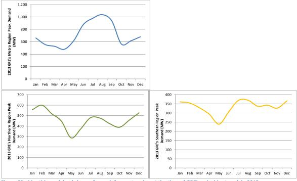
Figure 63. Monthly peak load shapes for each forecast region at the time of GRE's coincident peak in 2013.
